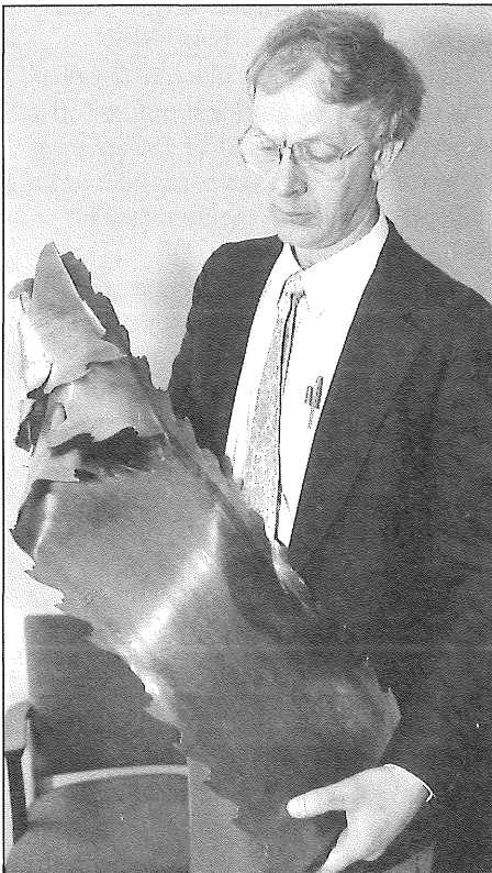
Howard Hedstrom, an owner of Hedstrom Lumber, Inc., showed members of the Criminal Justice Division March 20 what happens to a high-speed saw blade when it hits a spike hidden in a tree.
