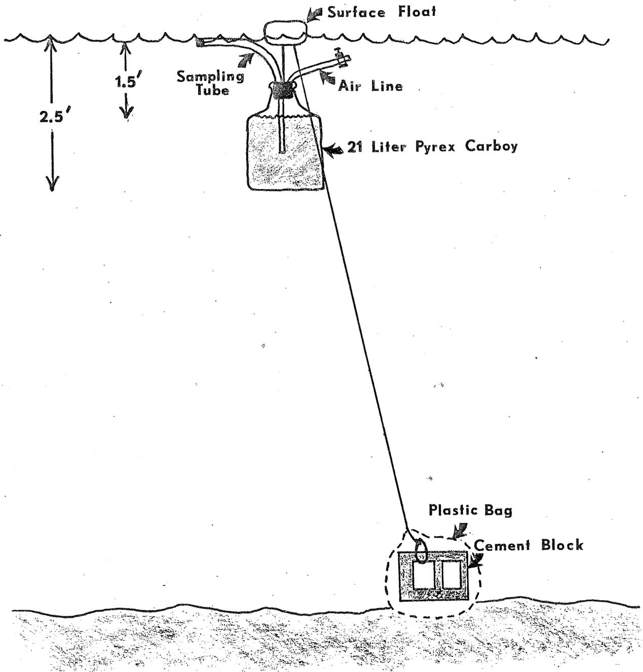
Figure 3. Detail of Enclosure Bottle.
