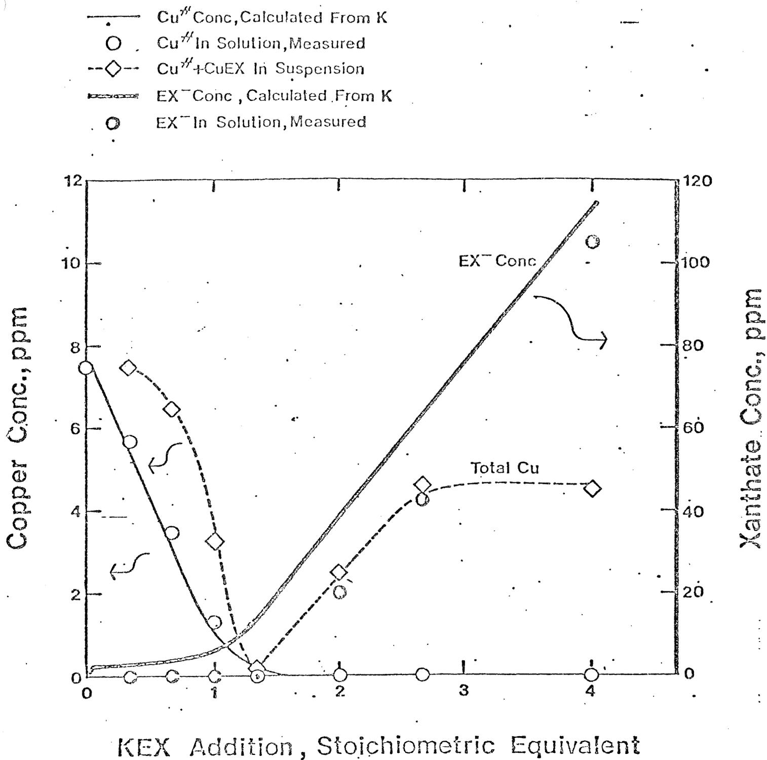
FIGURE 16. RESIDUAL CONCENTRATIONS OF COPPER AND XANTHATE IN ION FLOTATION AS A FUNCTION OF POTASSIUM ETHYL XANTHATE ADDITION<sup>7</sup>
