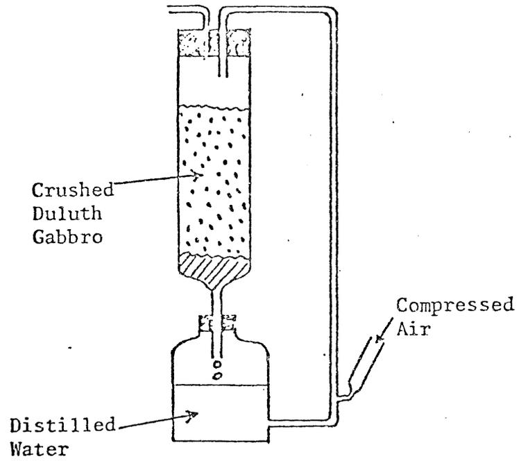
FIGURE 13. SCHEMATIC DIAGRAM OF AIRLIFT PERCOLATOR
