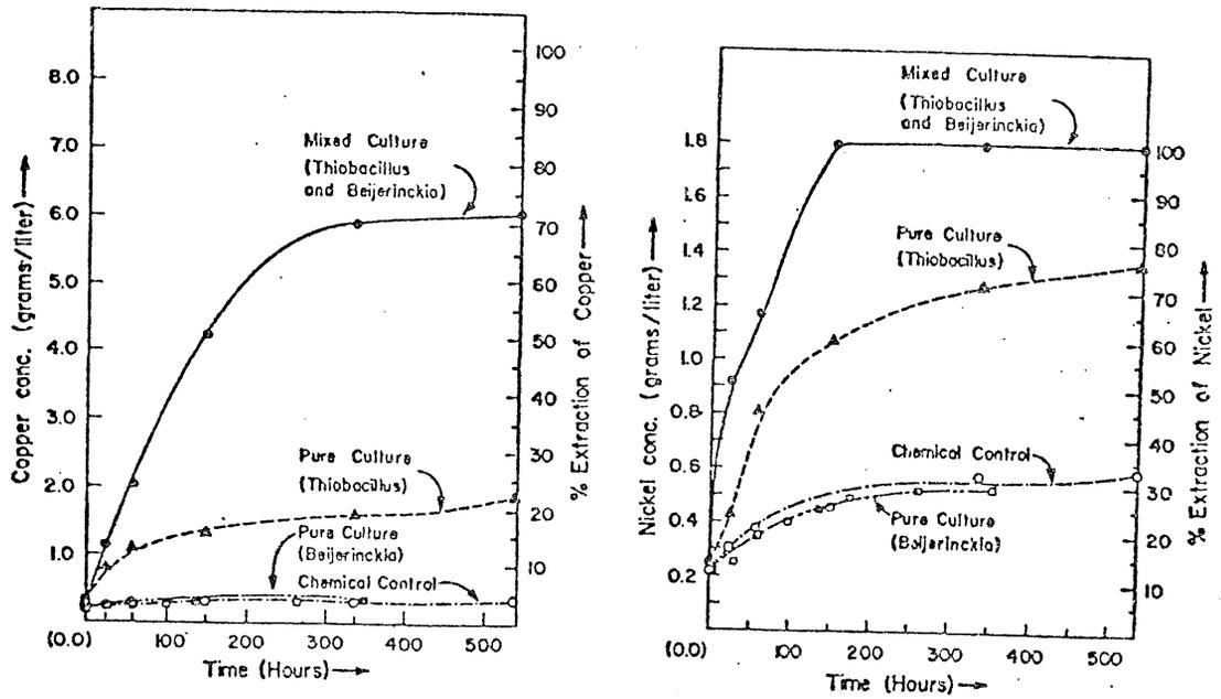
Figure 5. Batch leaching of copper and nickel with pure and mixed cultures of *T. ferrooxidans* and *B. lacticogenes* at 25°C. (From Trivedi and Tsuchiya, 1975).
