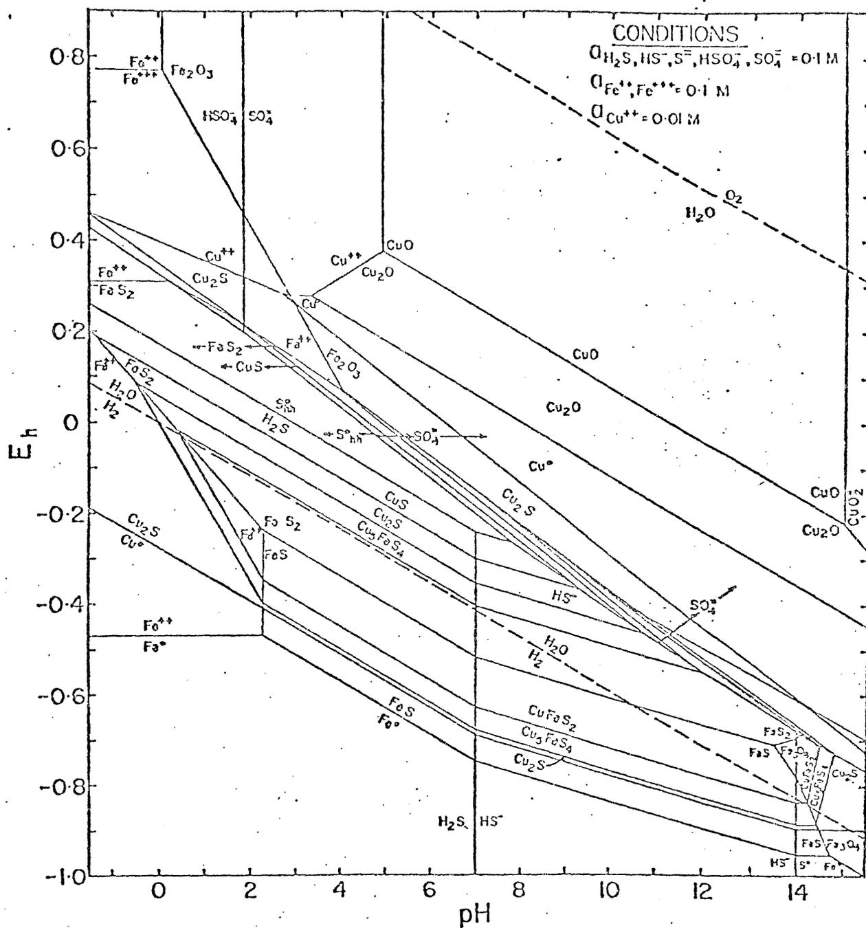
Figure 4. Eh-pH diagram for the Cu-Fe-S-H<sub>2</sub>O system. (Peters, 1970).
