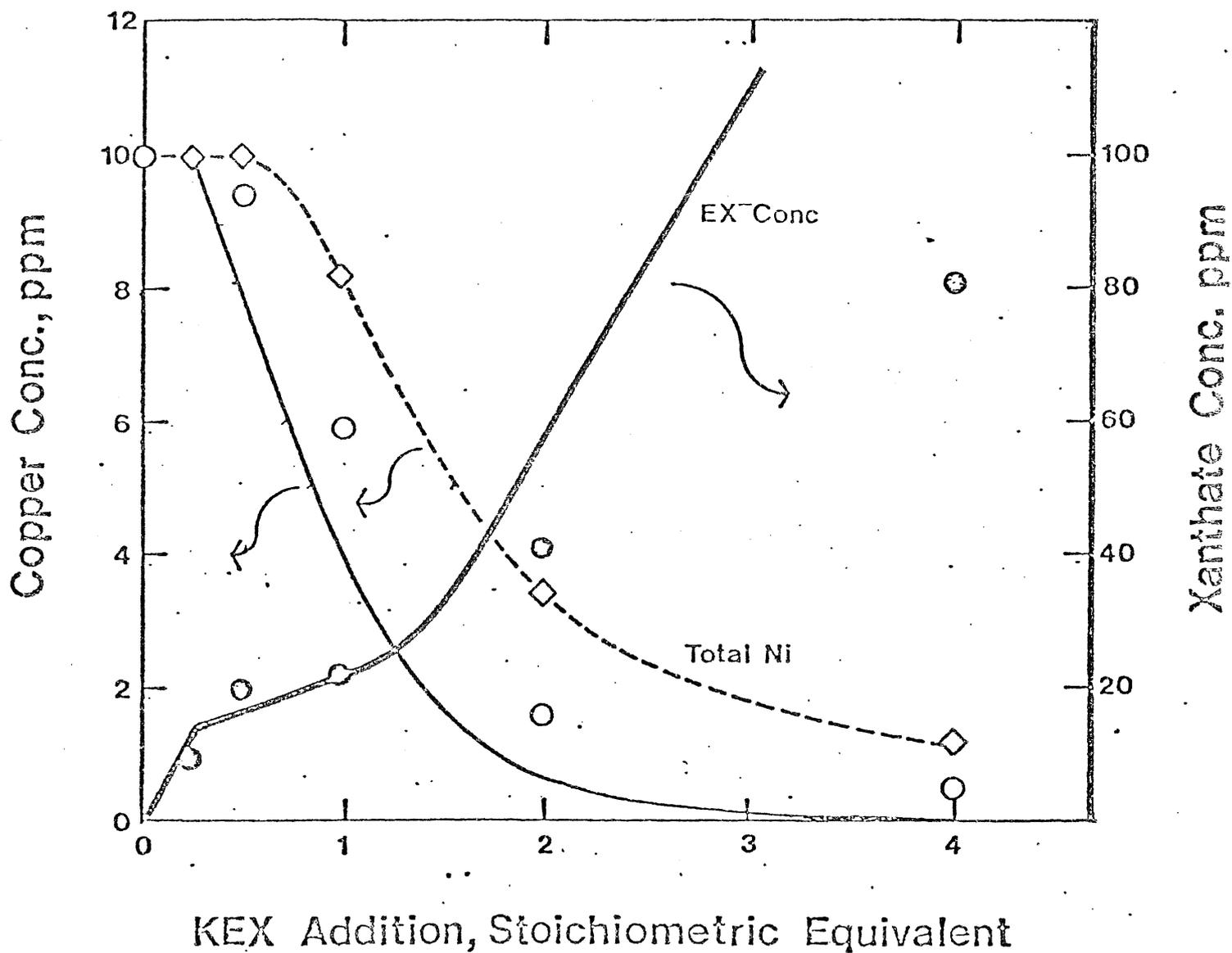
FIGURE 17. RESIDUAL CONCENTRATIONS OF NICKEL AND XANTHATE IN ION FLOTATION AS A FUNCTION OF POTASSIUM ETHYL XANTHATE ADDITION<sup>7</sup>
