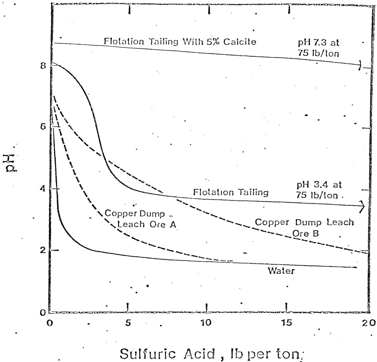
FIGURE 12. PULP pH OF A FLOTATION TAILING OF DULUTH GABBRO AND OF COPPER DUMP LEACH ORES AS A FUNCTION OF SULFURIC ACID ADDITION<sup>7</sup>
