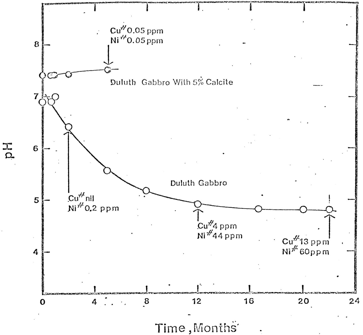
FIGURE 14. CHANGE IN pH WITH TIME OF WATER CIRCULATING THROUGH CRUSHED DULUTH GABBRO<sup>7</sup>
