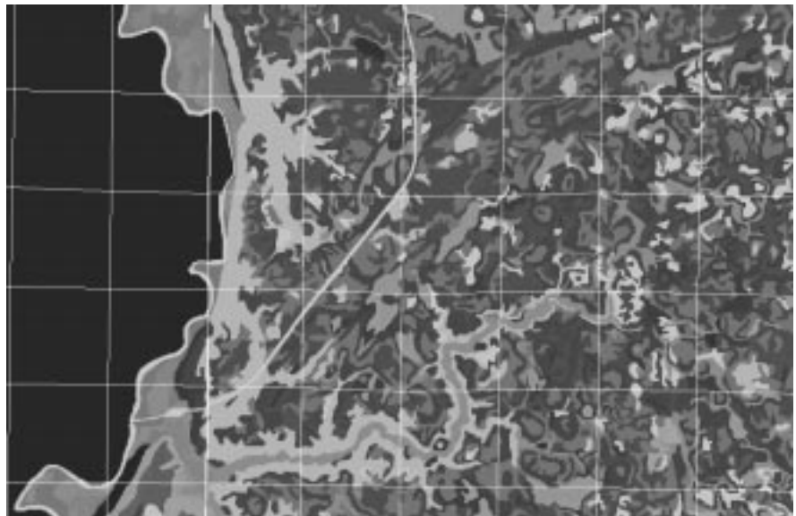
This gray-tone map displays soil types using EPPL7 raster-format software. It shows the northwestern corner of Le Sueur County. The straight white lines represent section lines from the Public Land Survey. Source: Land Management Information Center
