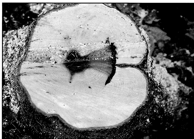
Cross section of a crack that has stain but no decay.
