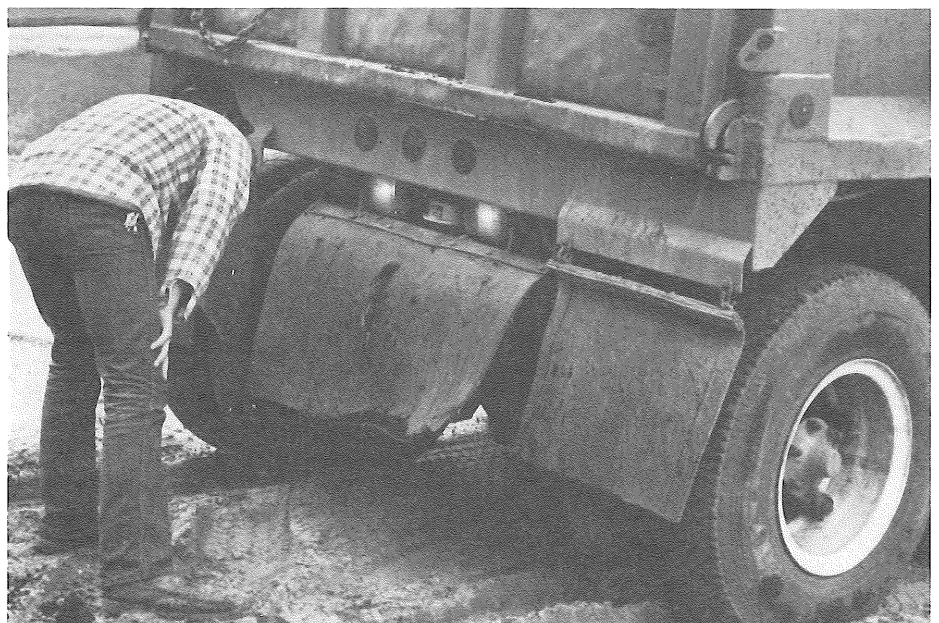
Chap. 548 requires that bottom-load dump trucks be equipped with flaps attached to the rear of the axles and that trucks carrying sand, gravel, dirt or similar material be properly loaded or securely covered.
