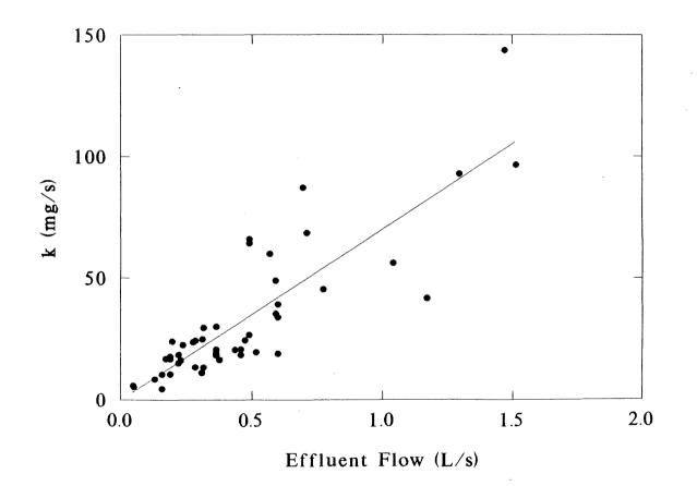
Figure 7. Alkalinity release rate (k) vs effluent flow.
