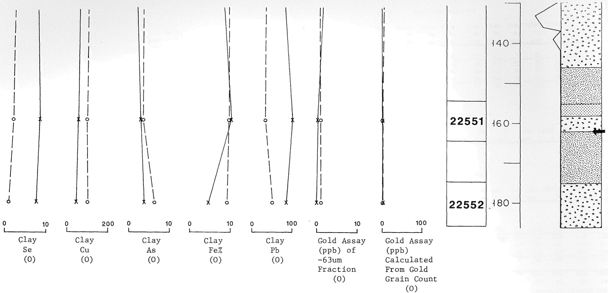
(146 - 155) VERY COARSE SAND & GRAVEL; UNOXIDIZED; sm cob at 153 ft.
