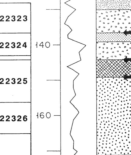
**R** (126 - 130) GRAVELLY SAND; OXIDIZED; loamy cgr to v cgr sand w/sev cobs to 128 ft, then v cgr pebbly sand; little or no carb; unox by 129.
