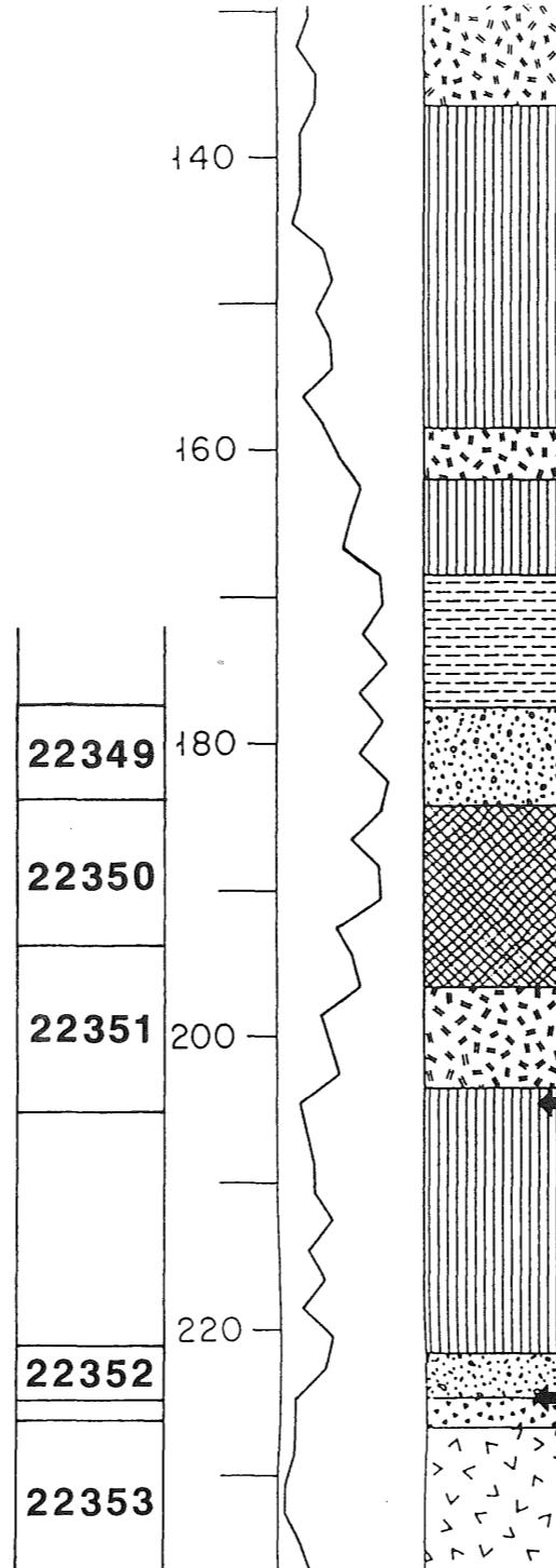
(136 - 158) CLAY & SILTY CLAY; UNOXIDIZED; laminated; calc; sm silt lens at 146 ft, more lenses & lam below, also sand lam; pebs at 153 1/2, 155; increasing sand grains in last few feet.
