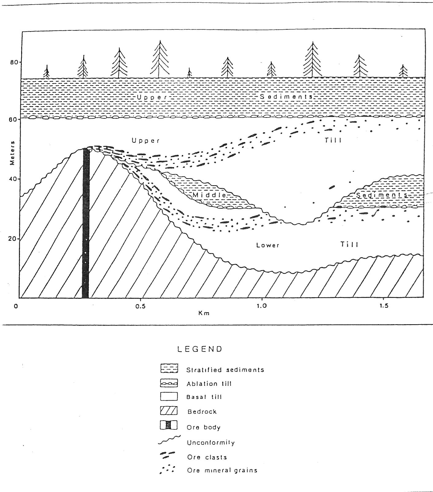
Figure 1. Dispersion pattern for two tills with gold source on a bedrock high (Developed by Overburden Drilling Management Ltd.).
