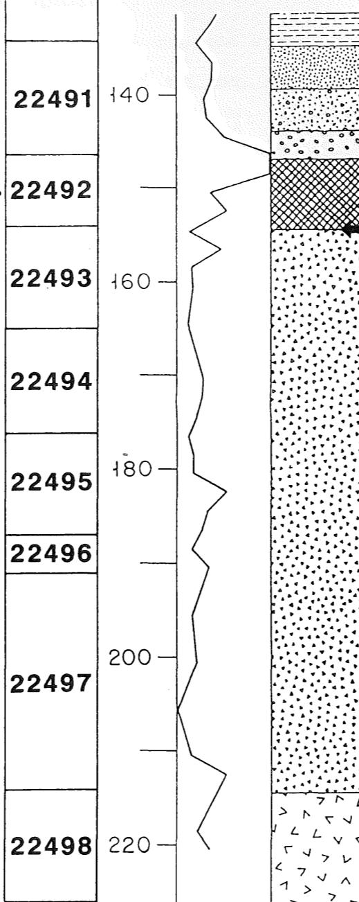
(131 - 134 1/2) SILT; UNOXIDIZED; calc; clayey silt lam; sand bed near baso.
