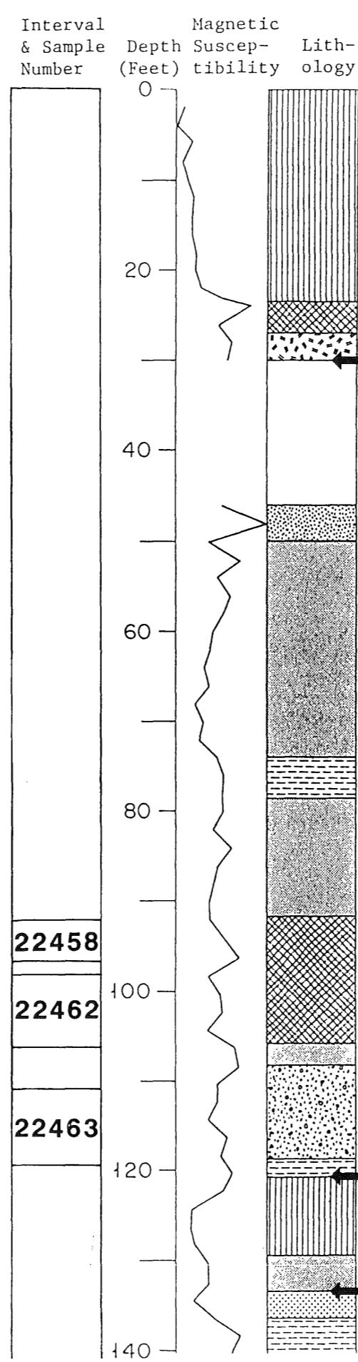
**K** (0 - 23 1/2) CLAY - SILTY CLAY; OXIDIZED; leached to 1 foot; massive; v few sand grains; carb gnl at 13 1/2, 19 ft.
