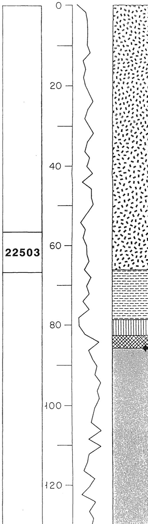
(66 - 78 1/2) SILT; UNOXIDIZED; calc; abrupt upper contact; sandy bed at 67 1/2 ft; clay lens at 73; laminated silt & clay from 73 1/2 - 75 1/2.
