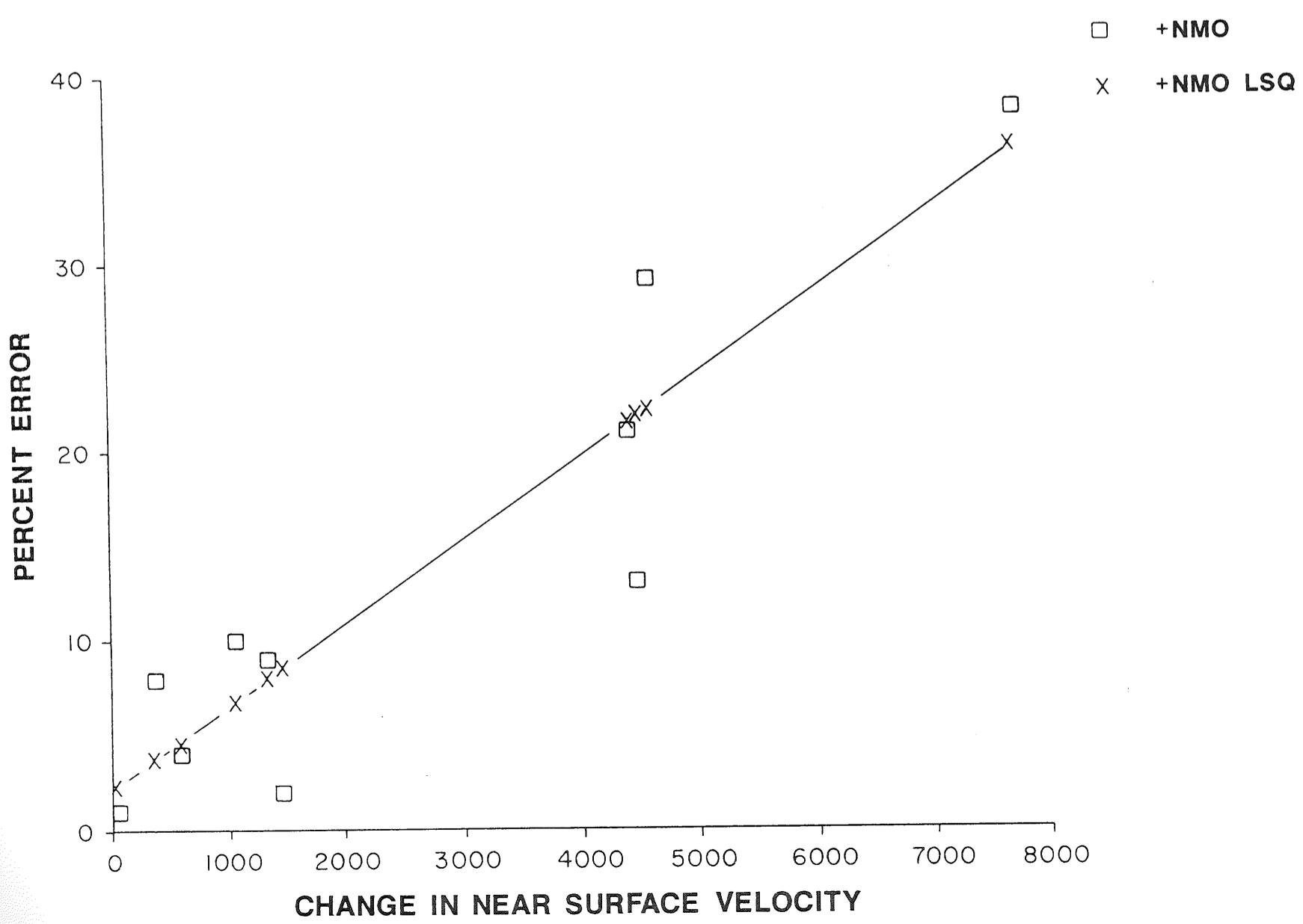
FIG. 8-3: NEAR SURFACE PERCENT ERROR/CHANGE IN VELOCITY
