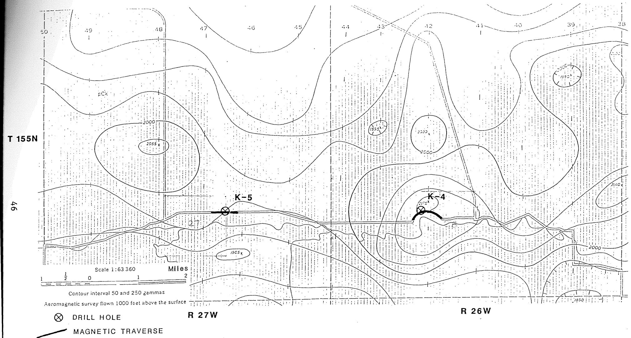
FIGURE 264-12. Aeromagnetic Map of a Portion of Koochiching County with Locations of DDH's K-4 and K-5, and Ground Magnetic Traverses (modified from Meuschke et al., 1957b).
