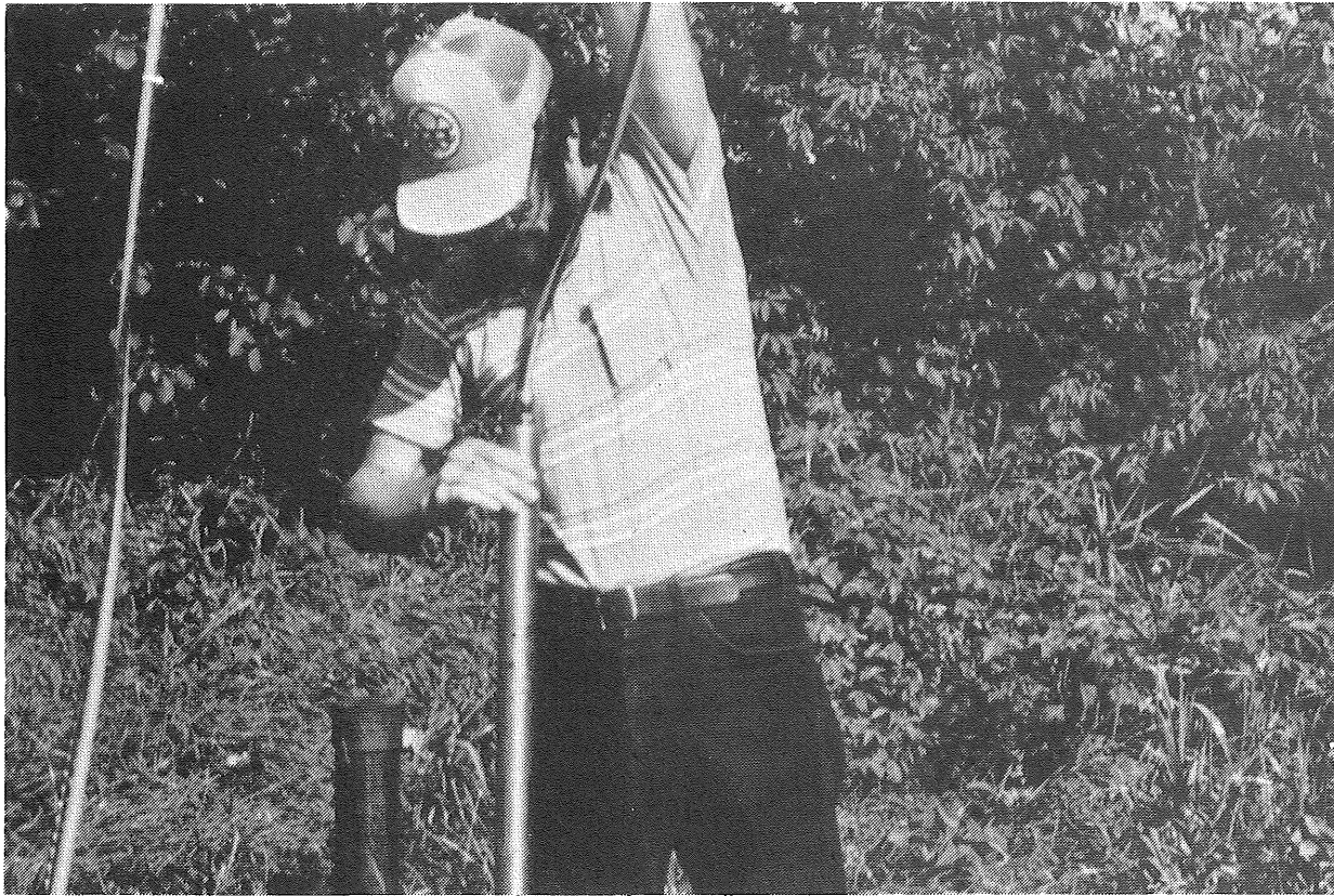
Collection of ground water samples from monitoring wells requires special equipment, in this case, a portable submersible pump which will fit inside narrow-diameter well casings.
