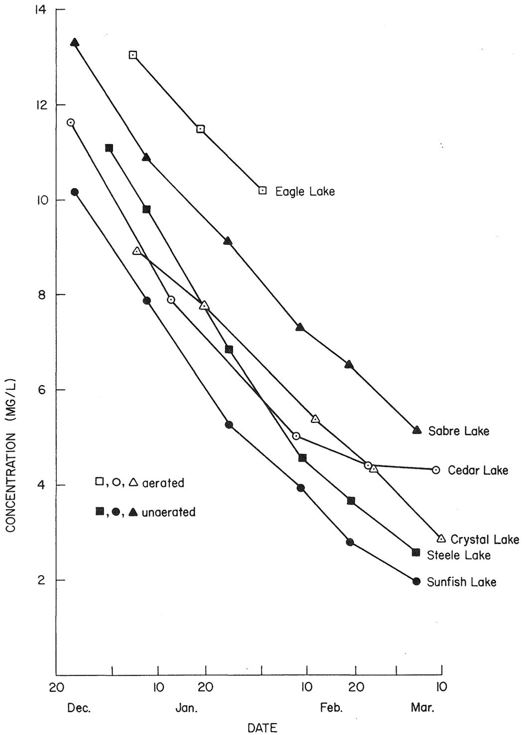
Figure 7. Volume-weighted mean lake oxygen concentrations of aerated and unaerated lakes, winter 1981-82.
