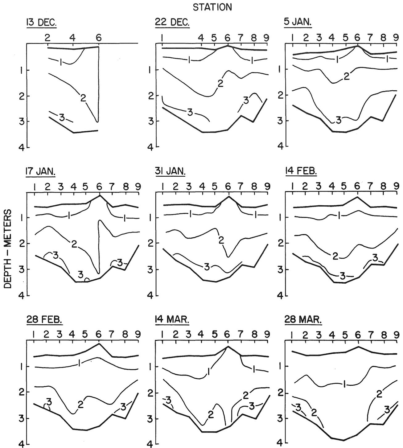
Figure 6. Isotherms ( $^{\circ}\text{C}$ ) in the Elysian Lake water column, winter 1978-79. Bold lines represent the underside of the ice layer and lake bottom.
