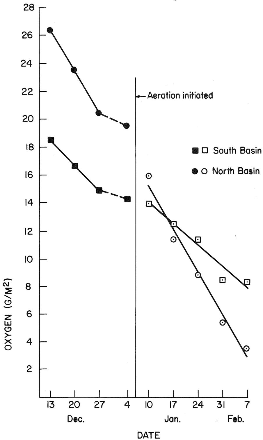
Figure 12. Oxygen mass (g/m<sup>2</sup> of surface area) before and after aeration began in Shetek Lake, winter 1983-84. Broken lines indicate intervals not included in regression analysis.
