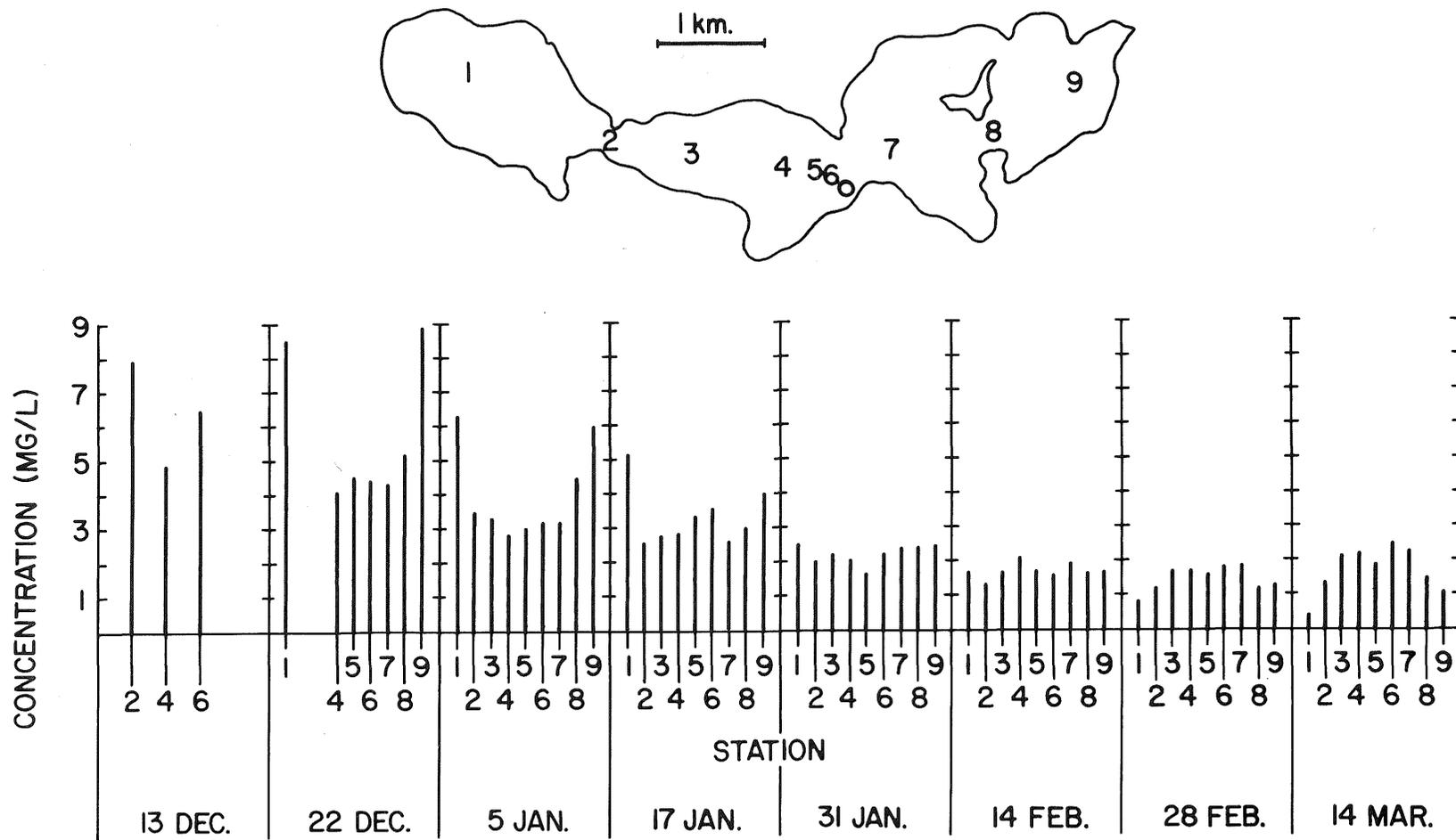
Figure 4. Elysian Lake sampling stations and mean water column dissolved oxygen concentrations (mg/l), winter 1978-79. Station 0 is the aeration site; Station 6 is 5-15 m from open water; Station 5 is 100 m from Station 6; others are to scale.
