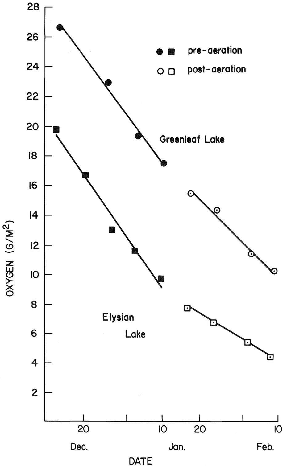
Figure 11. Oxygen mass ( $\text{g/m}^2$  of surface area) before and after aeration began in Greenleaf and Elysian Lakes, winter 1983-84.
