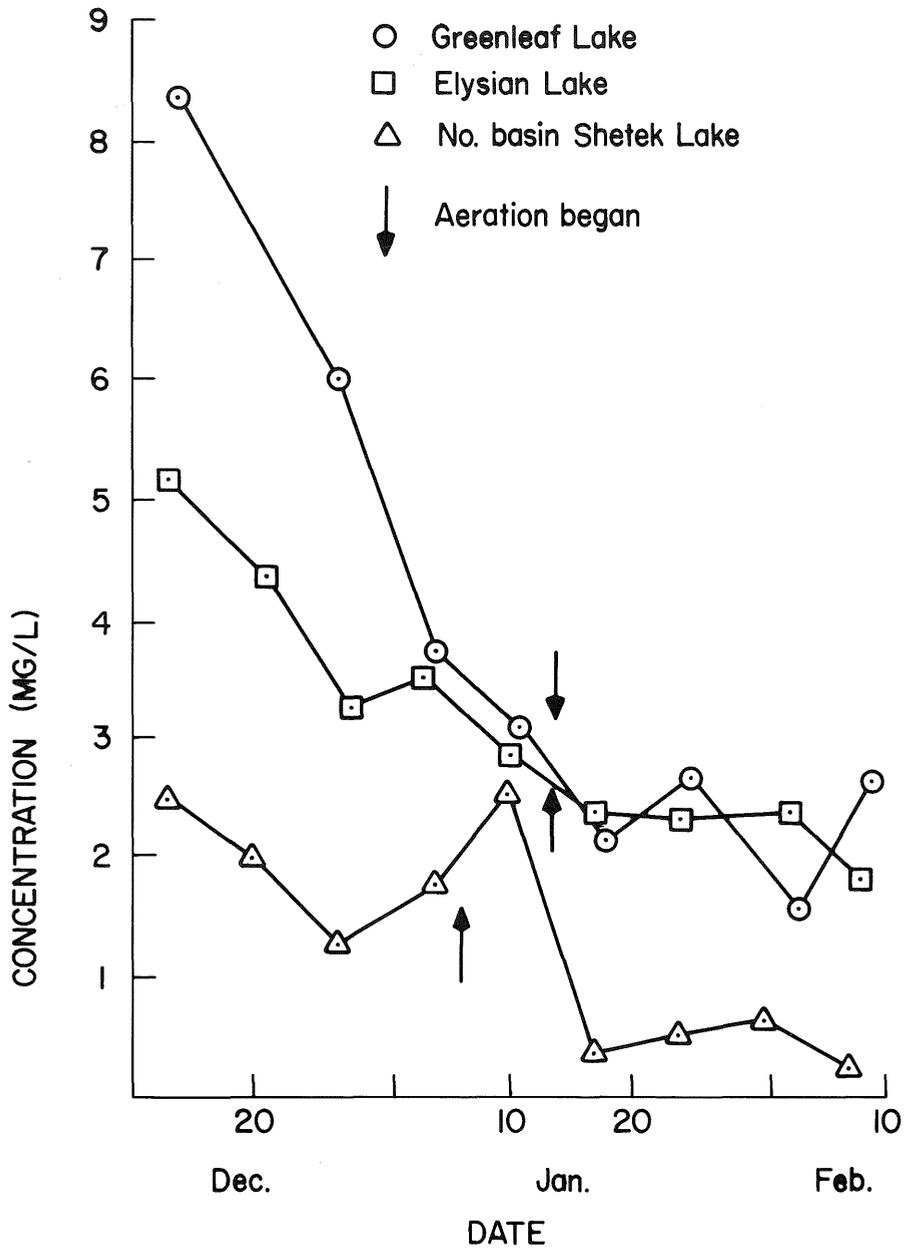
Figure 14. Mean station oxygen concentrations (mg/l) 20 cm above the bottom sediments in three lakes before and after aeration began, winter 1983-84.
