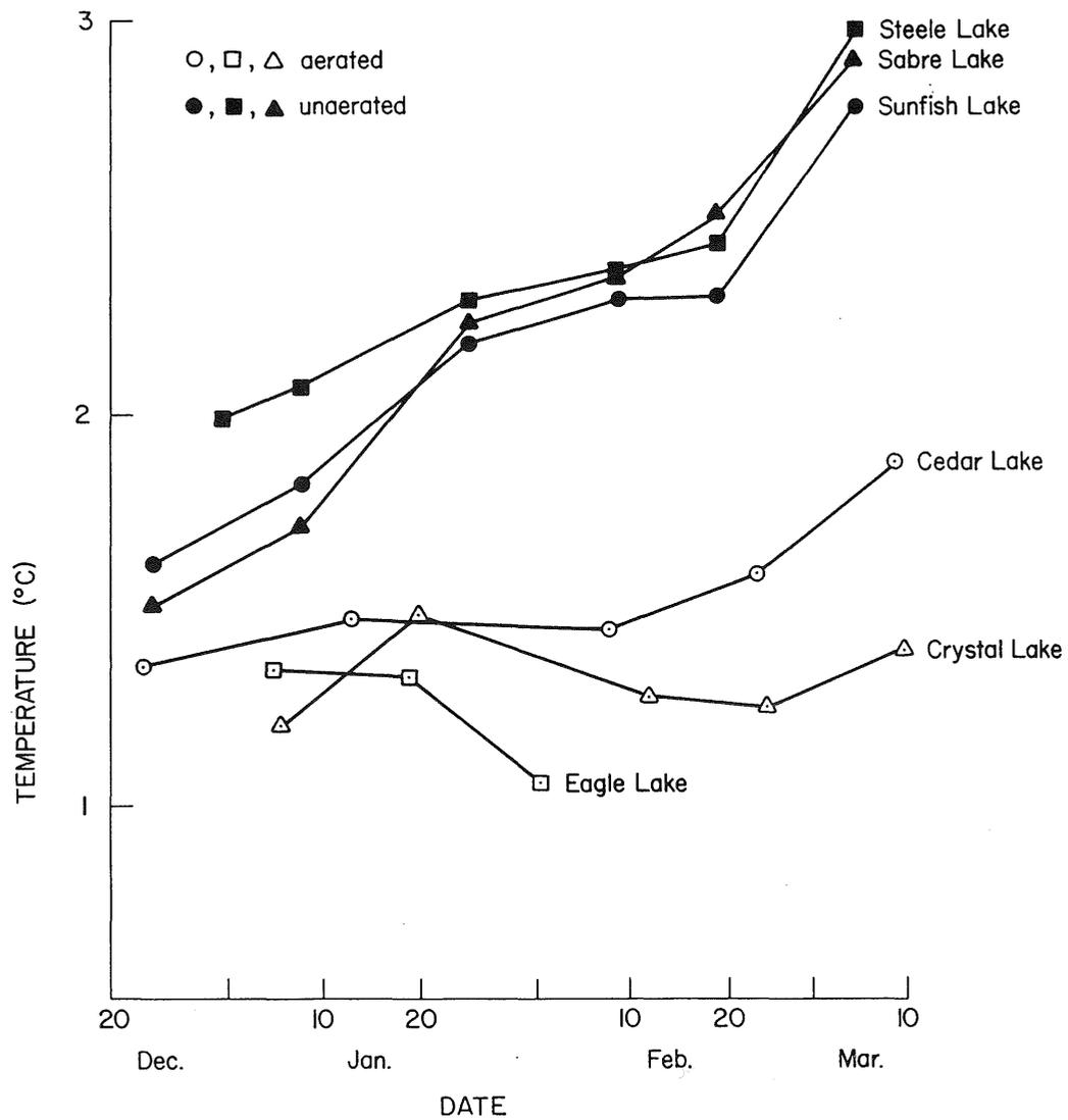
Figure 10. Volume-weighted mean lake temperatures ( $^{\circ}\text{C}$ ) of aerated and unaerated lakes, winter 1981-82.
