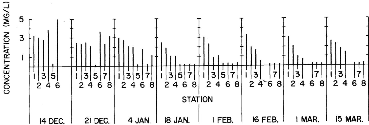
Figure 1. Lura Lake sampling stations, and mean water column dissolved oxygen concentrations (mg/l), winter 1978-79. Station 0 is the aeration site; Station 1 is 2-10 m from open water; Station 2 is 100 m from Station 1; others are to scale.
