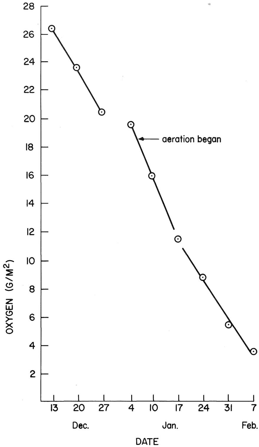
Figure 13. Oxygen mass ( $\text{g/m}^2$  of surface area) in the north basin of Shetek Lake before and after aeration began, winter 1983-84.
