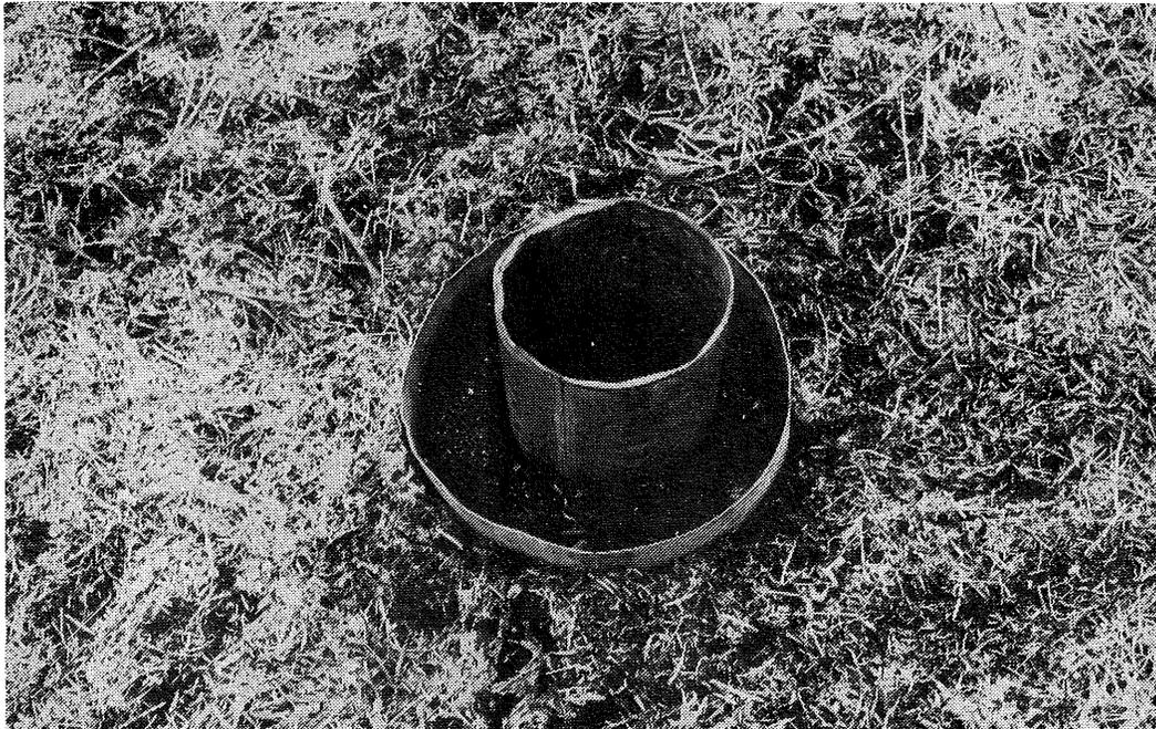
Figure 15. Photograph of double-ring infiltrometer at Fens.
