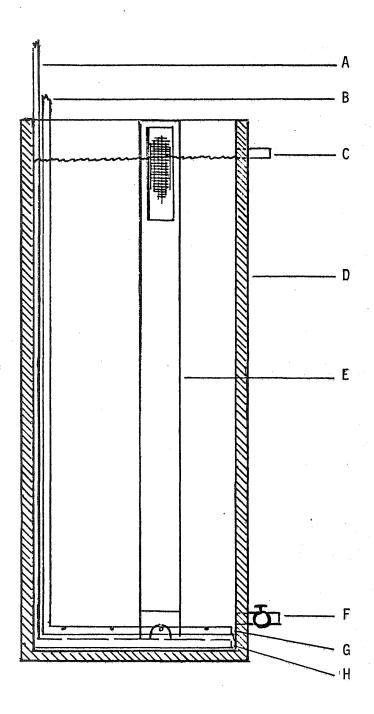
Fig. 3. Experimental incubator with air and water circulation systems. (A) air line, (B) water line, (C) water surface outlet, (D) insulated tank, (E) incubation tube, (F) water drain outlet, (G) water manifold, (H) air manifold.
