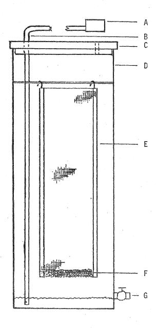
Fig. 2 System for experimental incubation of fish eggs in water-saturated air. (A) air pump, (B) air line, (C) removable top, (D) polyethylene tank, (E) egg container, (F) gravel, (G) water drain outlet.
