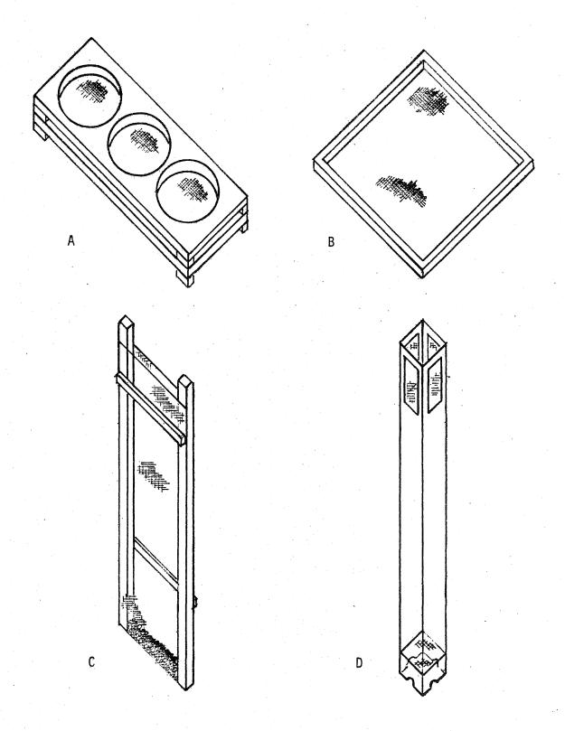
Fig. 1. Egg containers used in experimental incubation of fish eggs. (A), (B) screen-bottom trays, (C) vertical screened container, (D) incubation tube.
