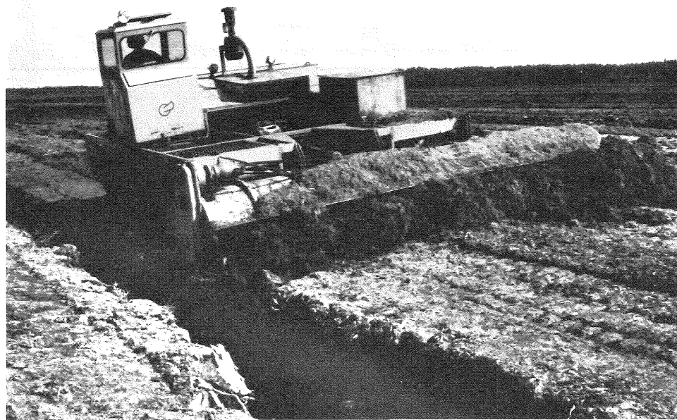
Ditching (left), the first step in the mining process, is necessary to drain the peatland so it can support heavy equipment such as the leveling machine (right), which prepares the surface of the peatland for mining.
