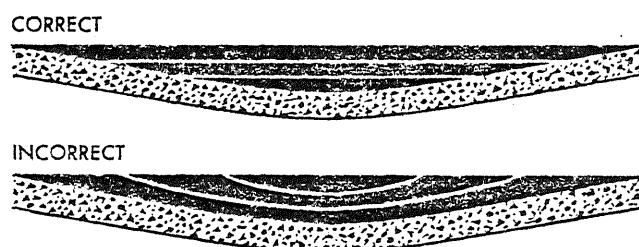
Figure 1—Correctly placed leveling wedges ensure smoother pavements
