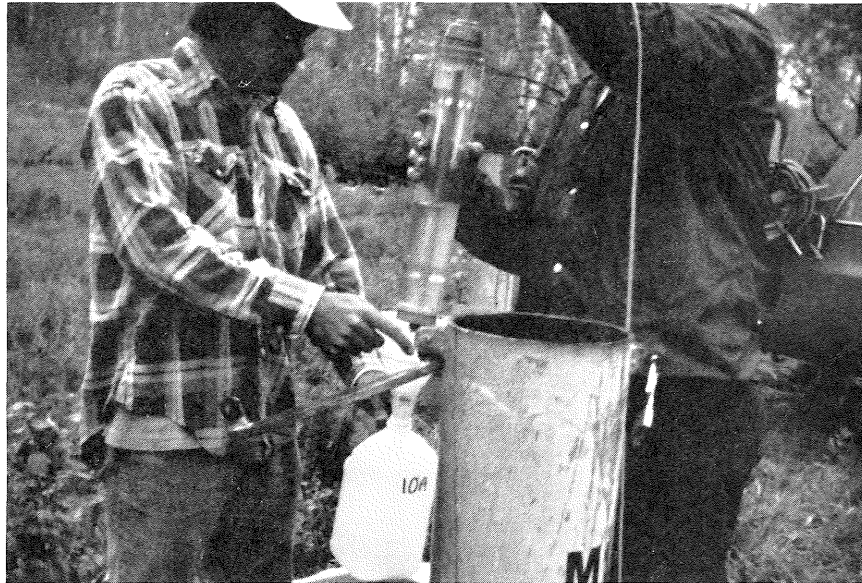
Figure 6. All Plastic Kemmler Sampler for Well Sampling
