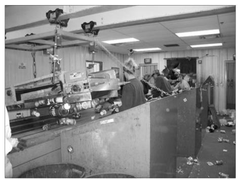
At the St. Louis County material recovery facility, shown here, a magnet separates steel cans and workers hand-separate glass, plastic, and aluminum containers from a commingled recycling stream.
