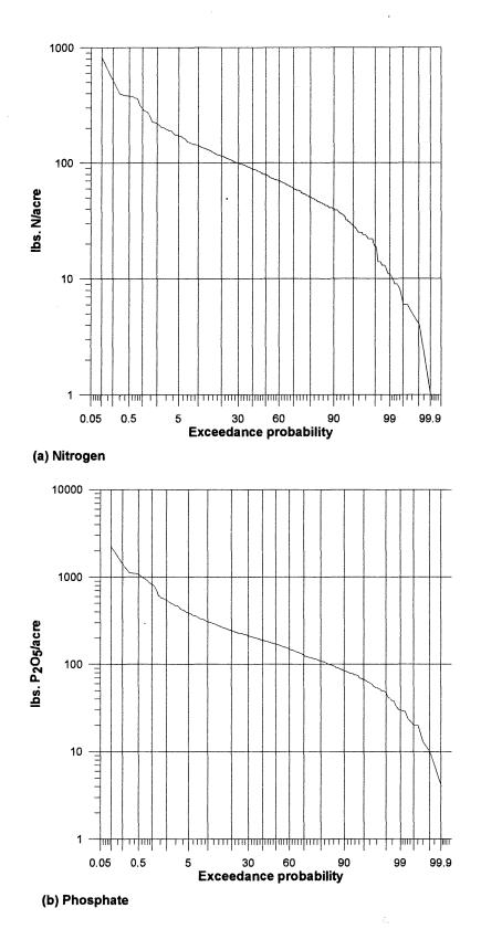
Figure 12. Probability plots of single-year available manure (a) N and (b)  $P_2O_5$  applications within a watershed.
