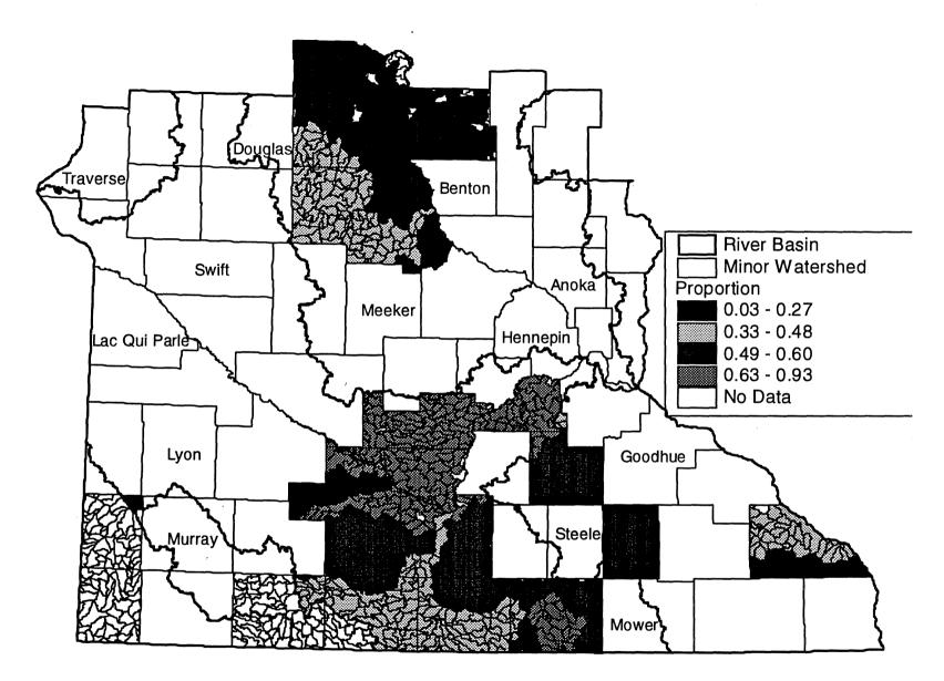
Figure 25. Proportion of surface water samples that exceed 0.25 mg/L at the major watershed outlet.
