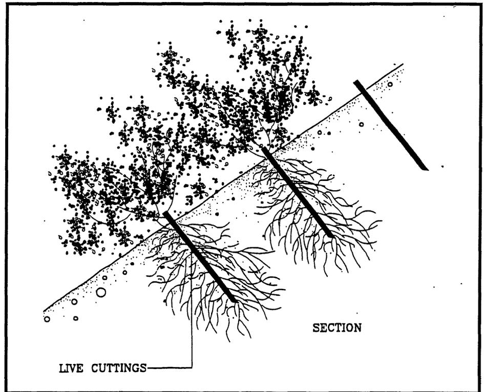
**Figure 4: Schematic diagram of an established, growing live stake installation.** From *Biotechnical and Soil Bioengineering Slope Stabilization, A Practical Guide for Erosion Control*, by Donald H. Gray and Robbin B. Sotir, John Wiley & Sons, 1996. Reprinted by permission of John Wiley & Sons, Inc.
