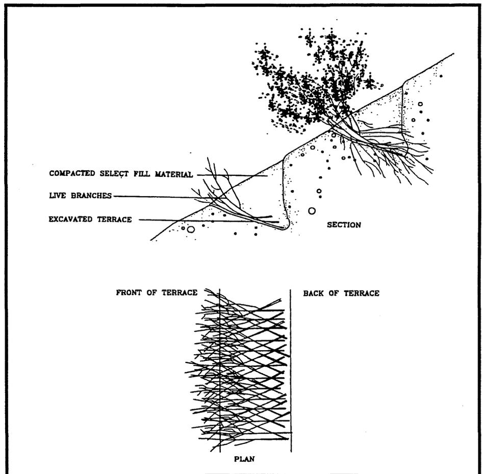
**Figure 8: Schematic diagram of an established, growing cut slope brush layer installation**, showing alternating layers of live cut brush placed on narrow benches or terraces excavated in the slope. From *Biotechnical and Soil Bioengineering Slope Stabilization, A Practical Guide for Erosion Control*, by Donald H. Gray and Robbin B. Sotir, John Wiley & Sons, 1996. Reprinted by permission of John Wiley & Sons, Inc.
