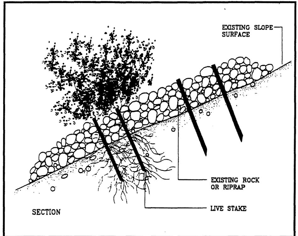
**Figure 9: Schematic diagram of an established, growing vegetated riprap joint planting.** From *Biotechnical and Soil Bioengineering Slope Stabilization, A Practical Guide for Erosion Control*, by Donald H. Gray and Robbin B. Sotir, John Wiley & Sons, 1996. Reprinted by permission of John Wiley & Sons, Inc.
