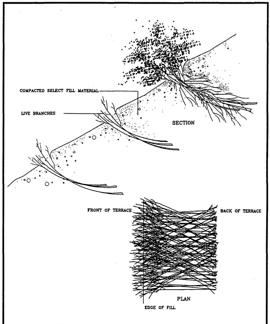
**Figure 7: Schematic diagram of an established, growing fill slope brush layer installation, showing alternating layers of live cut brush inserted between lifts of soil.** From *Biotechnical and Soil Bioengineering Slope Stabilization, A Practical Guide for Erosion Control*, by Donald H. Gray and Robbin B. Sotir, John Wiley & Sons, 1996. Reprinted by permission of John Wiley & Sons, Inc.
