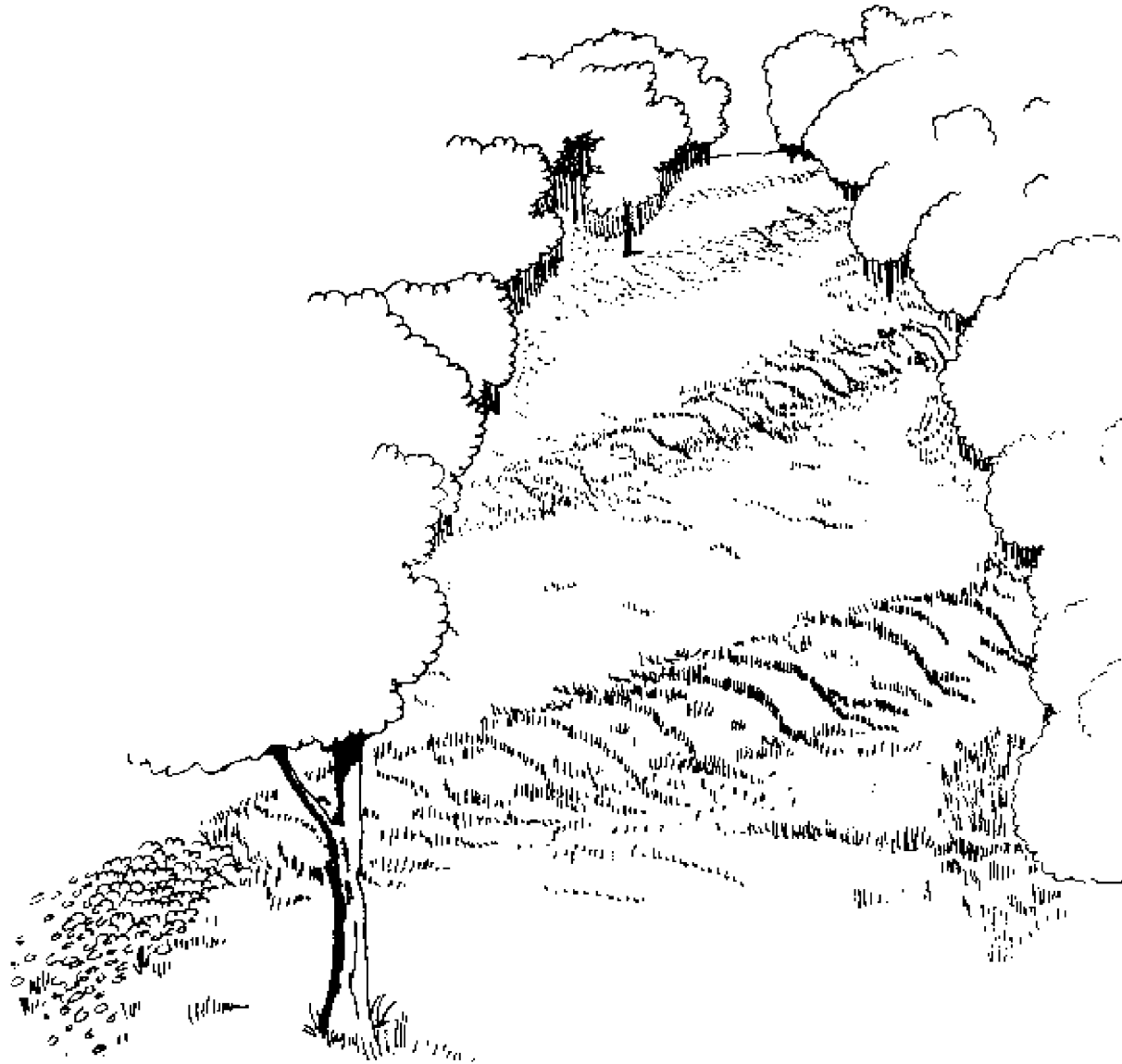
Figure 6.14-1 Water bars to protect utility right-of-way (source: North Carolina, May 1994)
