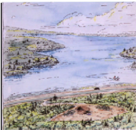
Figure TH-9: In visually sensitive areas, a recommended practice is to avoid placing landings within view of travel routes or recreational areas. The landing and slash piles above are in full view of travelers and recreational users along the adjacent travel route and waterway. The landing and slash piles below are hidden from the travel route and waterway as a result of the dogleg access road.
