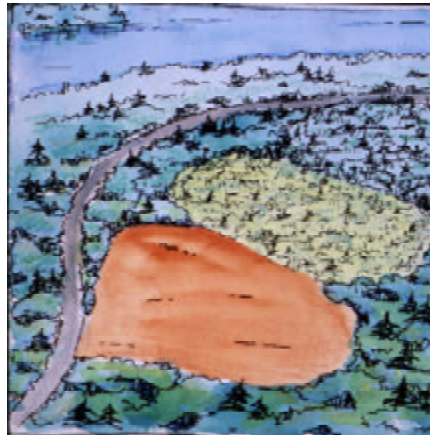
Figure TH-7: Multiple-stage cutting (right) can reduce apparent harvest area size.
