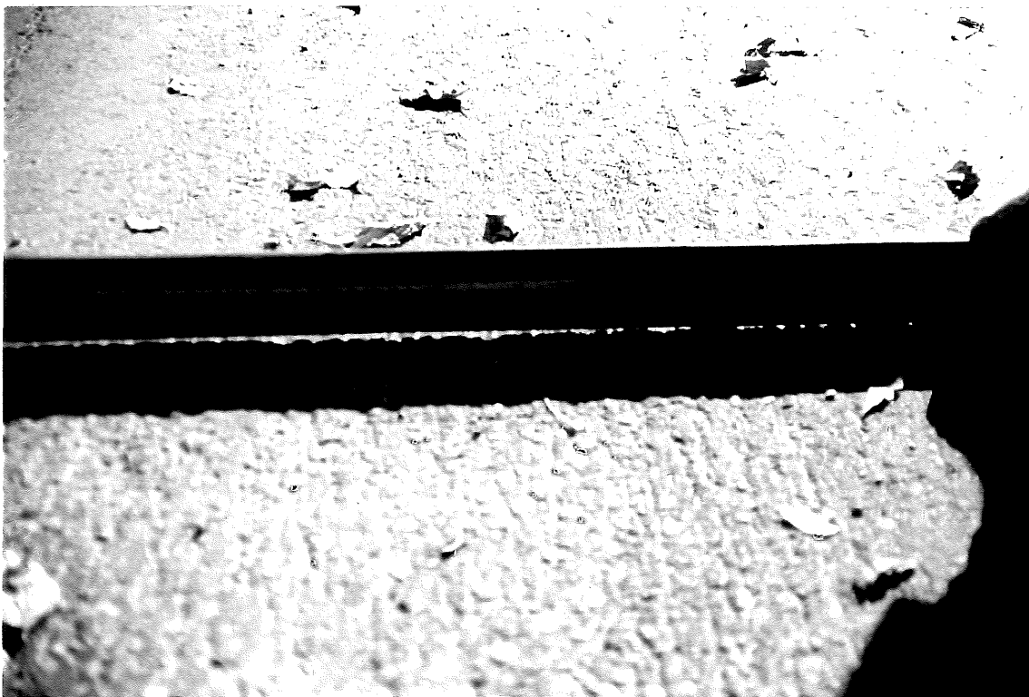
Straight-edge across the trail illustrates surface irregularities
