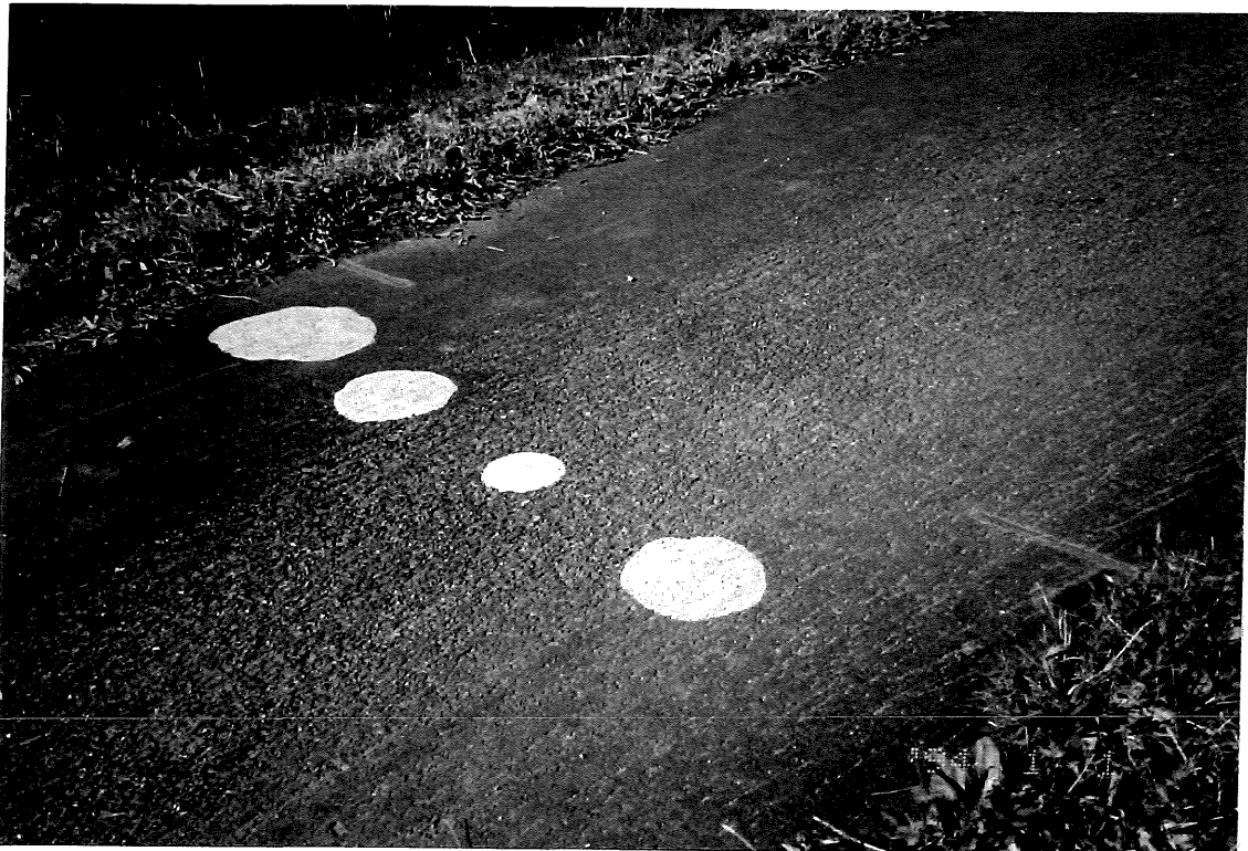
Typical test area (Note the differences in diameter of circles. The smaller circles indicate asphalt that has more grooves and abrasion; the larger circles indicate smoother asphalt.)
