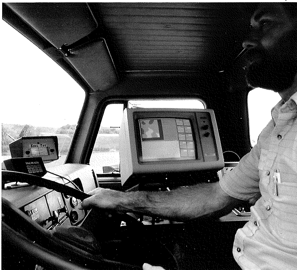
Computerized soil maps help vary the amount of fertilizer applied to different parts of a field.
