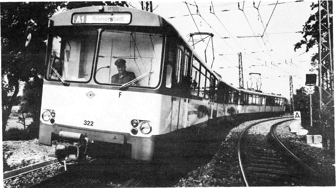
Light rail transit reaches the highest level of performance when located on its own right-of-way as demonstrated by this Frankfurt, West Germany suburban line. The U-2 type vehicle has also been delivered to Edmonton, Calgary and San Diego.
