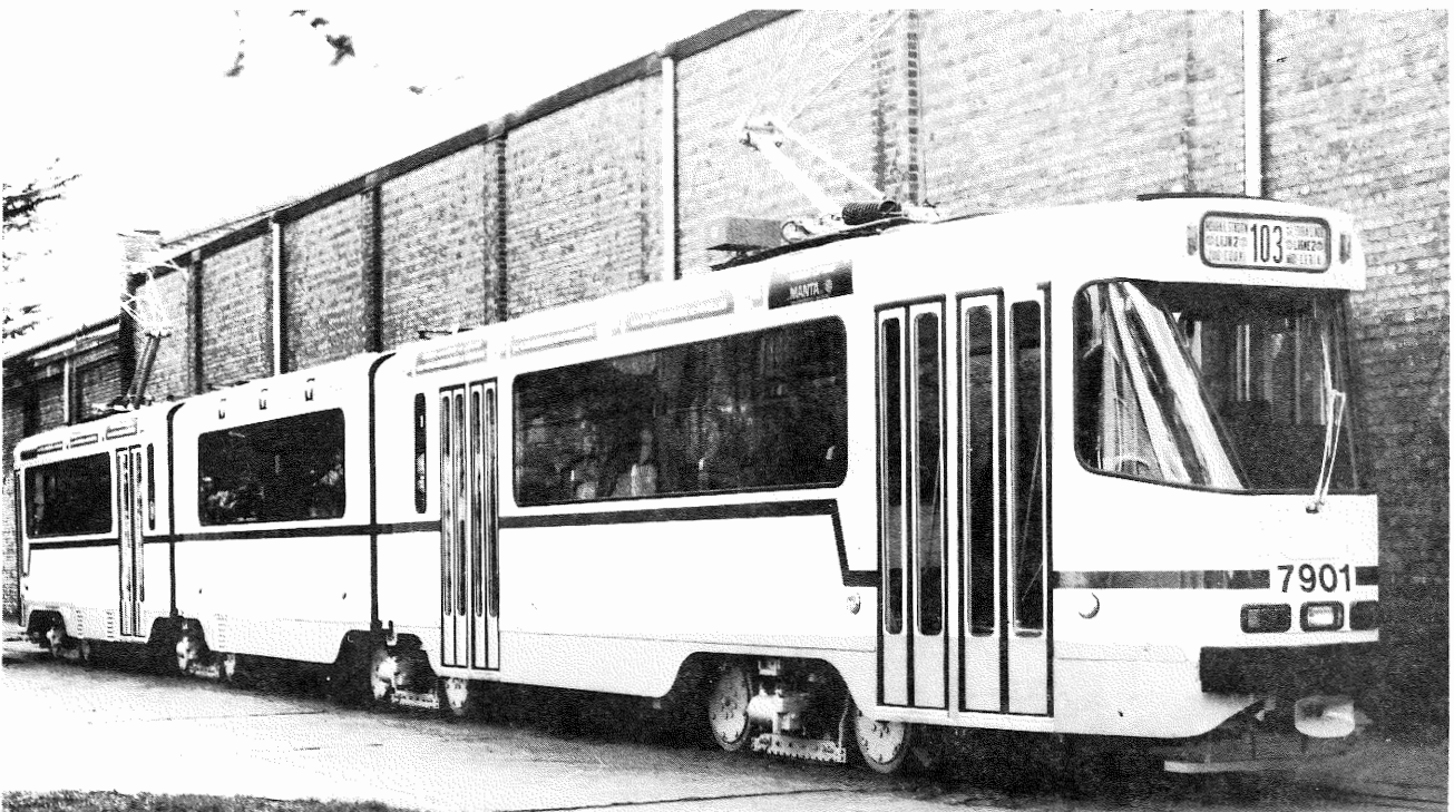
These three-unit vehicles were manufactured in Belgium for the expanding Brussels "premetro" light rail transit system. All trucks are powered.
