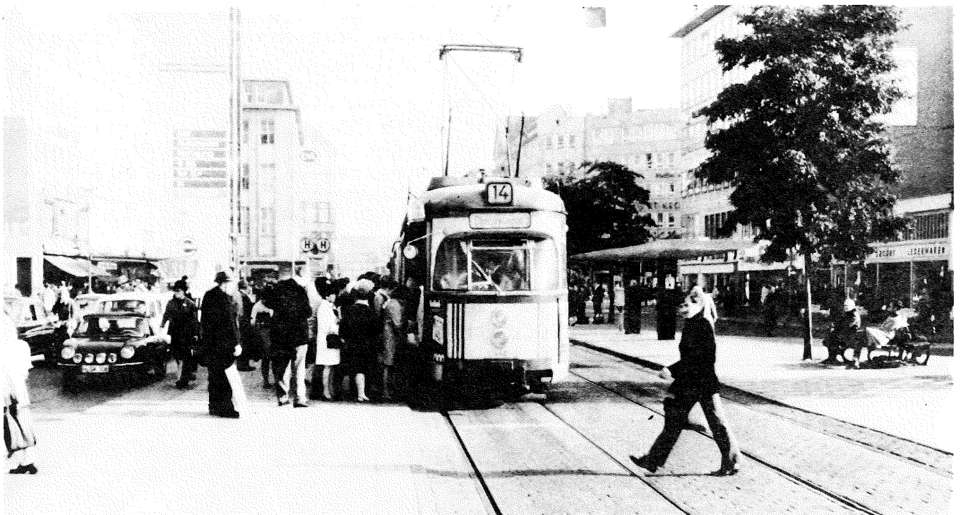
Downtown alignments in street medians or pedestrian malls provide the highest degree of passenger access at minimal cost. Operations can be speeded by LRT preemption of traffic signals.
