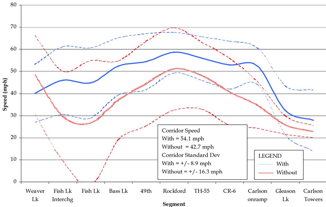
**Figure 5.3 I-35W NB Morning Speed and Speed Variability**
