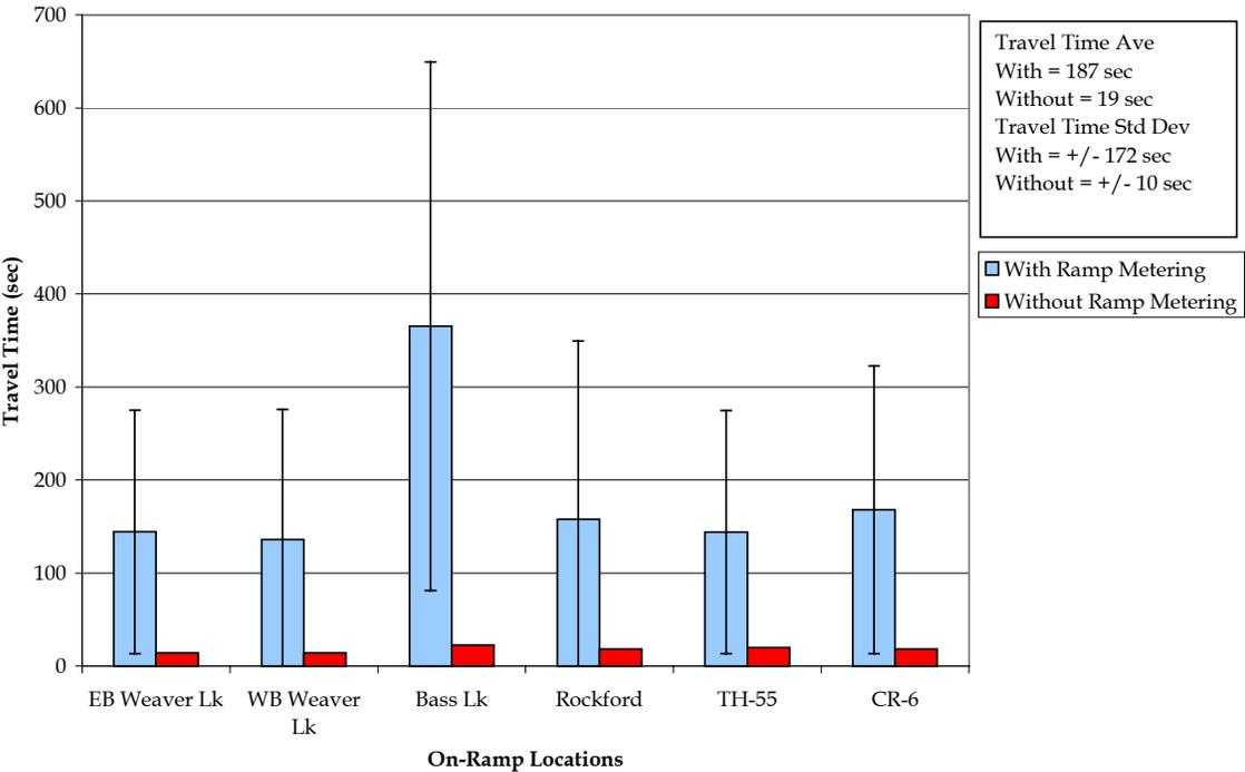
**Figure 5.24 I-35W NB Morning Ramp Travel Time**
