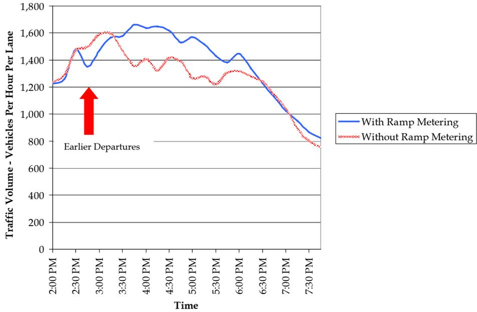
**Figure 9.2 I-35E Southbound Morning – Example of Traffic Volume Reduction**
