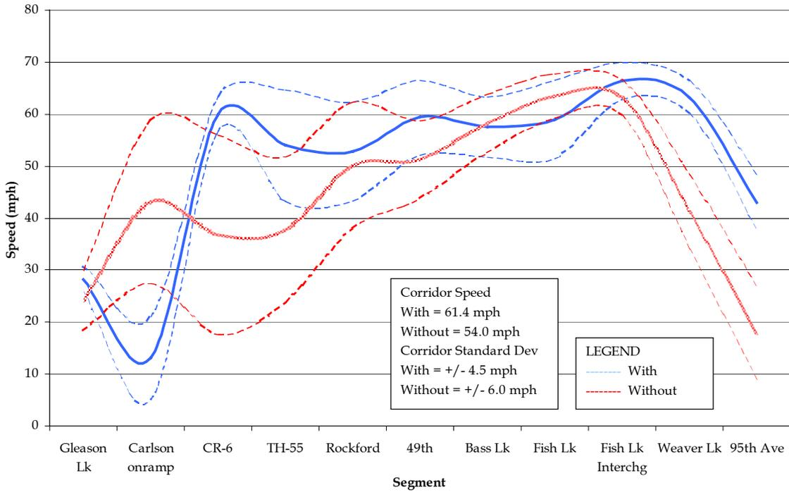
**Figure 5.2 I-494 SB Morning Speed and Speed Variability**
