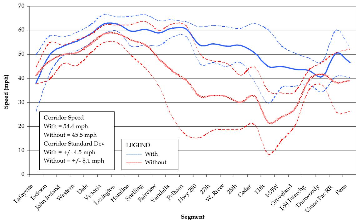
**Figure 5.7 I-35E NB Afternoon Speed and Speed Variability**
