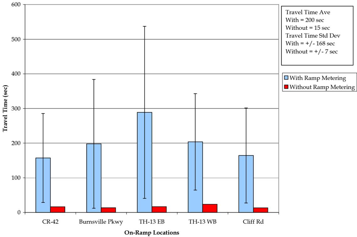
**Figure 5.25 I-94 EB Afternoon Ramp Travel Time**
