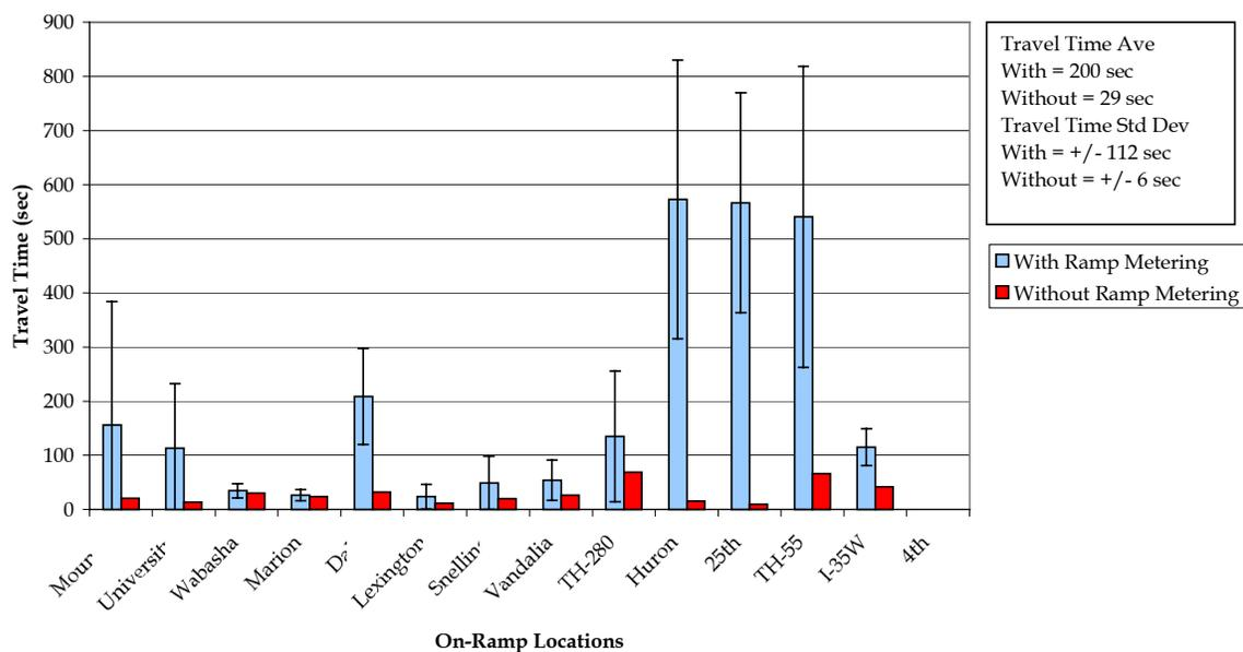
**Figure 5.28 I-35E NB Afternoon Ramp Travel Time**
