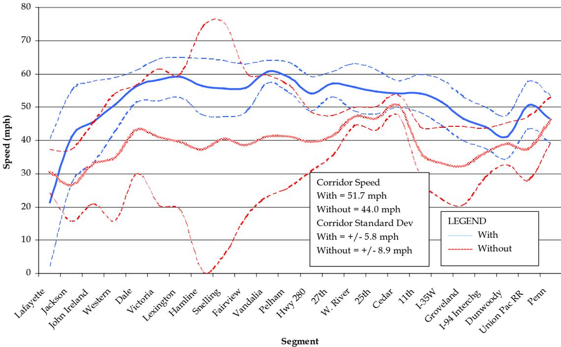
**Figure 5.6 I-94 WB Afternoon Speed and Speed Variability**
