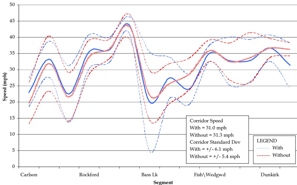
**Figure 5.11 Vicksburg Avenue NB Afternoon Speed and Speed Variability**
