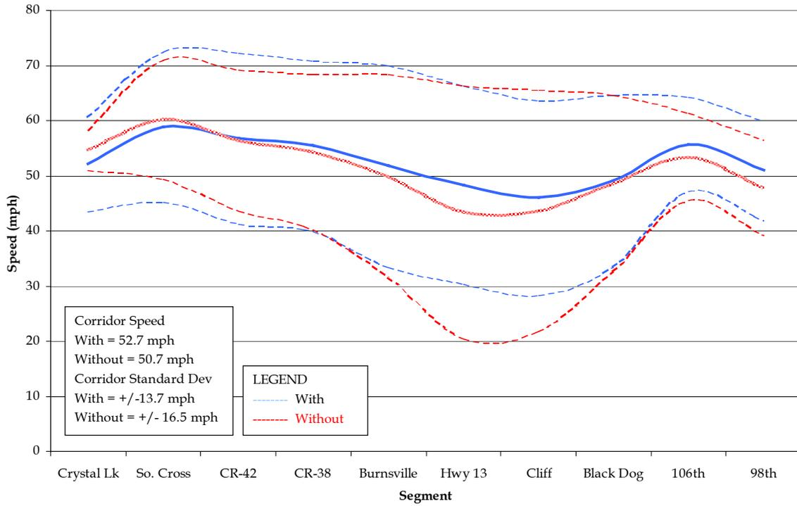
**Figure 5.4 I-94 EB Afternoon Speed and Speed Variability**
