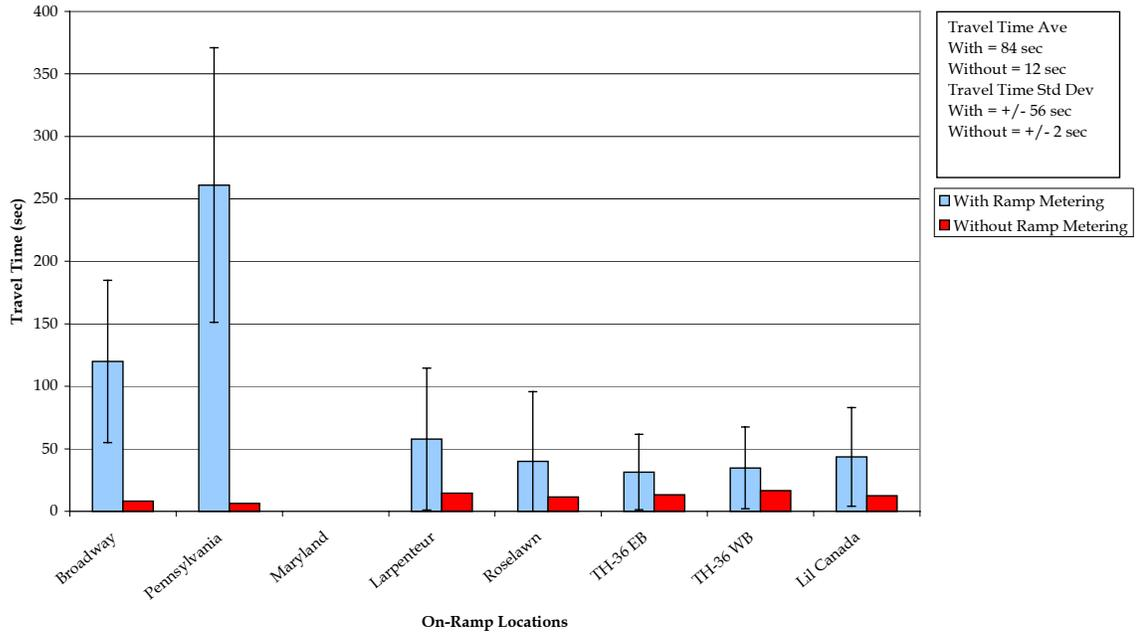
**Figure 5.29 I-35E SB Morning Ramp Travel Time**
