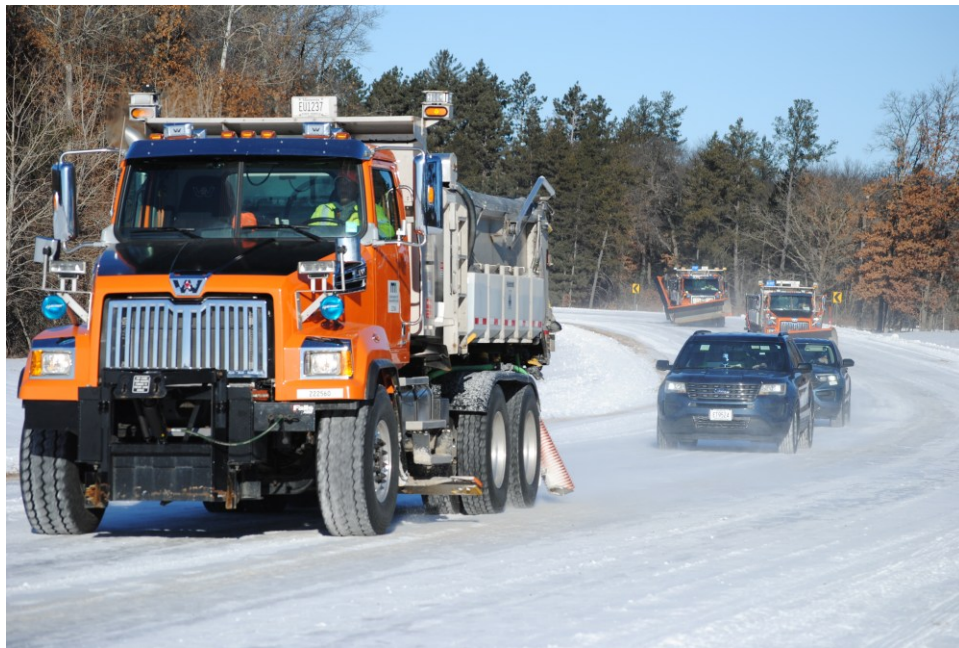
Figure 8. Typical traffic applied to perimeter track.
