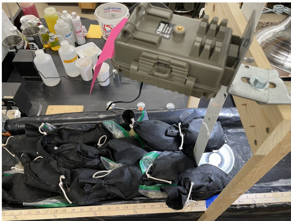
Figure 3.7 Use of flow seals (Ziplocks) experiment.
