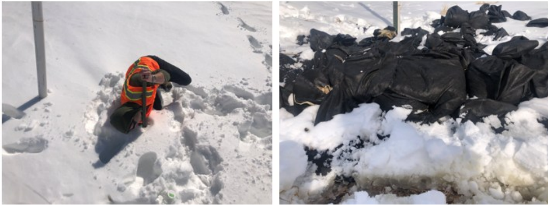
Figure 4.14 Ditch water flowing as a thin layer through the base of the snowpack then through the treatment berm; Sterling North location, March 7, 2025.
