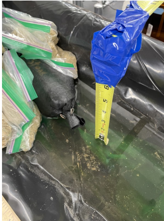
Figure 3.6 Treatment media bag relative permeability and flow direction experiment.
