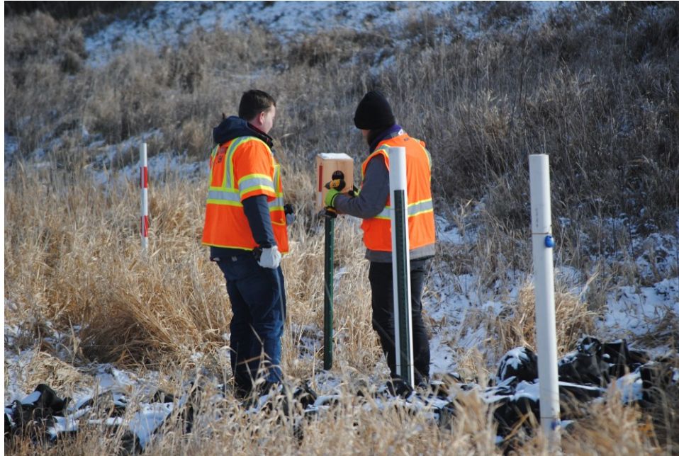
Figure 4.9 Instrumentation installation December 3, 2024. From left to right along ditch line: snowmobile warning post with reflective tape, time lapse camera being installed in an imitation “bird house” on post, post and PVC standpipe for ditch water access up
