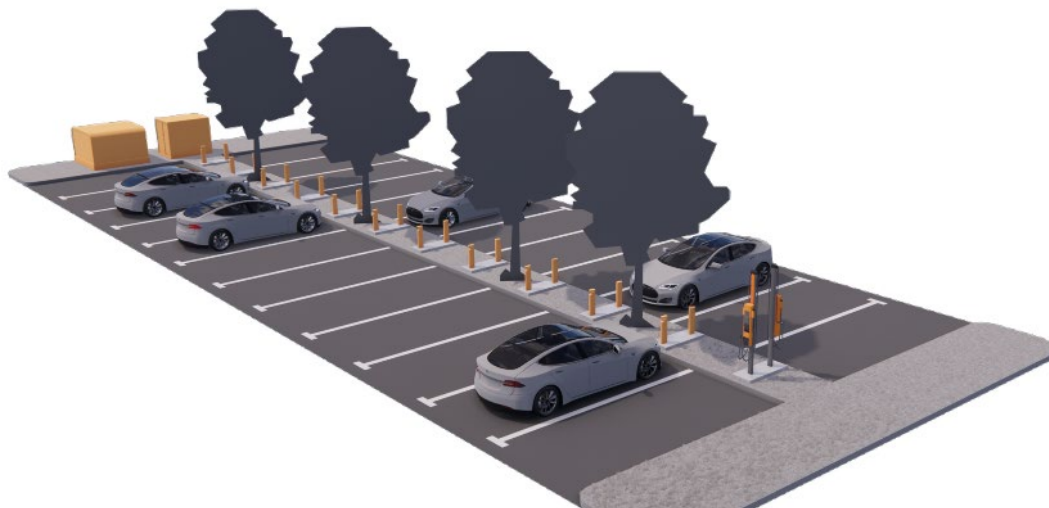
Figure 7: Example of Level 2 Destination Charging Hub
