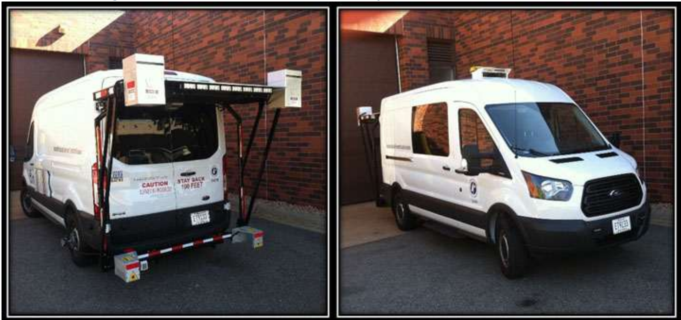
Figure 2. Network-Level Pavement Surface Data Collection Vehicle
