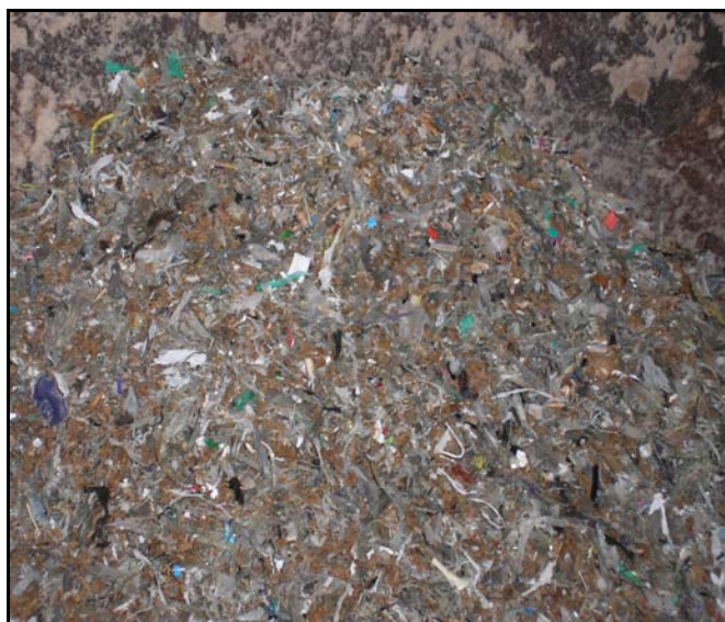
Figure 7: Debris Removed From Recycled Paper Slurry
