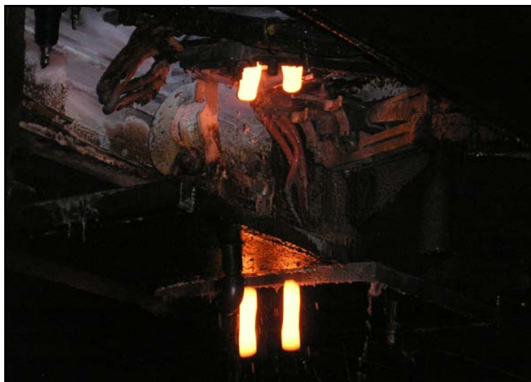
Figure 9: Sheering of Molten Glass
