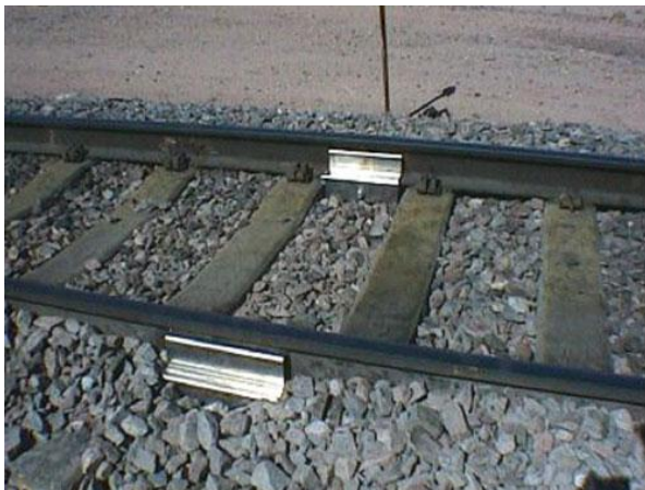
Figure 16: Example of a Truck Performance Detector with Strain Gauges
