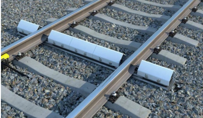
Figure 4: An Example of a Fixed Accelerometer Dragging Equipment Detector
