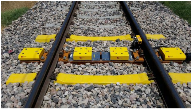
Figure 18: Hot Bearing (Outer) and Hot Wheel (Inner) Detector Co-location
