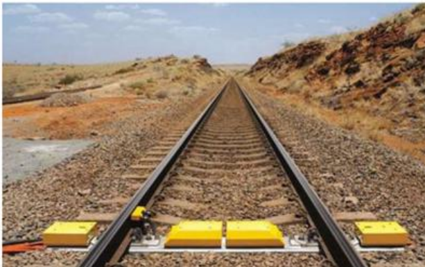
Figure 3: An Example of a HBD System (Outer Detectors) and a HWD System (Inner Detectors)
