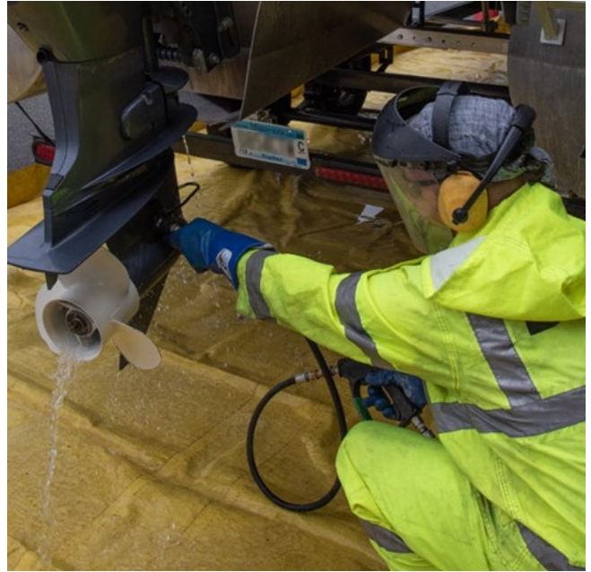
Figure 15. Level 2 Inspector Matt Dwelly conducts an engine decontamination on a pontoon boat's outboard motor.
