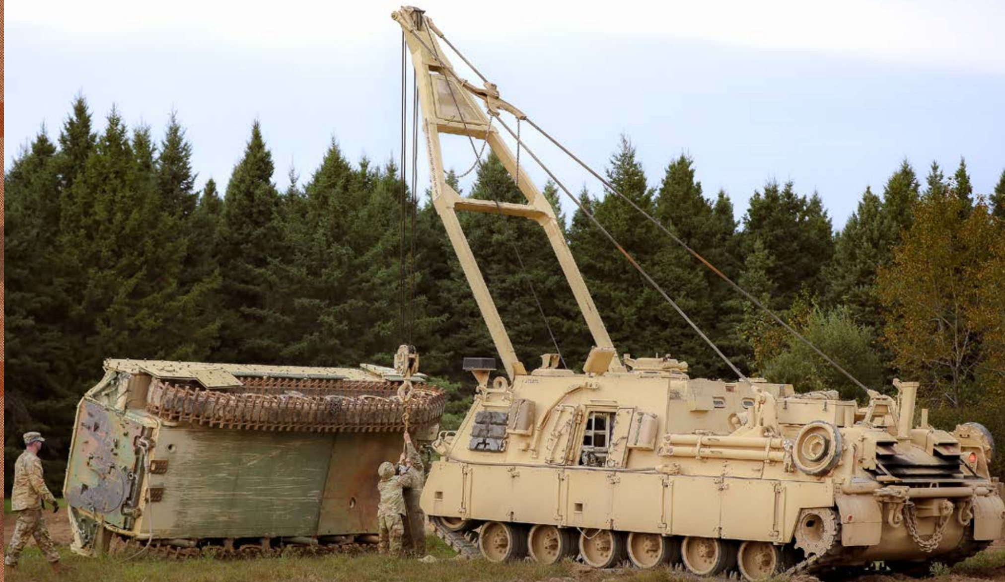
The Regional Training Site-Maintenance hosted a track vehicle recovery course for Soldiers, utilizing the M88 Hercules recovery vehicle to tow M1 Abrams Tanks, M109 Paladin howitzers, and more, Sept. 12, 2025, Camp Ripley, near Little Falls, Minnesota
