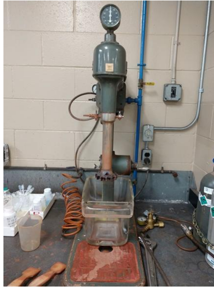
Figure 9. Flotation experimental set-up at NRRI.
