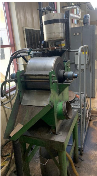
Figure 7. Wet low-intensity magnetic separator at NRRI.
