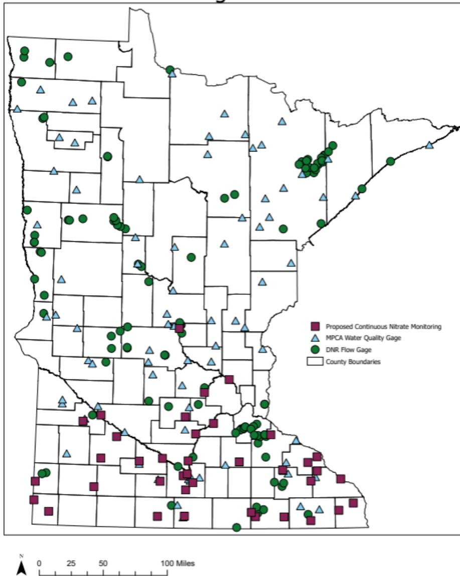
This map shows active stream gaging locations. All points represent the DNR streamflow quantity monitoring network. The blue triangles are sites where MPCA also collects water quality samples. The red squares show the locations where MPCA collects water quality samples and has or will be installing continuous nitrate sensors using the one-time appropriated funds from the FY24 legislative session.
