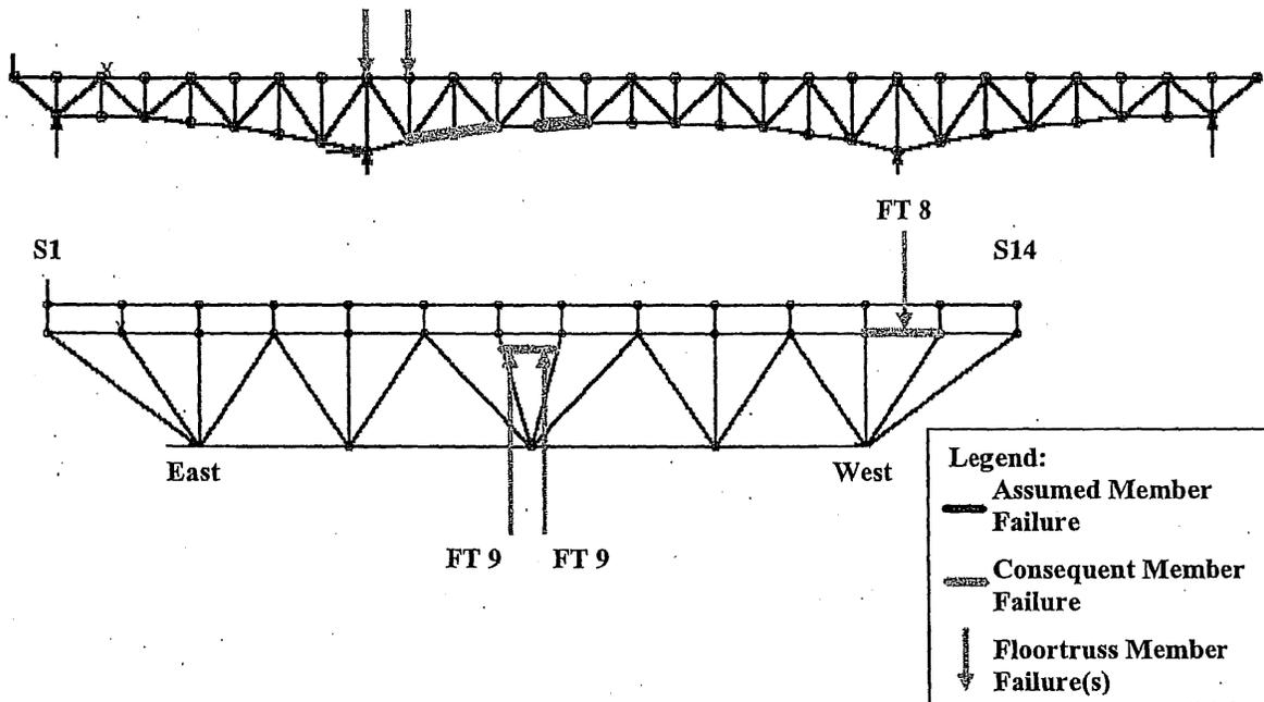
Figure 6-32: Load Case 2 – Failure of East Truss Lower Chord L12-L13
