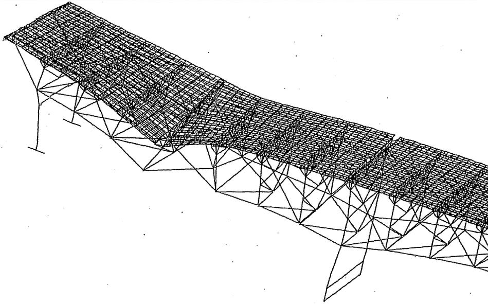
**Figure 6-11: Deformed Shape after Failure of East Truss Lower Chord L4-L5**
