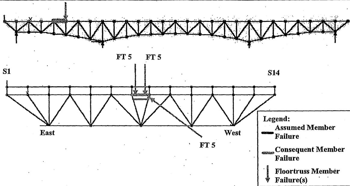
Figure 6-25: Load Case 2 – Failure of East Truss Upper Chord U4-U5
