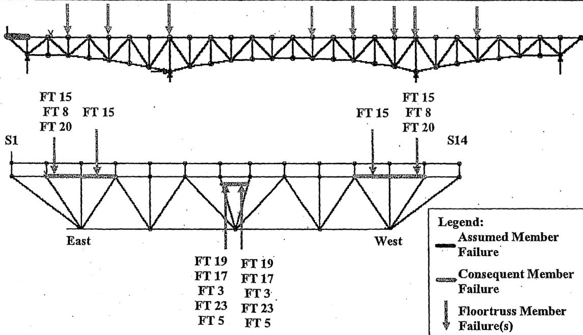
Figure 6-41: Load Case 3 – Failure of East Truss Upper Chord U0-U1
