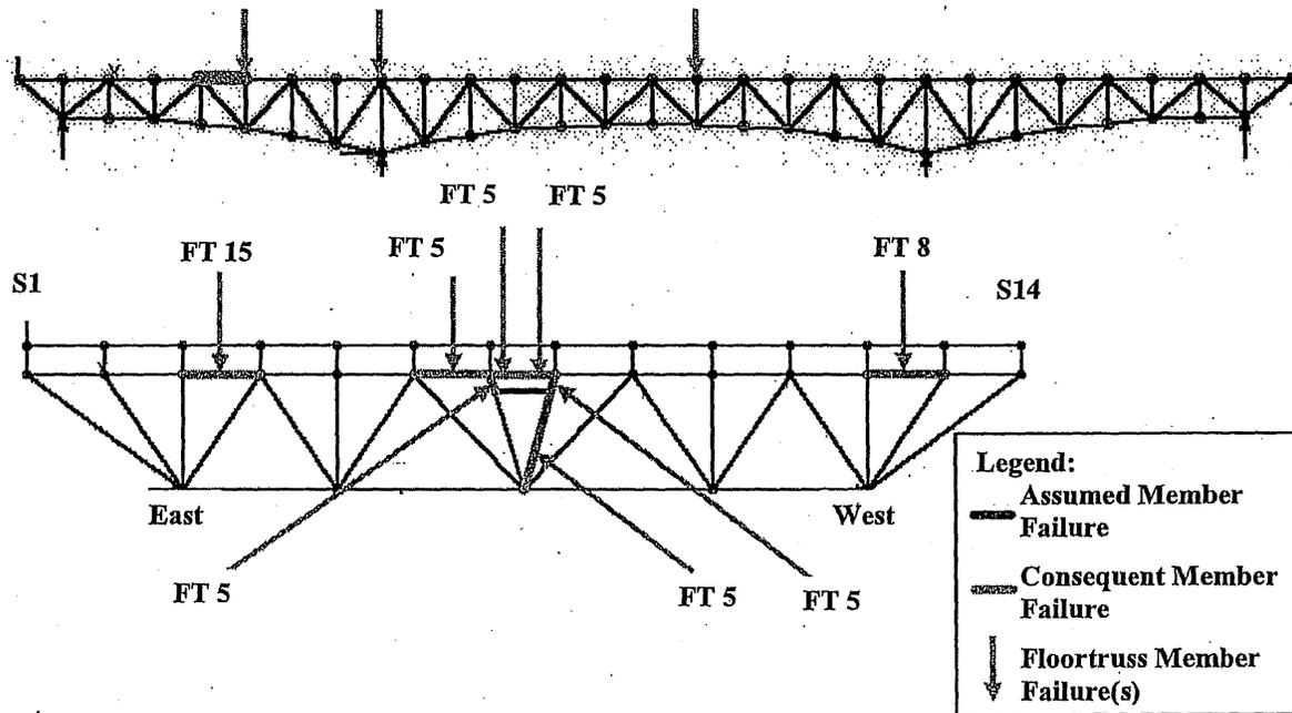
Figure 6-26: Load Case 2 – Failure of East Truss Upper Chord U4-U5
