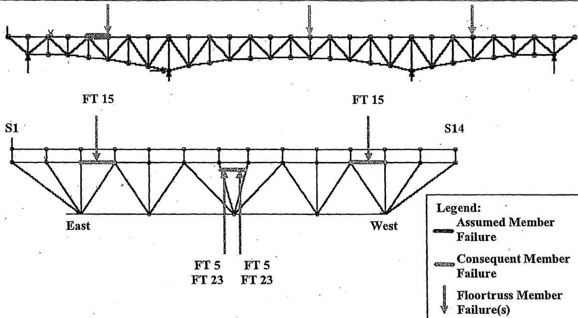
**Figure 6-24: Load Case 2 – Failure of East Truss Upper Chord U4-U5
