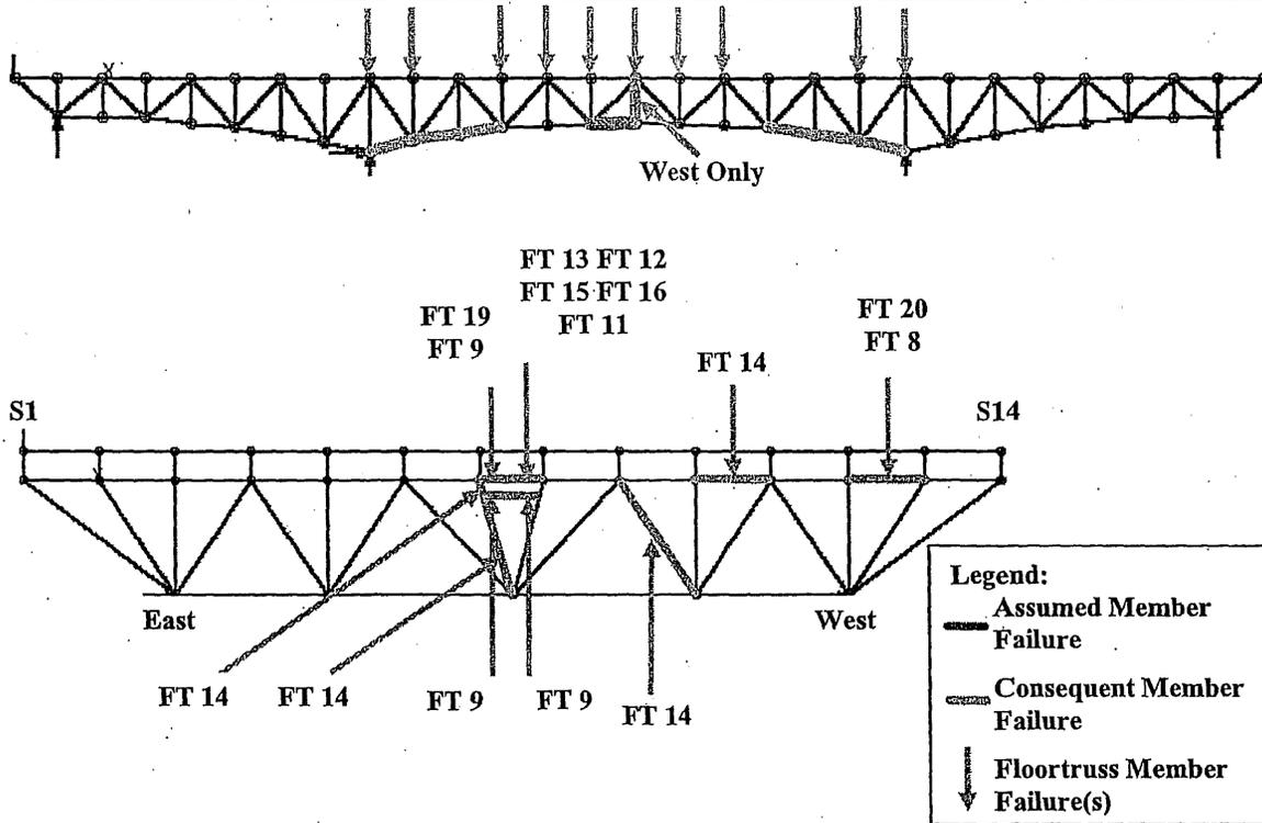
Figure 6-73: Load Case 4 – Failure of East Truss Lower Chord L13-L14
