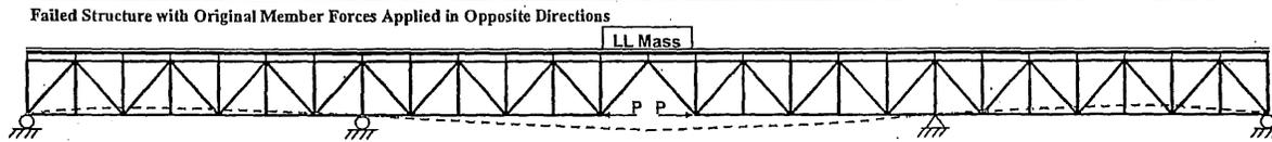
Figure 6-3: Sudden Member Failure as a Dynamic Step Load Consisting of a Pair of Forces
