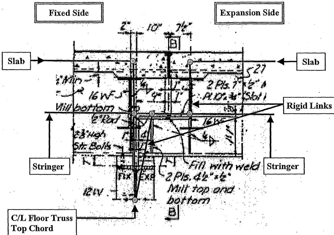
Figure 3-11: Stringer and Deck Expansion Joints
