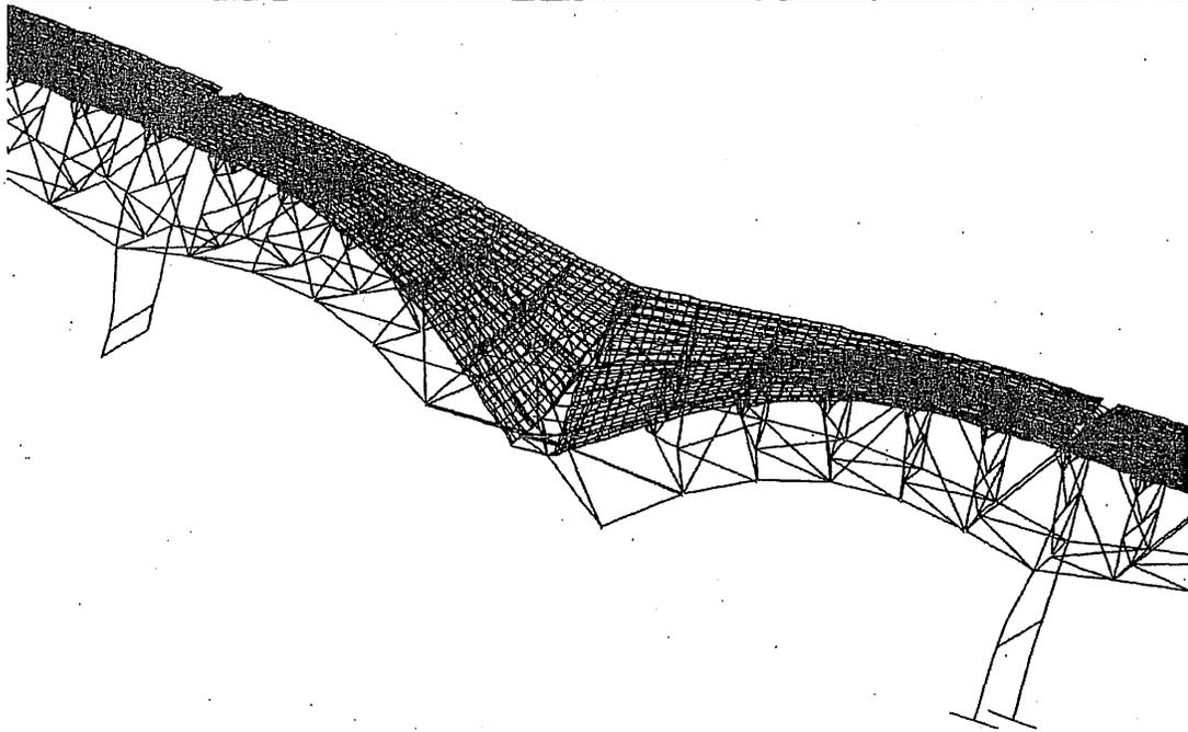
**Figure 6-13: Deformed Shape after Failure of East Truss Lower Chord L13-L14**
