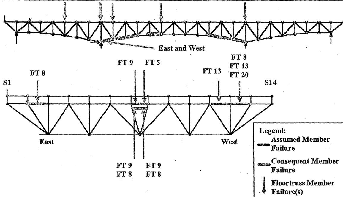
**Figure 6-51: Load Case 3 – Failure of East Truss Lower Chord L12-L13
