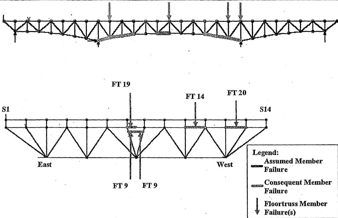
Figure 6-72: Load Case 4 – Failure of East Truss Lower Chord L13-L14
