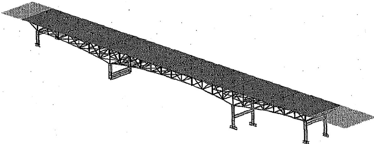
**Figure 3-1. Overview of Bridge 9340 Computer Model**
