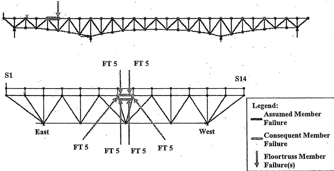
Figure 6-17: Load Case 1 – Failure of East Truss Upper Chord U4-U5
