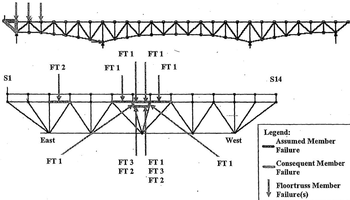
Figure 6-22: Load Case 2 – Failure of East Truss Upper Chord U0-U1
