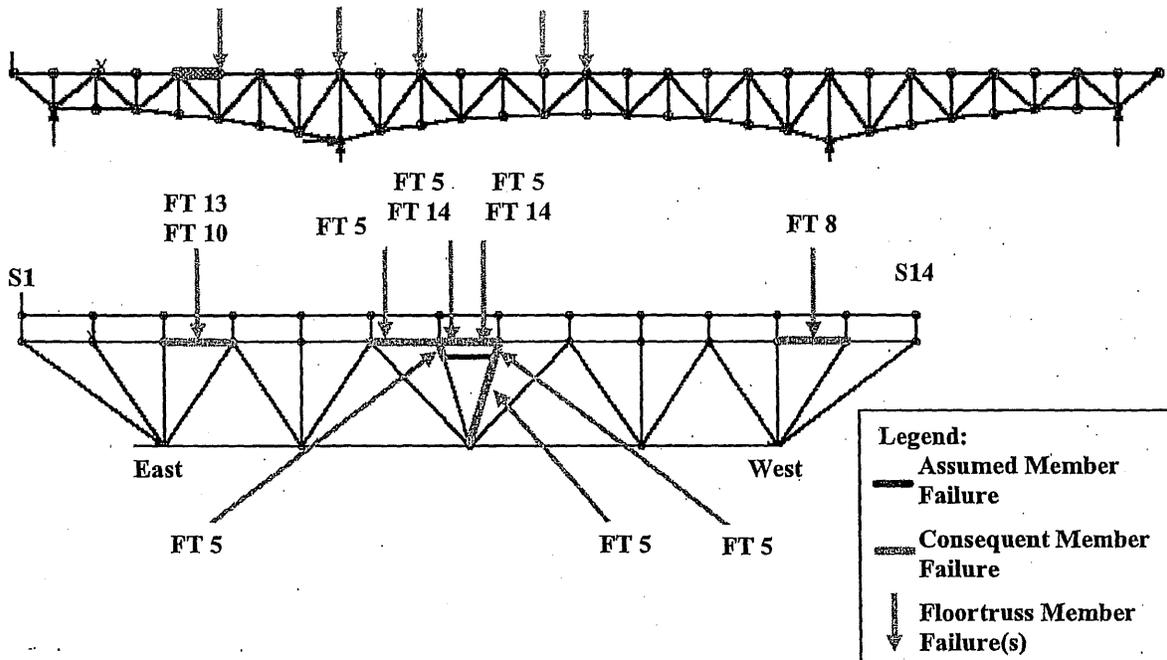
Figure 6-46: Load Case 3 – Failure of East Truss Upper Chord U4-U5
