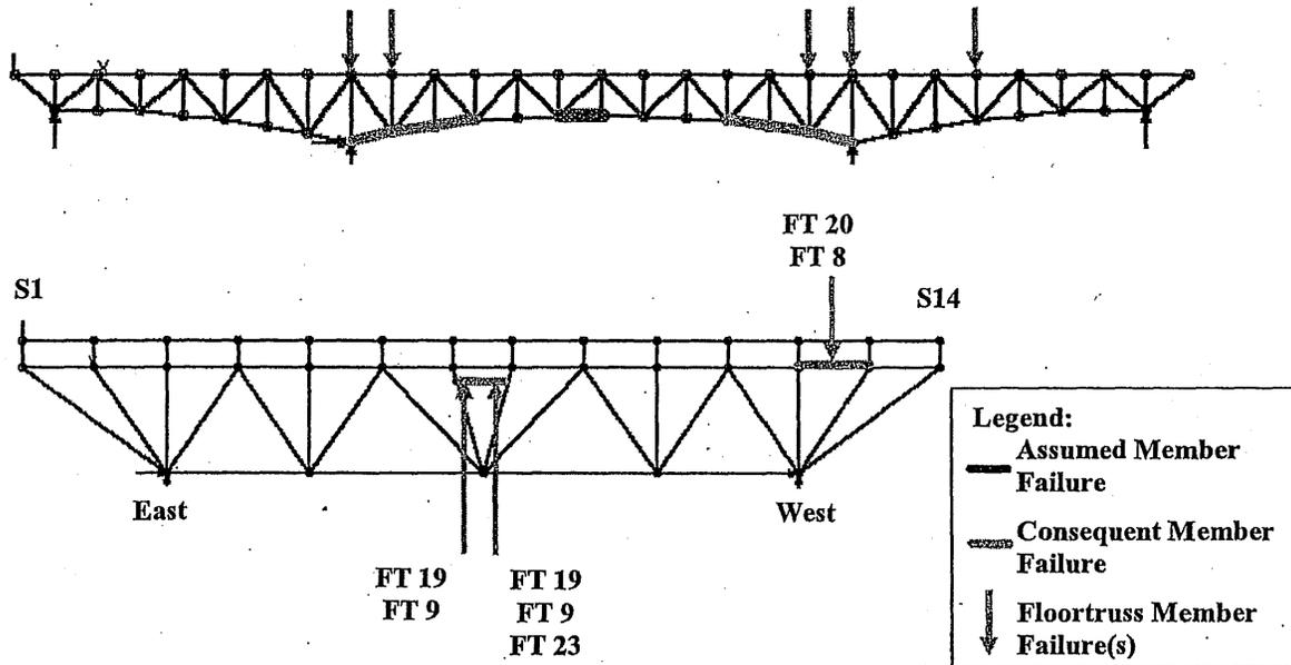
Figure 6-21: Load Case 1 – Failure of East Truss Lower Chord L13-L14
