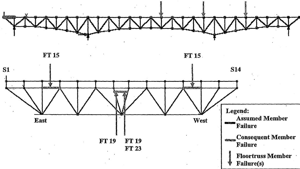
Figure 6-58: Load Case 4 – Failure of East Truss Upper Chord U0-U1
