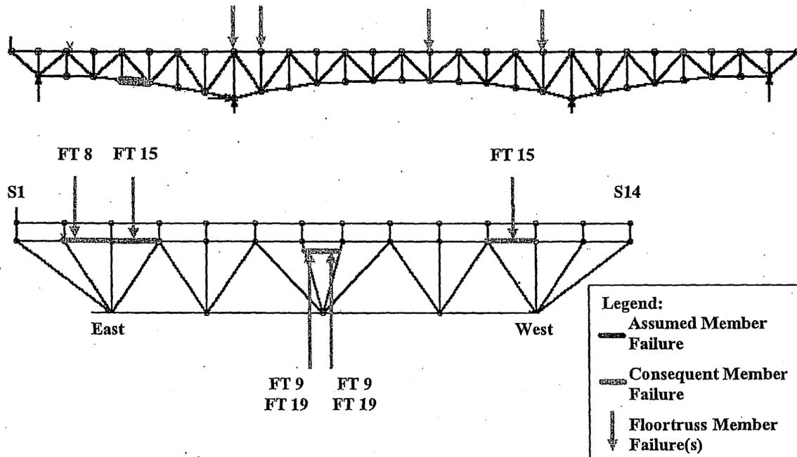
**Figure 6-65: Load Case 4 – Failure of East Truss Lower Chord L4-L5
