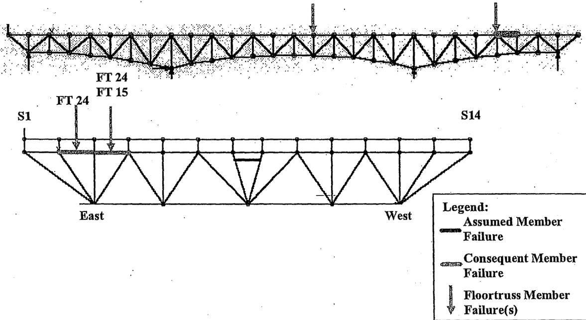
Figure 6-29: Load Case 2 – Failure of East Truss Upper Chord U4'-U3' Consequent Member Failures with a Dynamic Impact Factor of 1.854
