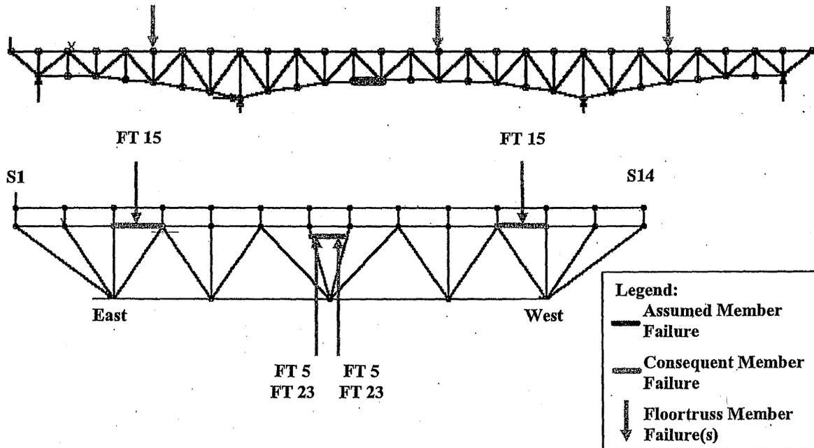
Figure 6-31: Load Case 2 – Failure of East Truss Lower Chord L12-L13
