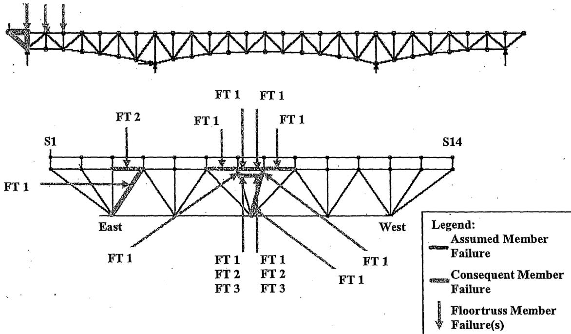
Figure 6-15: Load Case 1 – Failure of East Truss Upper Chord U0-U1 Consequent Member Failures with a Dynamic Impact Factor of 1.854
