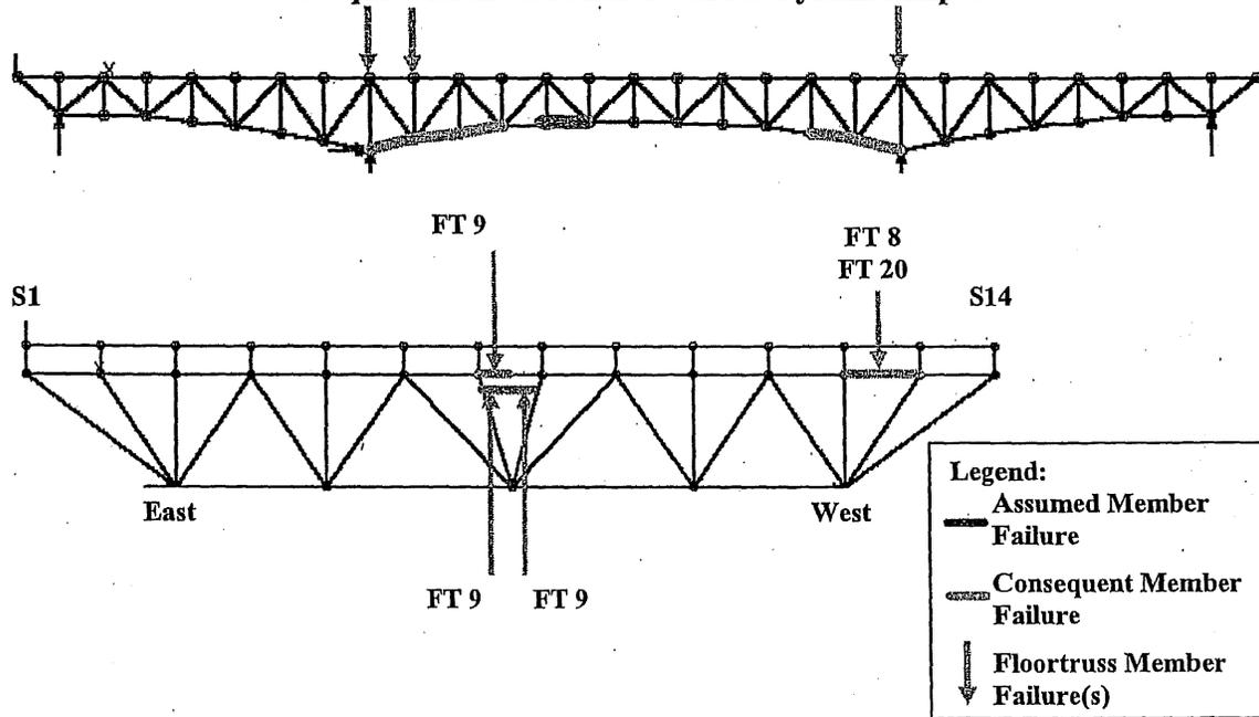
Figure 6-70: Load Case 4 – Failure of East Truss Lower Chord L12-L13
