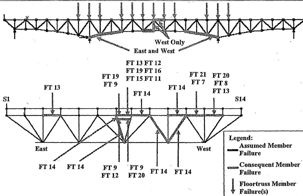
Figure 6-54: Load Case 3 – Failure of East Truss Lower Chord L13-L14
