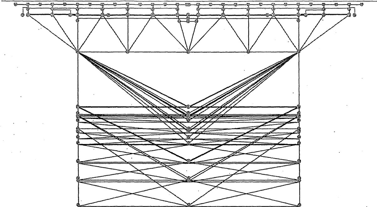
Figure 3-4. Cross Section of Bridge Model Presented by Line Members
