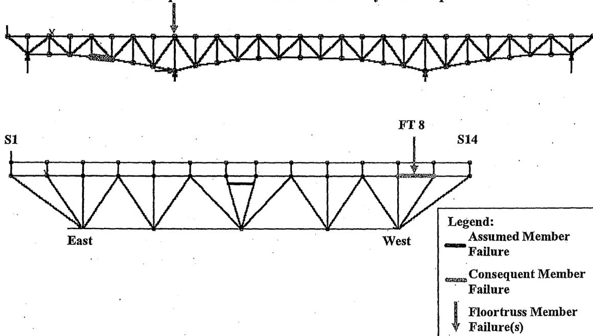
Figure 6-67: Load Case 4 – Failure of East Truss Lower Chord L4-L5
