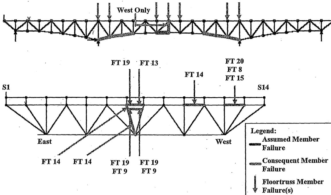
Figure 6-37: Load Case 2 – Failure of East Truss Lower Chord L13-L14
