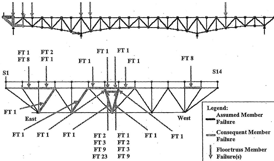
Figure 6-60: Load Case 4 – Failure of East Truss Upper Chord U0-U1
