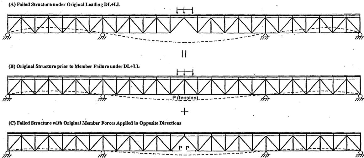
**Figure 6-2: Superposition Process for Truss Member Forces Caused by a Member Failure**
