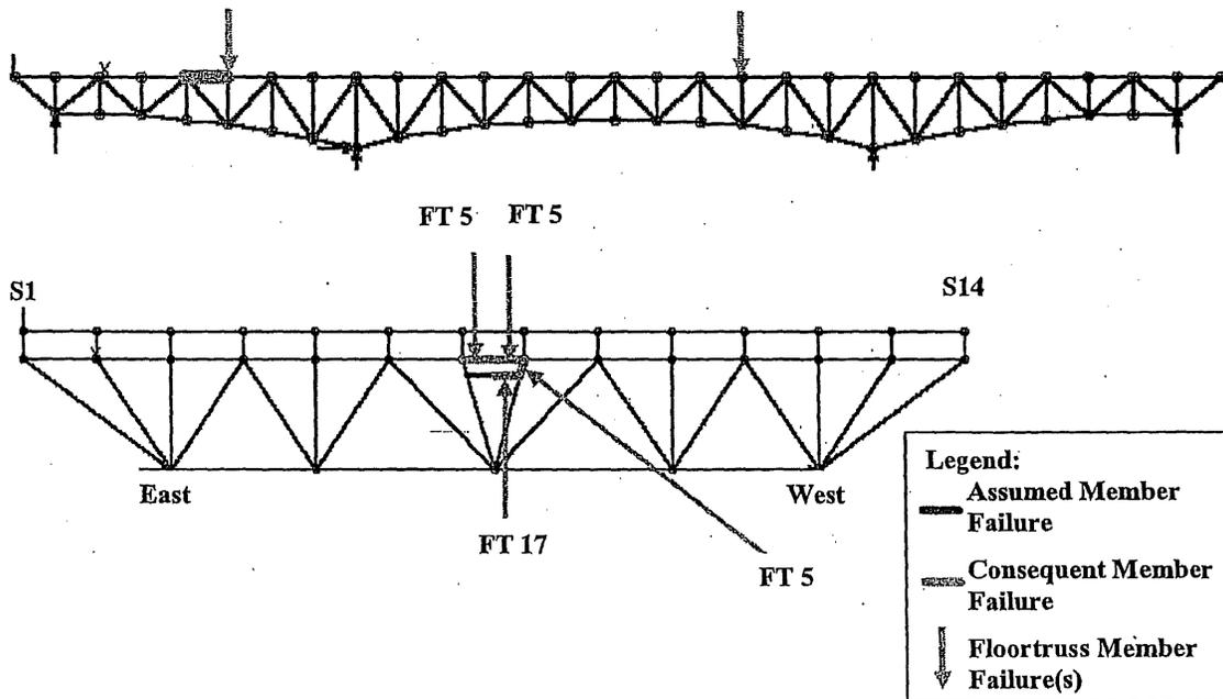
Figure 6-62: Load Case 4 – Failure of East Truss Upper Chord U4-U5
