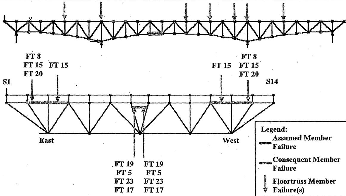
Figure 6-49: Load Case 3 – Failure of East Truss Lower Chord L12-L13
