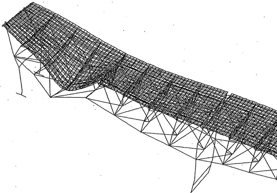
**Figure 6-6: Deformed Shape after Failure of East Truss Diagonal L3-U4**
