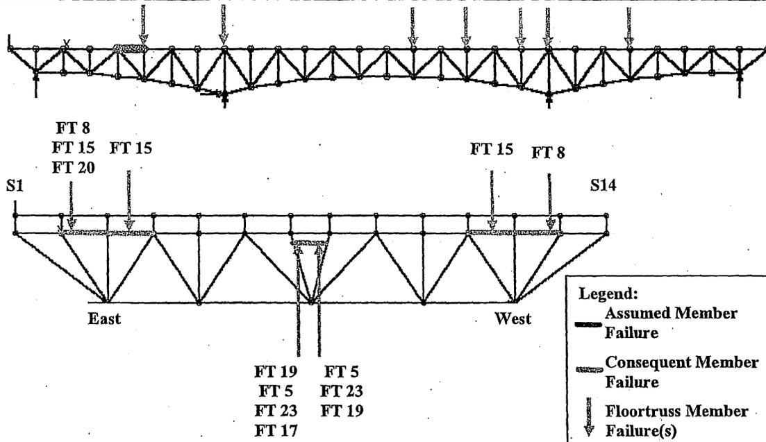
Figure 6-61: Load Case 4 – Failure of East Truss Upper Chord U4-U5
