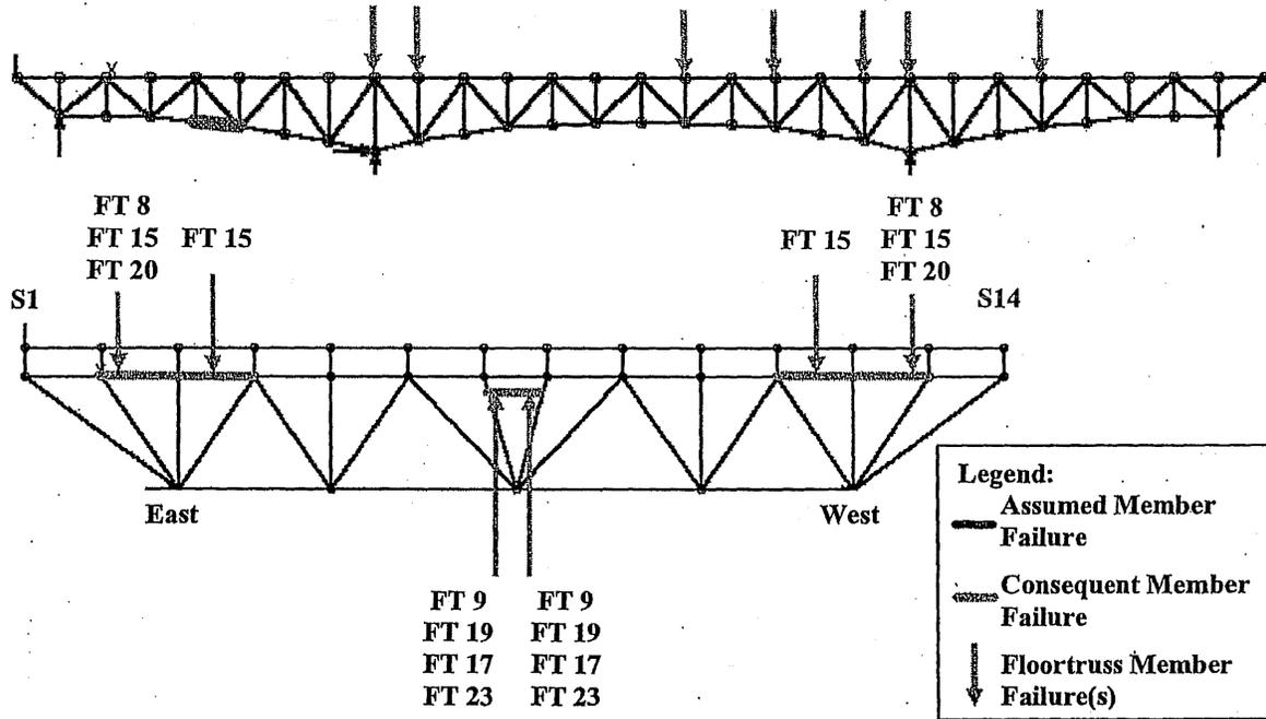
**Figure 6-48: Load Case 3 – Failure of East Truss Lower Chord L4-L5
