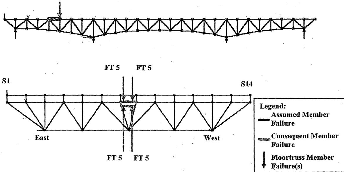
Figure 6-16: Load Case 1 – Failure of East Truss Upper Chord U4-U5
