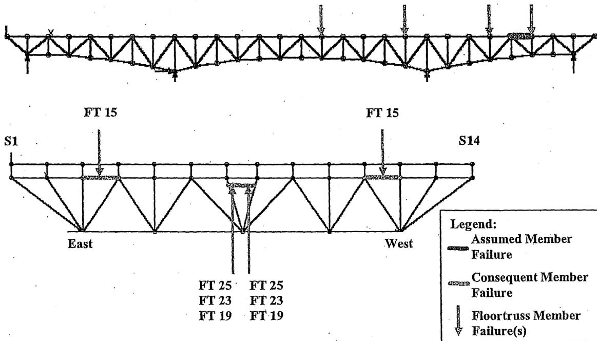
**Figure 6-64: Load Case 4 – Failure of East Truss Upper Chord U4'-U3'
