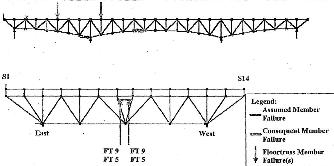
Figure 6-18: Load Case 1 – Failure of East Truss Lower Chord L12-L13
