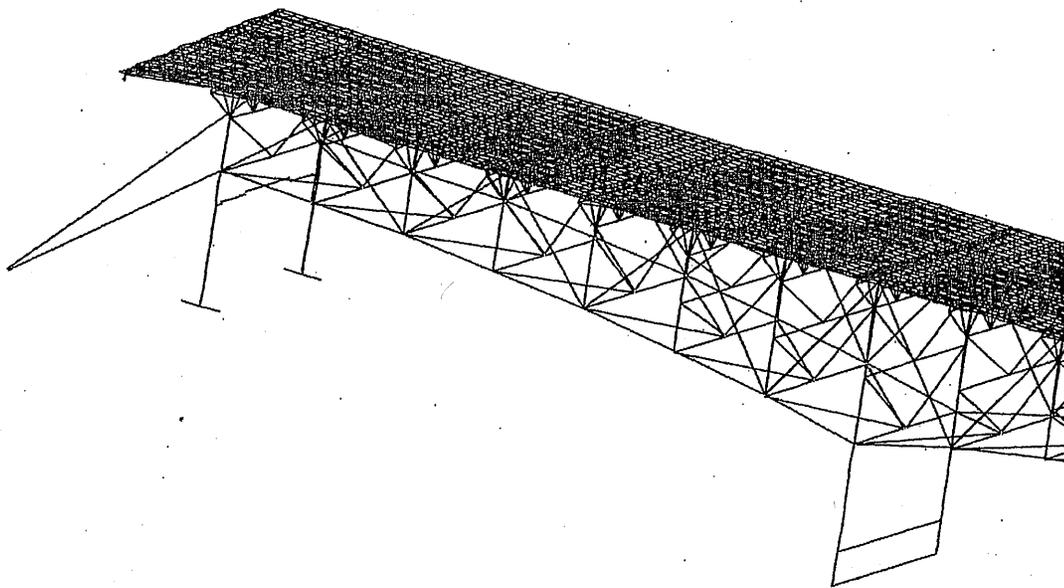
**Figure 6-8: Deformed Shape after Failure of East Truss Upper Chord U0-U1**
