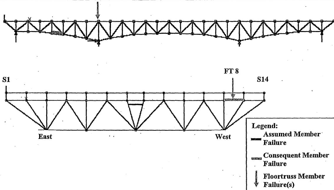
Figure 6-66: Load Case 4 – Failure of East Truss Lower Chord L4-L5
