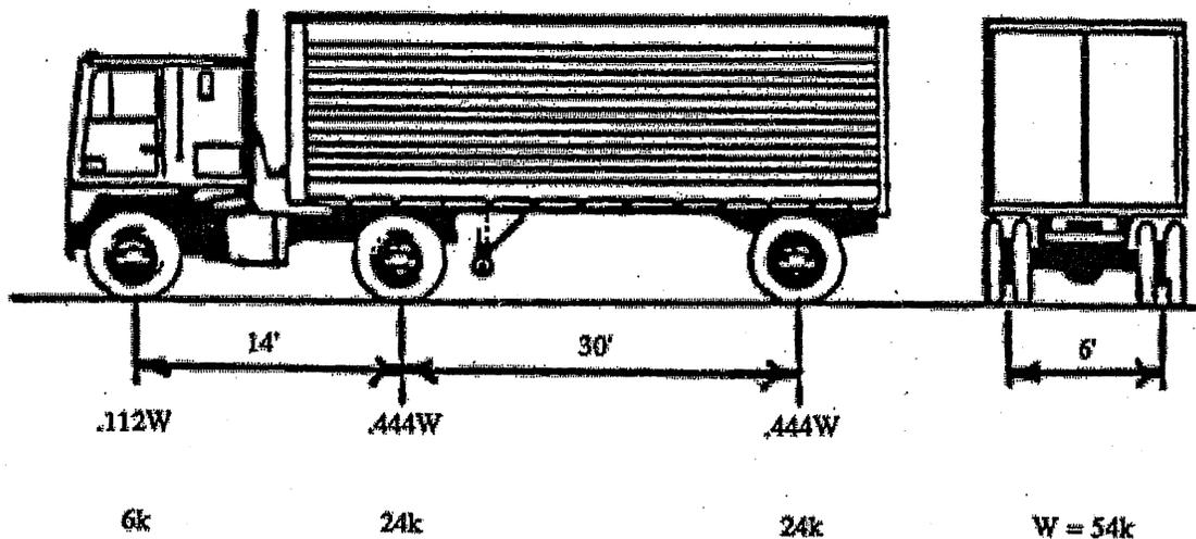
Note: A Variable spacing of 14 to 30 feet can be used instead of the 30-foot main axle spacing, but this may significantly reduce the calculated remaining life.
