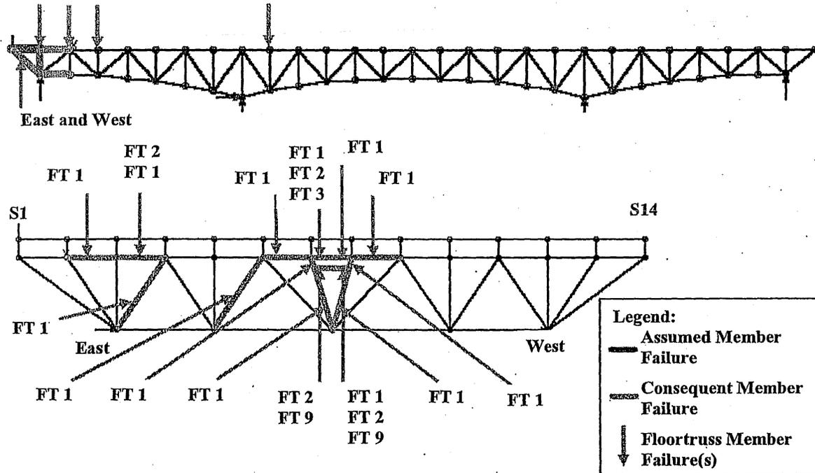
Figure 6-43: Load Case 3 – Failure of East Truss Upper Chord U0-U1 – Consequent Member Failures with a Dynamic Impact Factor of 1.854
