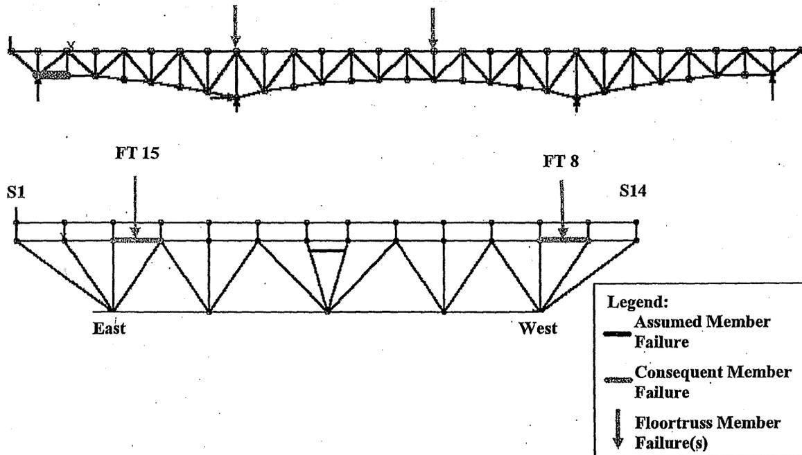
Figure 6-57: Load Case 4 – Failure of East Truss Lower Chord L1-L2
