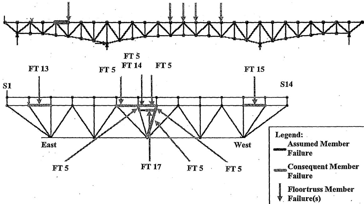
Figure 6-63: Load Case 4 – Failure of East Truss Upper Chord U4-U5
