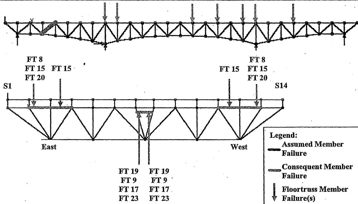
**Figure 6-38: Load Case 3 – Failure of East Truss Diagonal L3-U4
