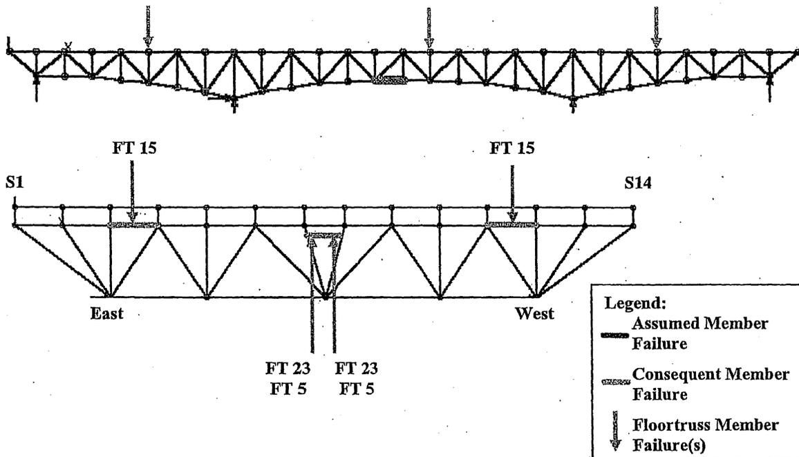
**Figure 6-34: Load Case 2 – Failure of East Truss Lower Chord L13-L14
