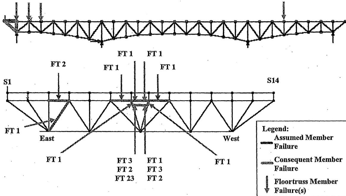
Figure 6-59: Load Case 4 – Failure of East Truss Upper Chord U0-U1
