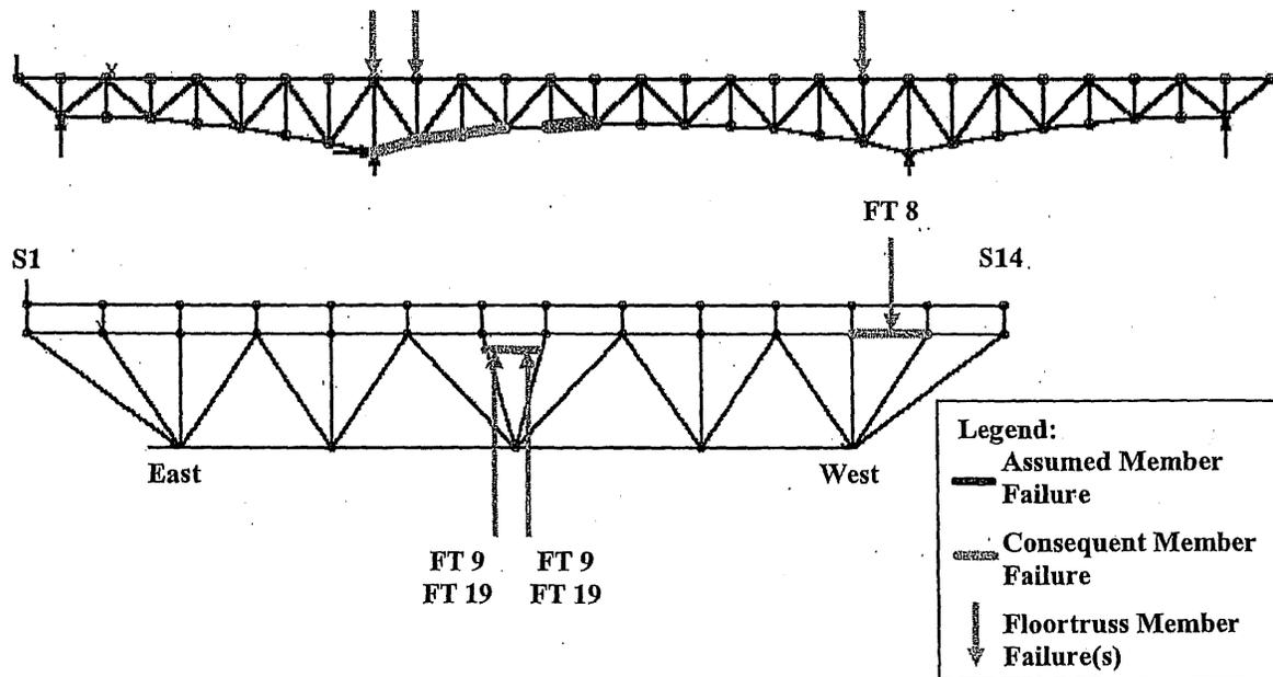
Figure 6-33: Load Case 2 – Failure of East Truss Lower Chord L12-L13
