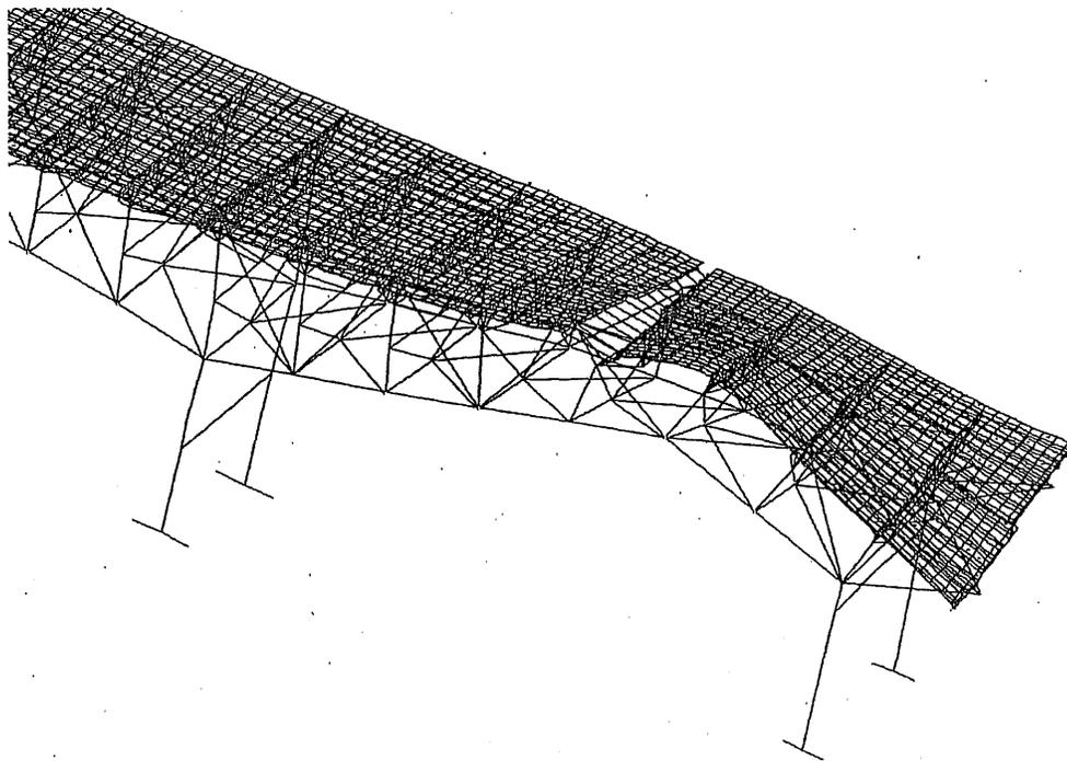
**Figure 6-10: Deformed Shape after Failure of East Truss Upper Chord U4'-U3'**
