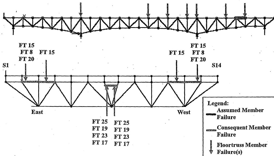
Figure 6-47: Load Case 3 – Failure of East Truss Upper Chord U4'-U3'
