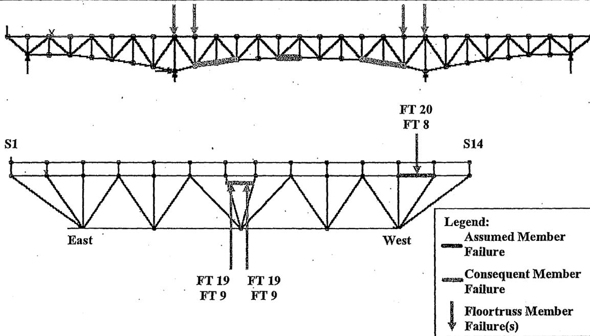
Figure 6-35: Load Case 2 – Failure of East Truss Lower Chord L13-L14
