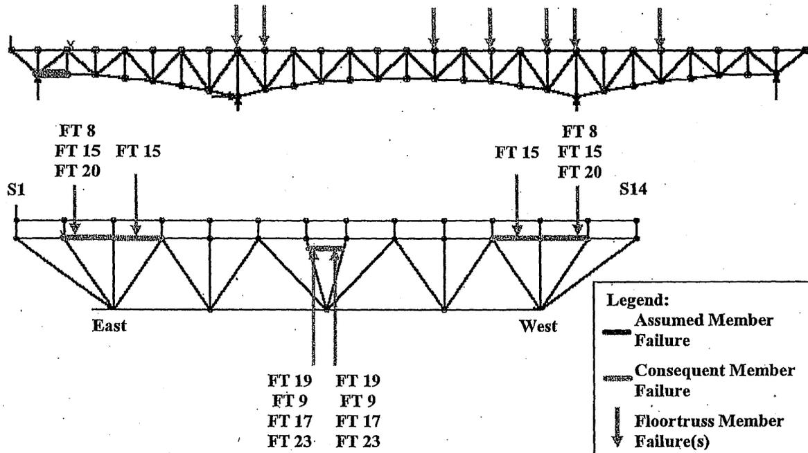
Figure 6-39: Load Case 3 – Failure of East Truss Lower Chord L1-L2
