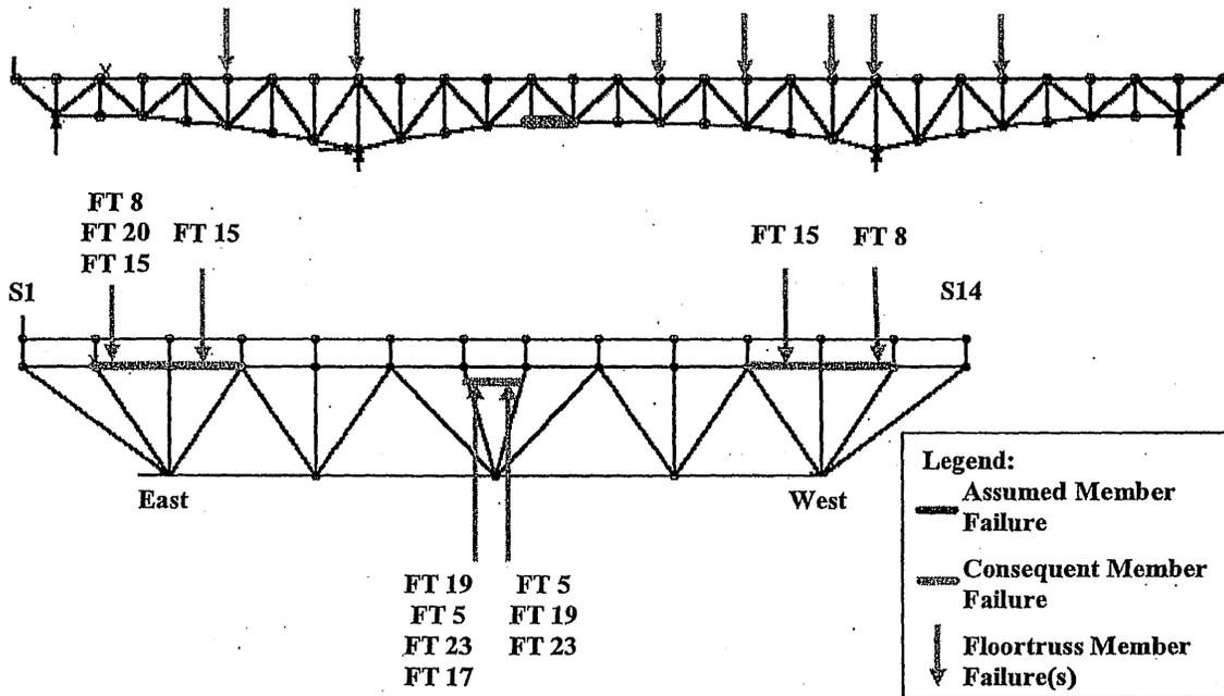
**Figure 6-68: Load Case 4 – Failure of East Truss Lower Chord L12-L13
