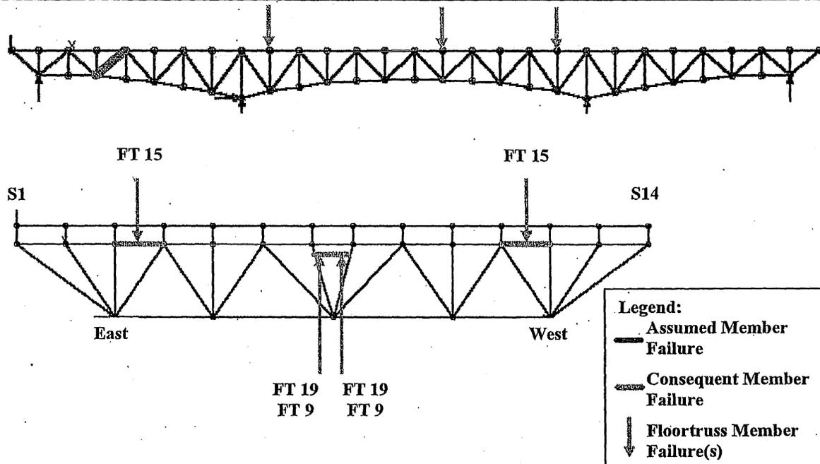
**Figure 6-55: Load Case 4 – Failure of East Truss Diagonal L3-U4
