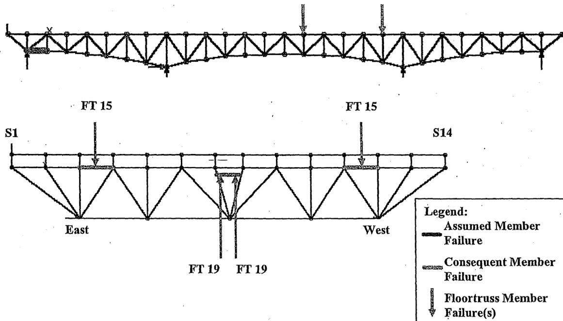
**Figure 6-56: Load Case 4 – Failure of East Truss Lower Chord L1-L2**
