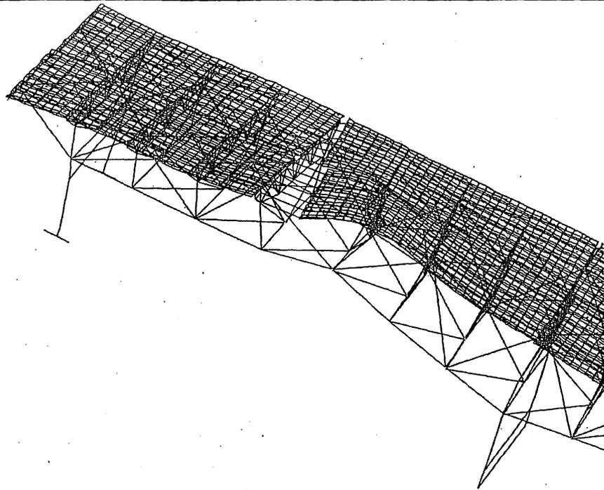
**Figure 6-9: Deformed Shape after Failure of East Truss Upper Chord U4-U5**
