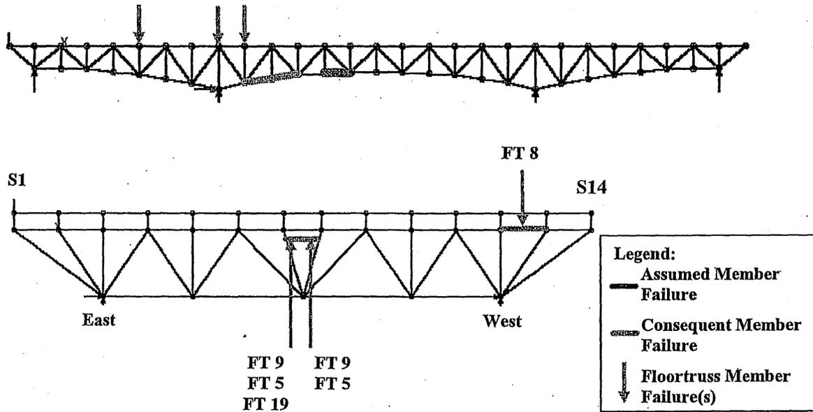
Figure 6-19: Load Case 1 – Failure of East Truss Lower Chord L12-L13
