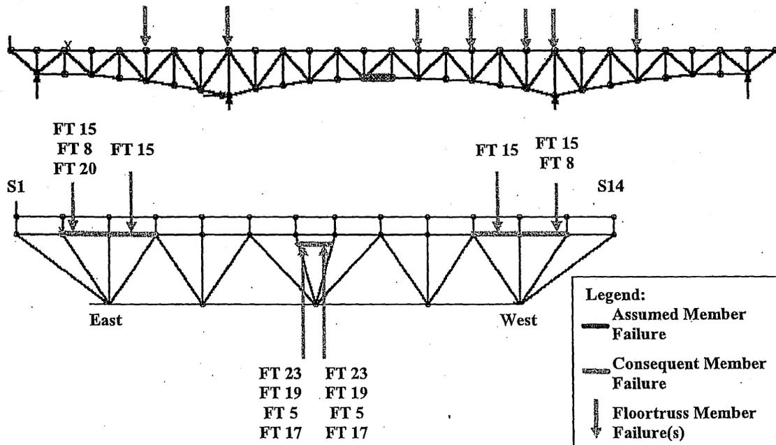
Figure 6-71: Load Case 4 – Failure of East Truss Lower Chord L13-L14
