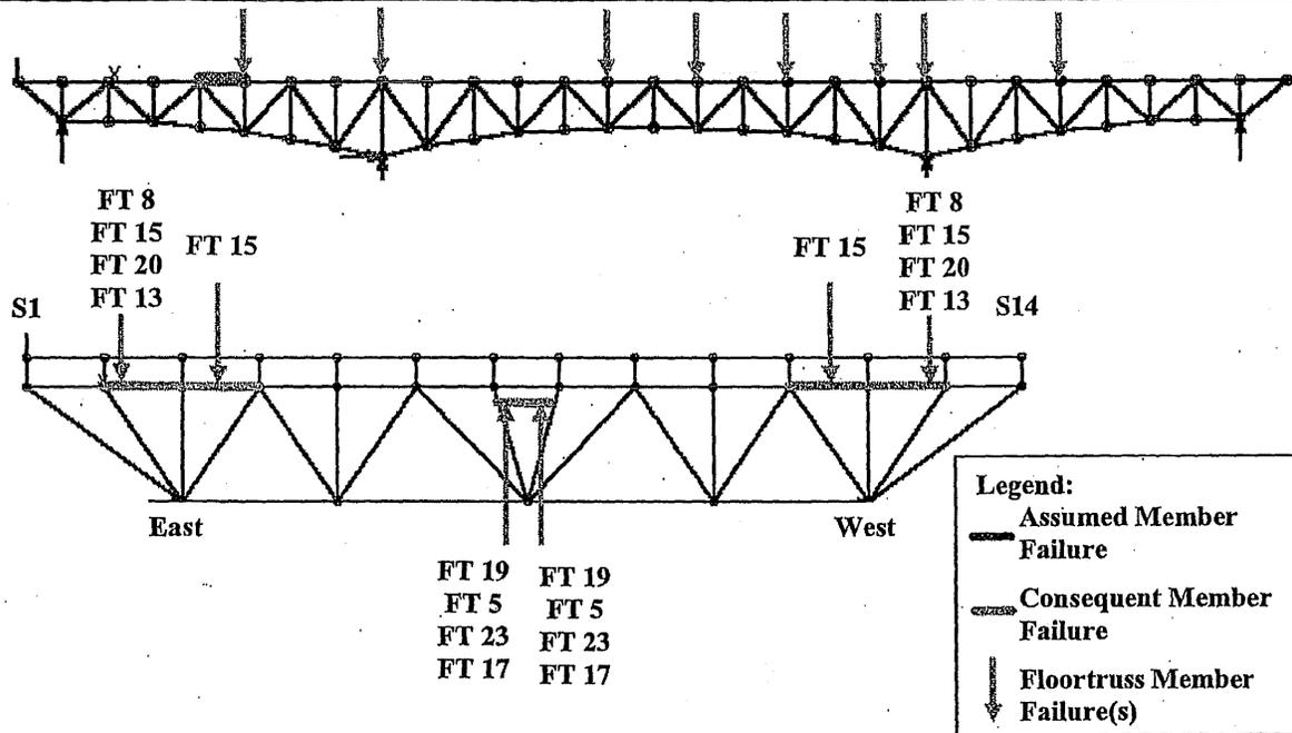
Figure 6-44: Load Case 3 – Failure of East Truss Upper Chord U4-U5
