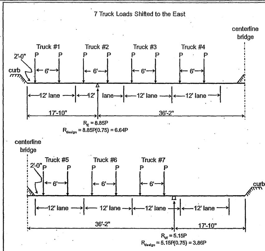
Figure 4-1: Governing Live Load for Strength Design
