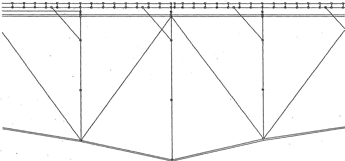
Figure 3-5. Elevation of a Portion of Bridge Model above a Pier Presented by Line Members
