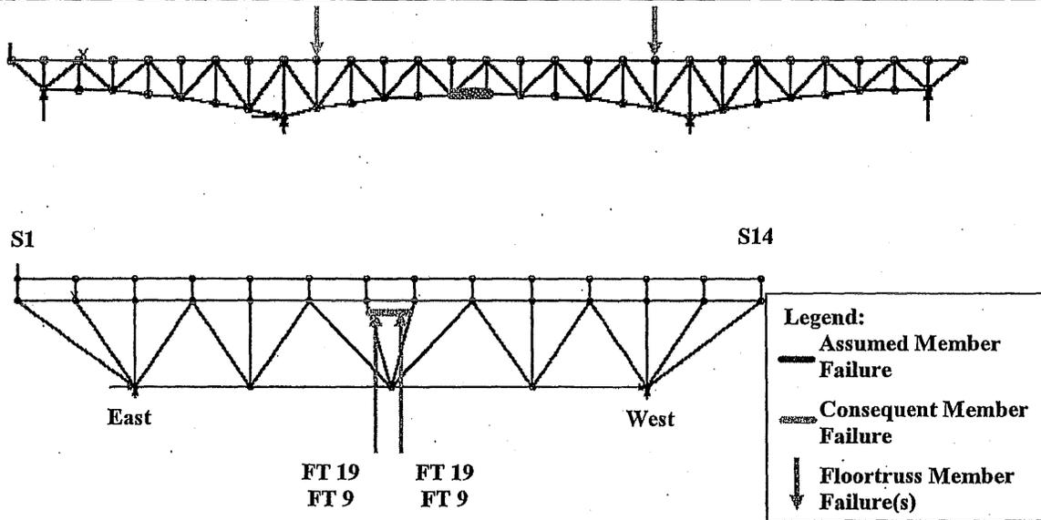
Figure 6-20: Load Case 1 – Failure of East Truss Lower Chord L13-L14
