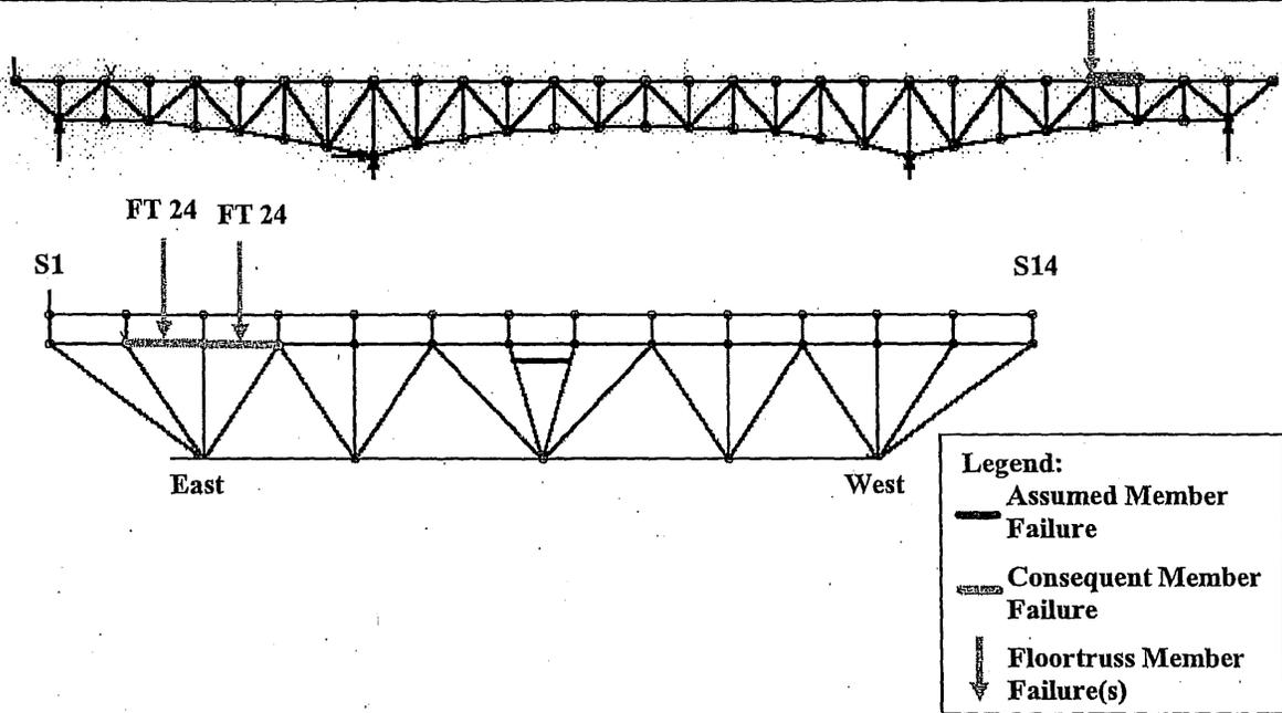
Figure 6-28: Load Case 2 – Failure of East Truss Upper Chord U4'-U3' Consequent Member Failures without Dynamic Impact
