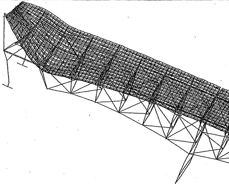
**Figure 6-7: Deformed Shape after Failure of East Truss Lower Chord L1-L2**
