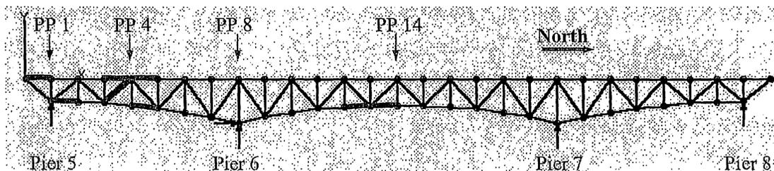
**Figure 6-1: Eight Most Critical Truss Members**
