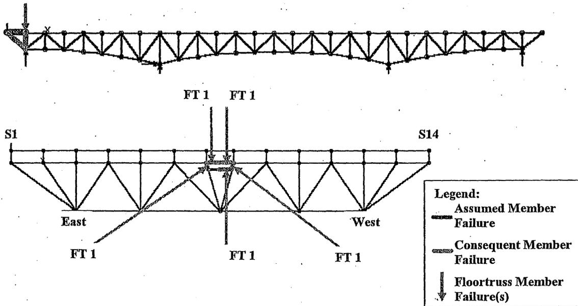
Figure 6-14: Load Case 1 – Failure of East Truss Upper Chord U0-U1
