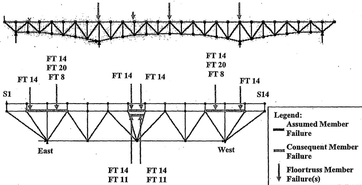
Figure 6-5: Floor Truss Member “Failures” of Intact Structure under Dead Load Only
