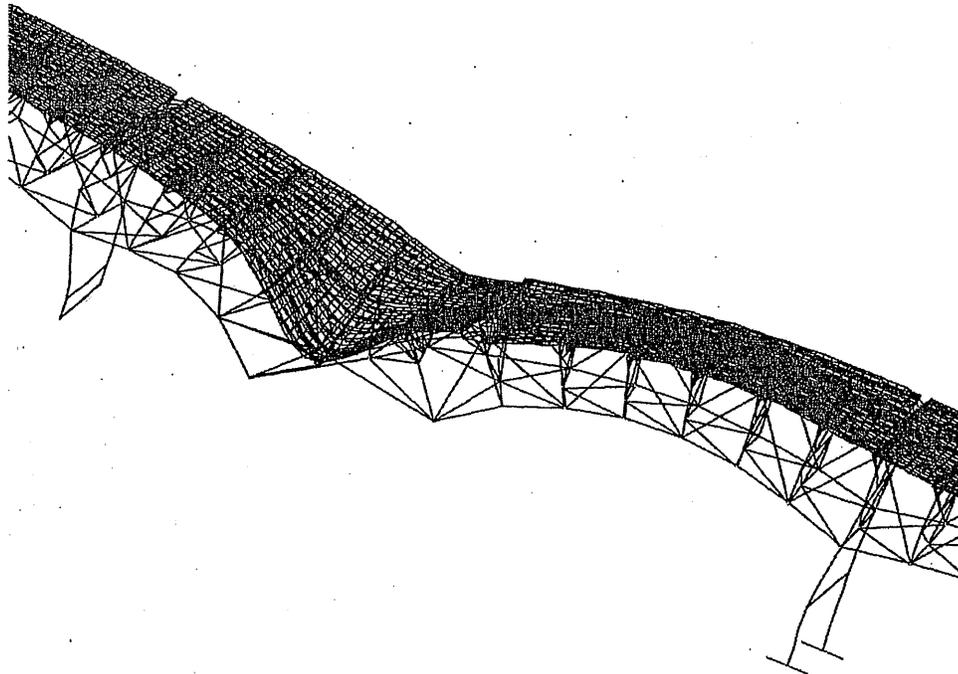
**Figure 6-12: Deformed Shape after Failure of East Truss Lower Chord L12-L13**
