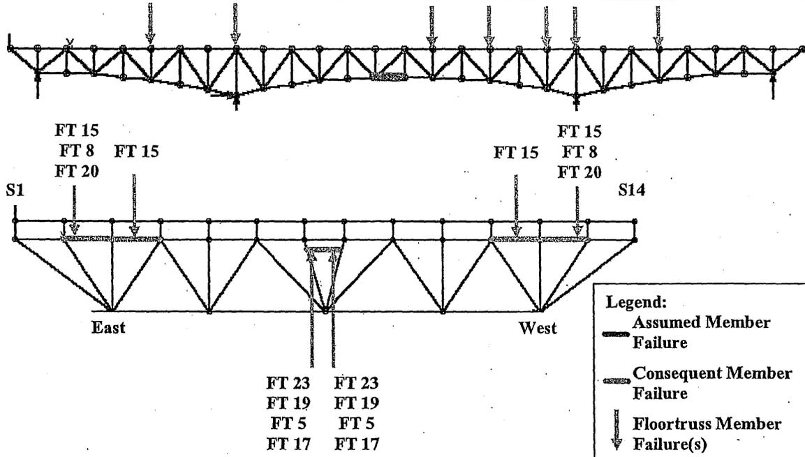
Figure 6-52: Load Case 3 – Failure of East Truss Lower Chord L13-L14
