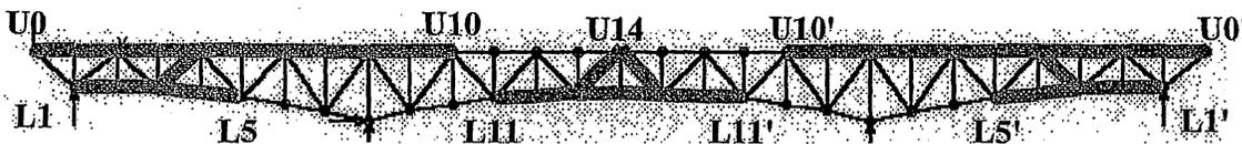
Figure 5-1: Main Truss Members with Fatigue Susceptible Details
