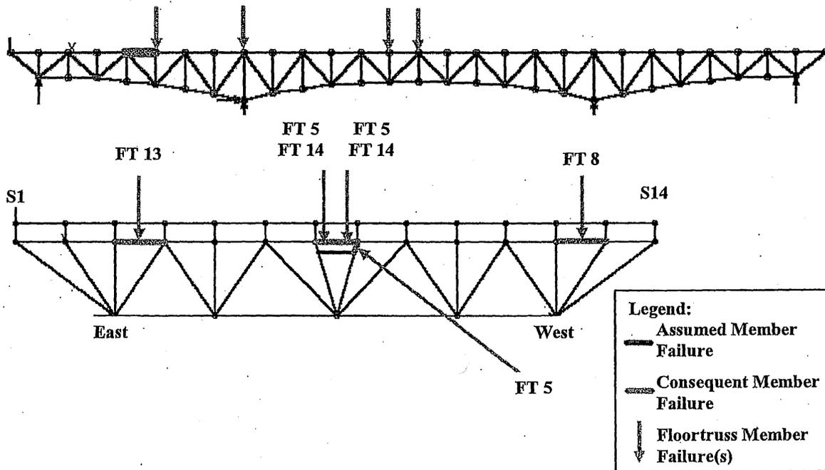
Figure 6-45: Load Case 3 – Failure of East Truss Upper Chord U4-U5
