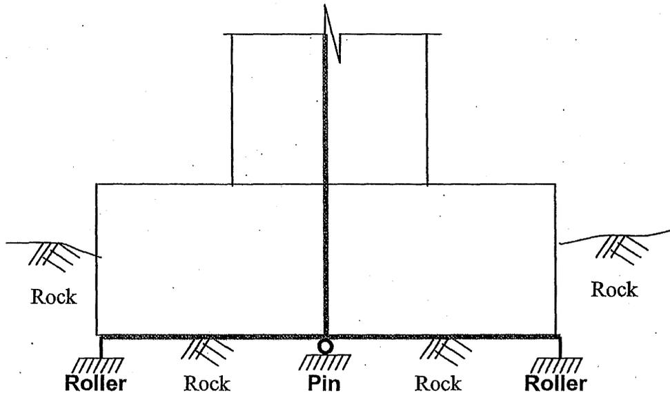
Figure 3-22: Modeling of Base Support of Piers 5, 7, and 8
