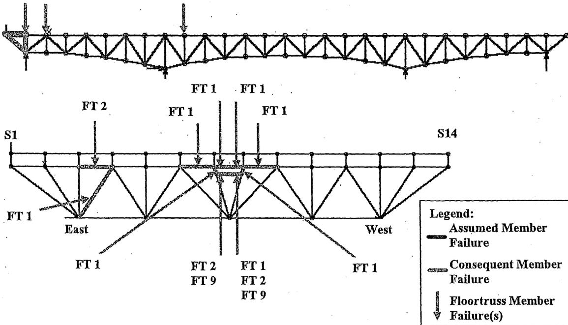
Figure 6-42: Load Case 3 – Failure of East Truss Upper Chord U0-U1 –
