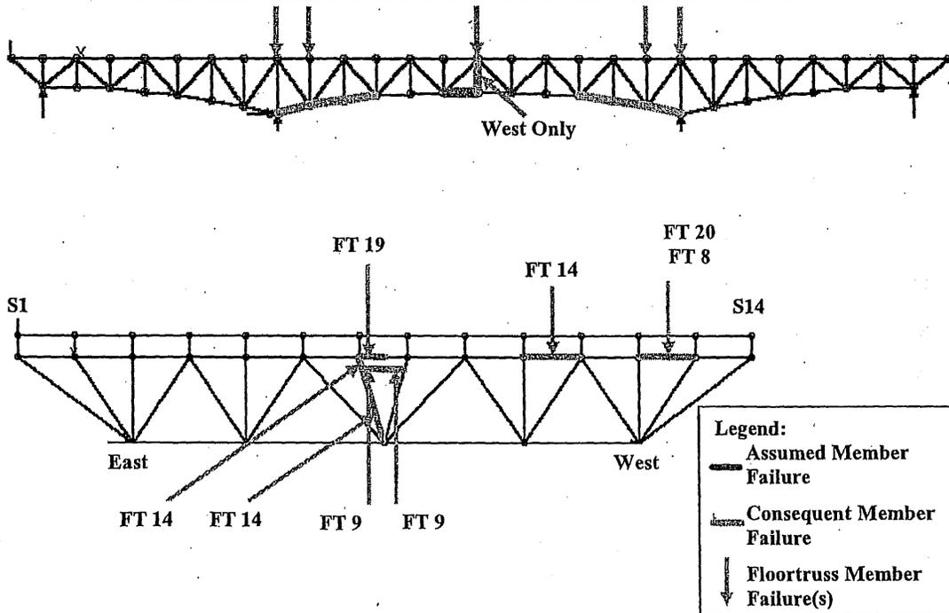
Figure 6-53: Load Case 3 – Failure of East Truss Lower Chord L13-L14
