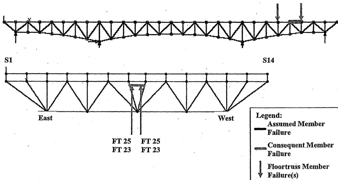
**Figure 6-27: Load Case 2 – Failure of East Truss Upper Chord U4'-U3'
