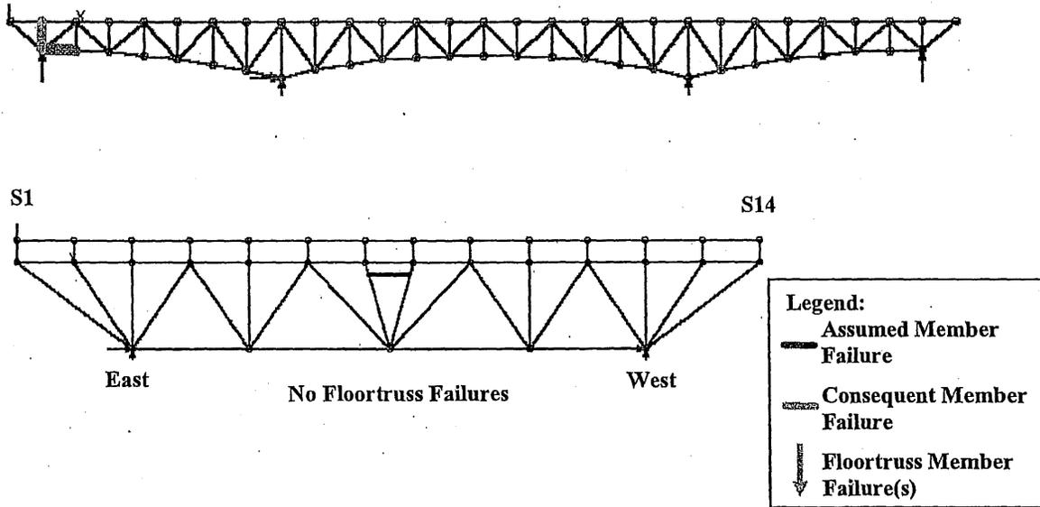
**Figure 6-40: Load Case 3 – Failure of East Truss Lower Chord L1-L2
