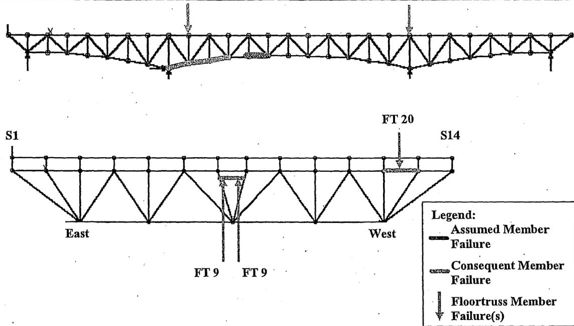
Figure 6-69: Load Case 4 – Failure of East Truss Lower Chord L12-L13
