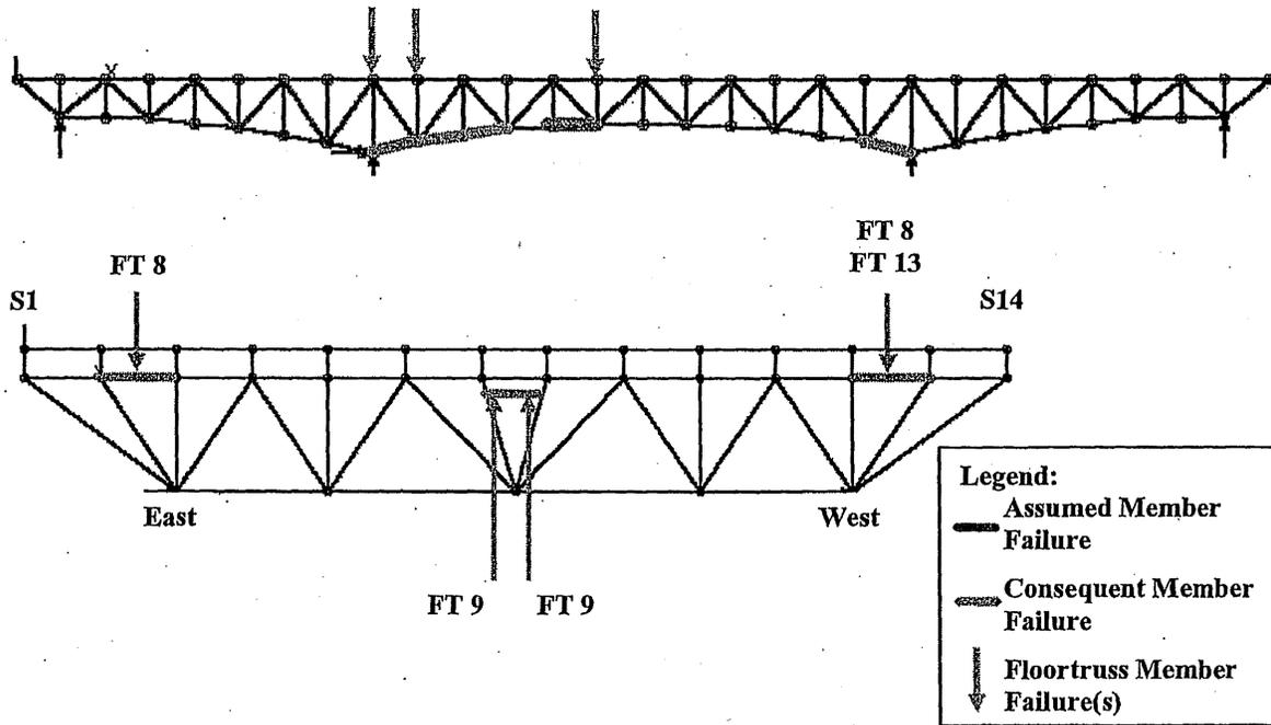
Figure 6-50: Load Case 3 – Failure of East Truss Lower Chord L12-L13
