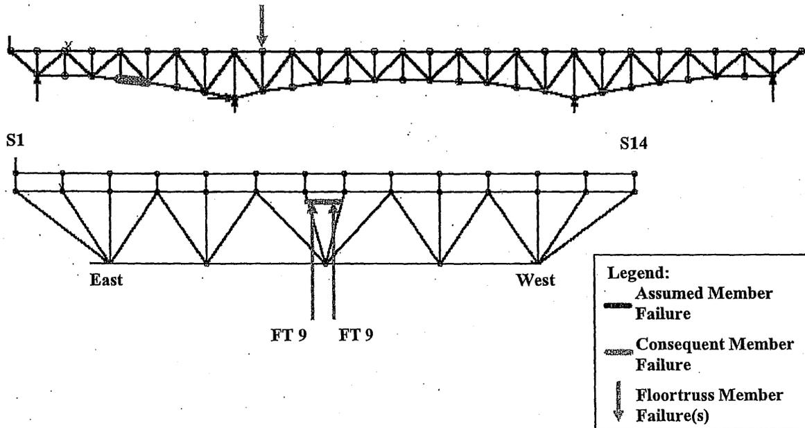
**Figure 6-30: Load Case 2 – Failure of East Truss Lower Chord L4-L5
