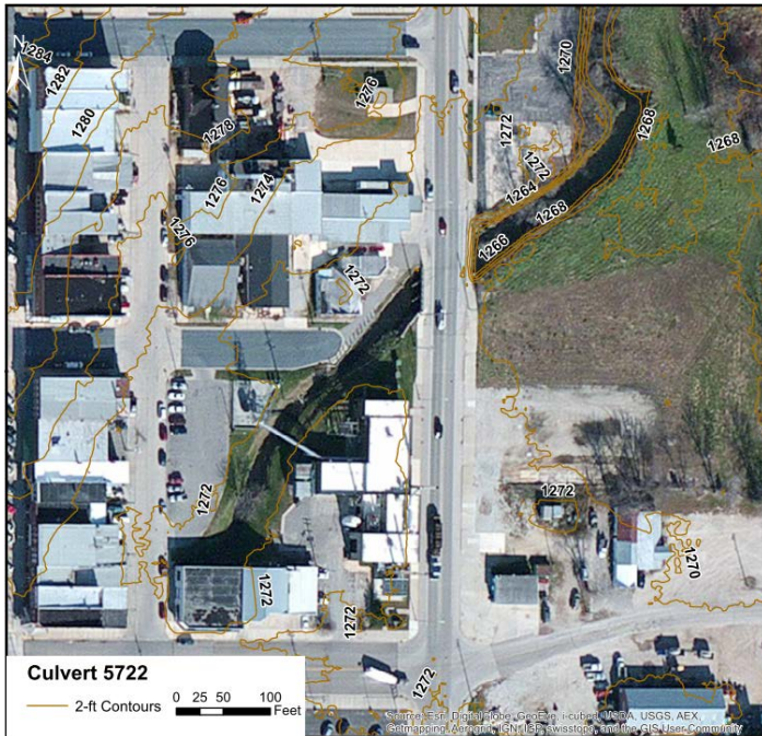
Figure 31: Plan View of Culvert 5722 Showing Elevation Contours
