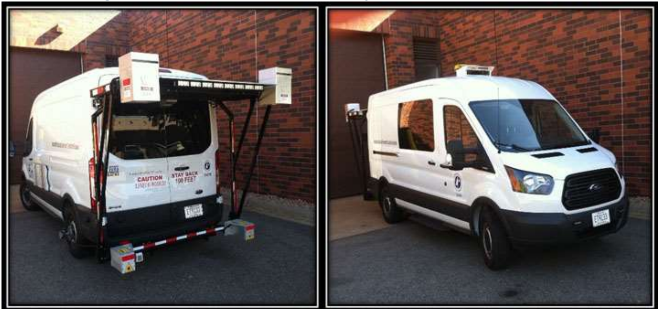
Figure 2. Network-Level Pavement Surface Data Collection Vehicle
