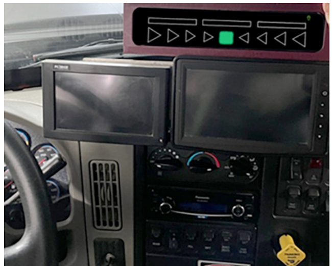
A dashboard guidance system displays visual indicators and auditory warnings to significantly enhance safety in whiteout conditions.
