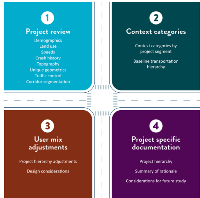
Figure 15. Transportation hierarchy framework process summary from MnDOT’s Complete Streets Project Transportation Hierarchy Tool
