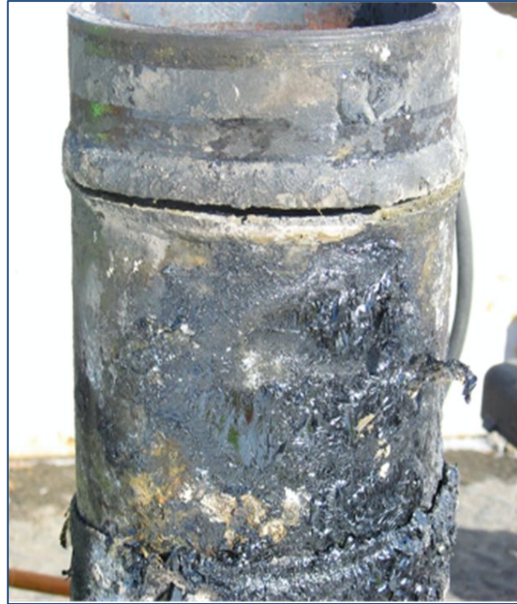
Left: Morris Campus - ruptured natural gas pipe
