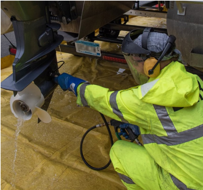
Level 2 Inspector Matt Dwelly conducts an engine decontamination on a pontoon boat's outboard motor in 2022.
