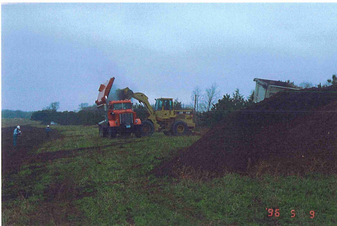
Figure A9.5. Loading MSW compost into the compost spreader. Note the pile of MSW compost in the foreground, and the steam rising from the load being placed into the spreader.
