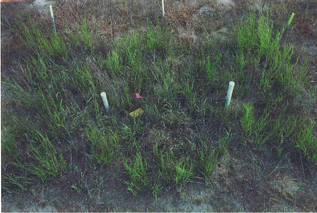
Figure A15.7. MSW (lysimeter plots). The two white PVC pipes are the 6" and 24" suction lysimeters that were installed in 1997.
