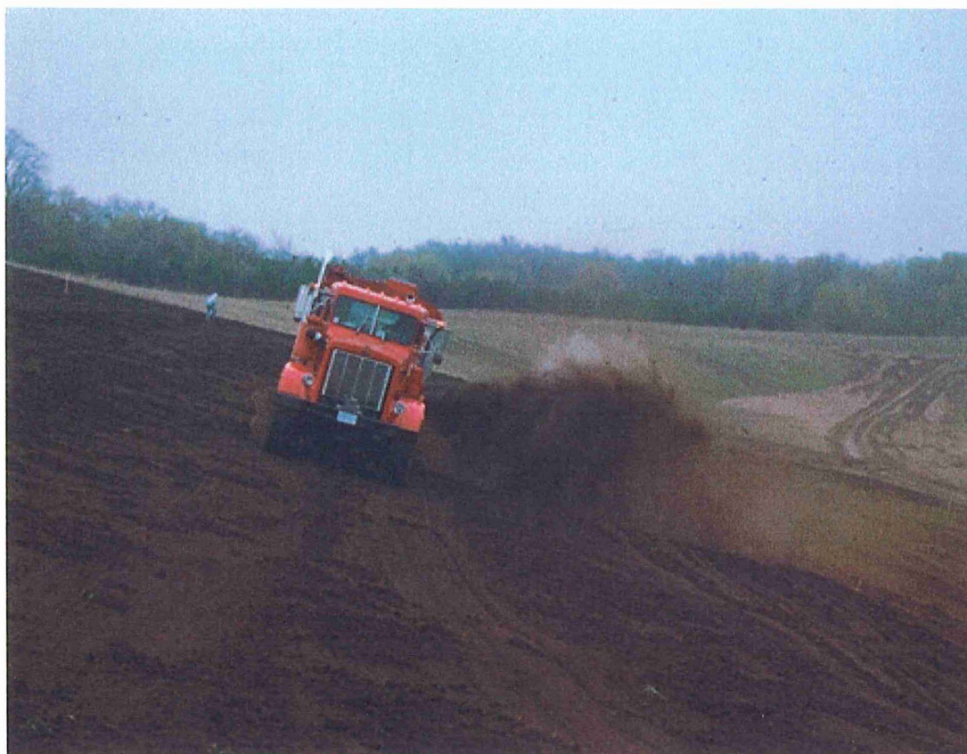
Figure A9.6. Spreading MSW compost on the demonstration plot with a compost spreader, which was also used to spread the NVS on its demonstration plot.
