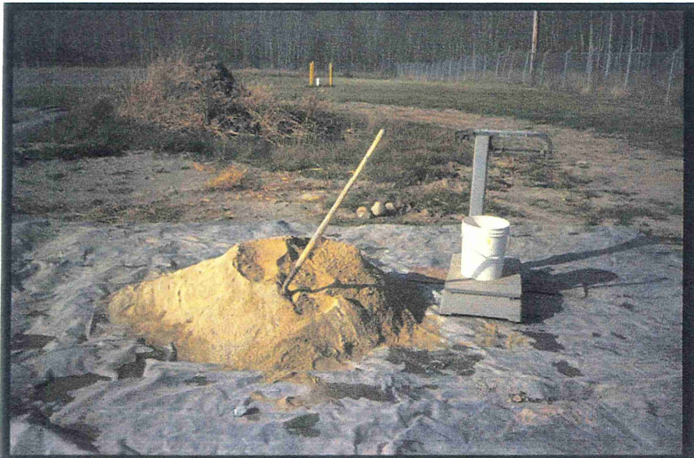
Figure 13. Limestone used for the alkaline mixture experiment. The limestone product was purchased from Agrerate Resources' Larson Mine on Grey Cloud Island and is called a manufactured sand
