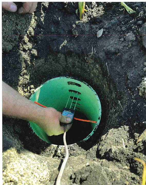
Photo 1. Soil moisture sensor installed in the field.
