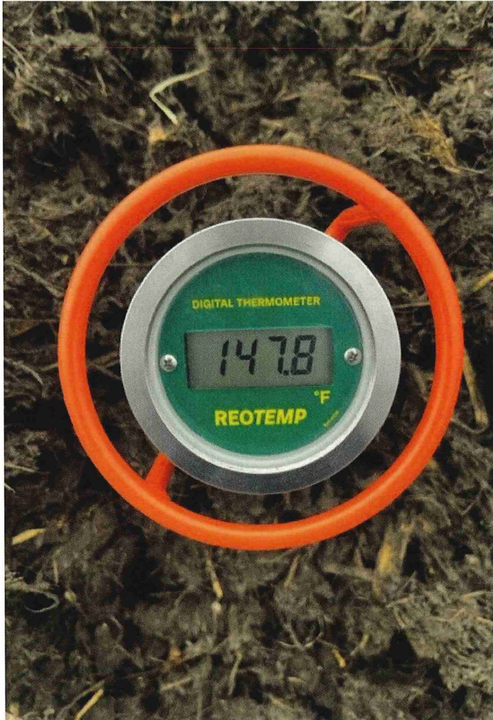
Compost thermometer used for recording compost temperatures.
