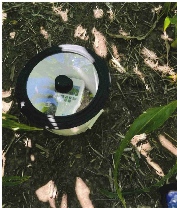
Measuring soil carbon dioxide in corn plot.
