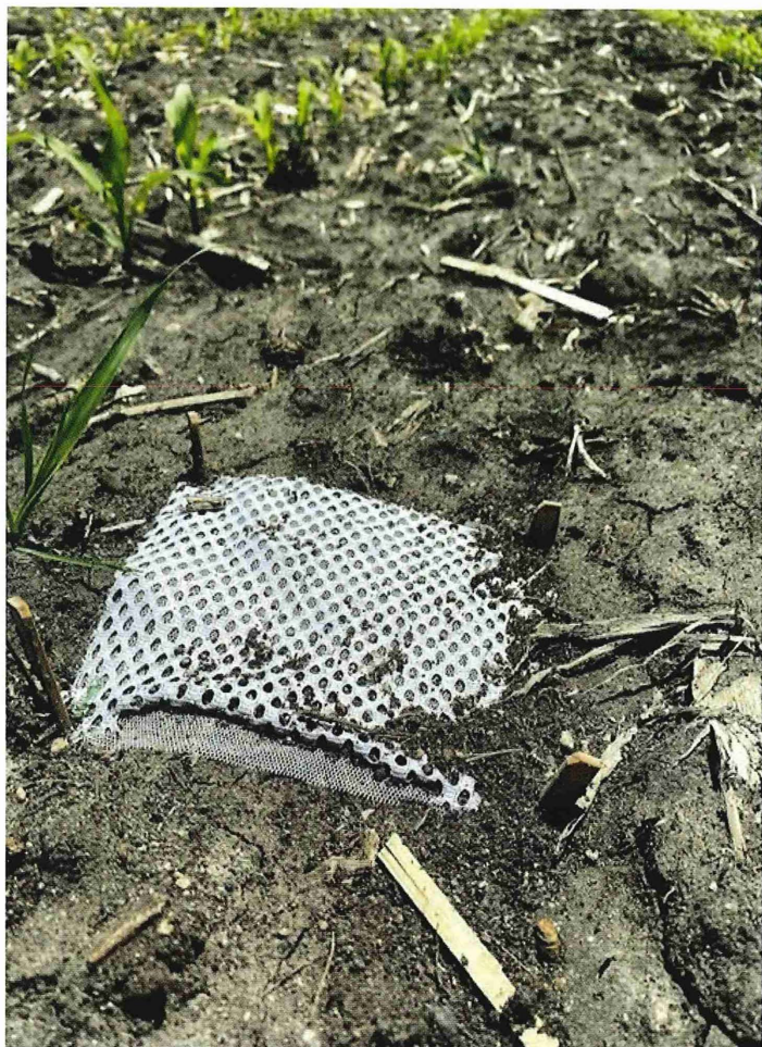
Photo 4. Mat with soil movement collected. Photo taken on collection day of mats.
