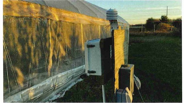
Temperature sensor and data logger outside the high tunnel.
