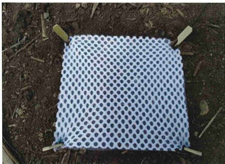
Example of mat used to collect soil movement.
