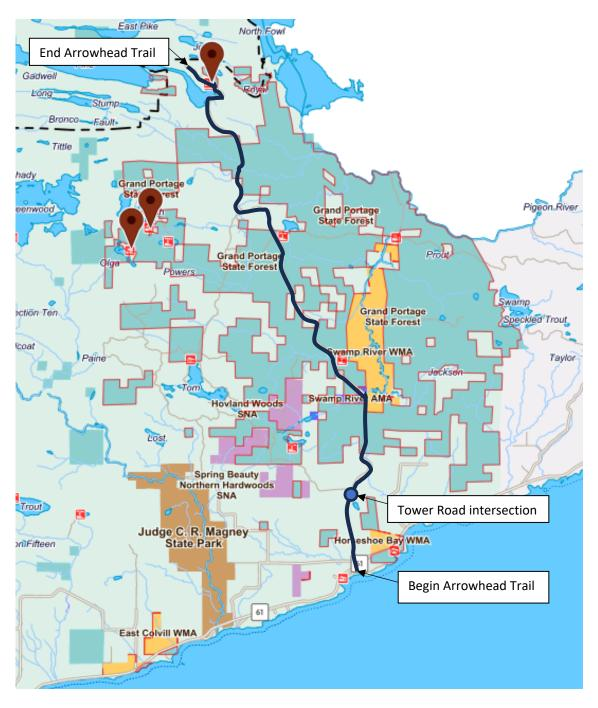
The proposed project will start at the beginning of the Arrowhead Trail (intersection with Trunk Highway 61) and commence 2.5 miles north, ending at the intersection with Tower Road (see map below). The project will upsize an undersized culvert into a bridge that was determined to be a barrier for fish passage and inadequate drainage, replace five corrugated metal culverts that are beyond their useful life with concrete culverts, and resurface the entire 2.5 miles of existing pavement.
