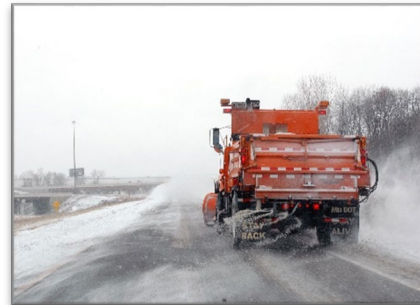
Minnesota Department of Transportation applying road salt. Photo by David R. Gonzalez of MnDOT.
