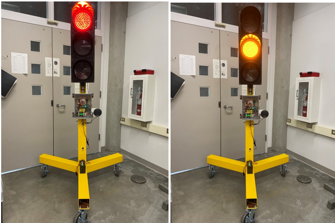
Figure 2.7 Photographs of the two modes on the smart work zone traffic signal.
