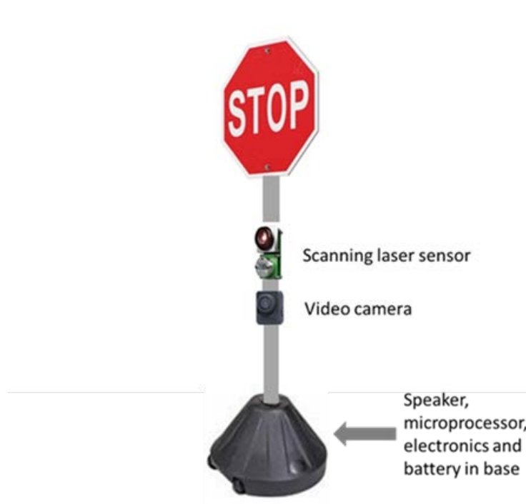
Figure 2.1 Proposed initial work zone traffic control device.
