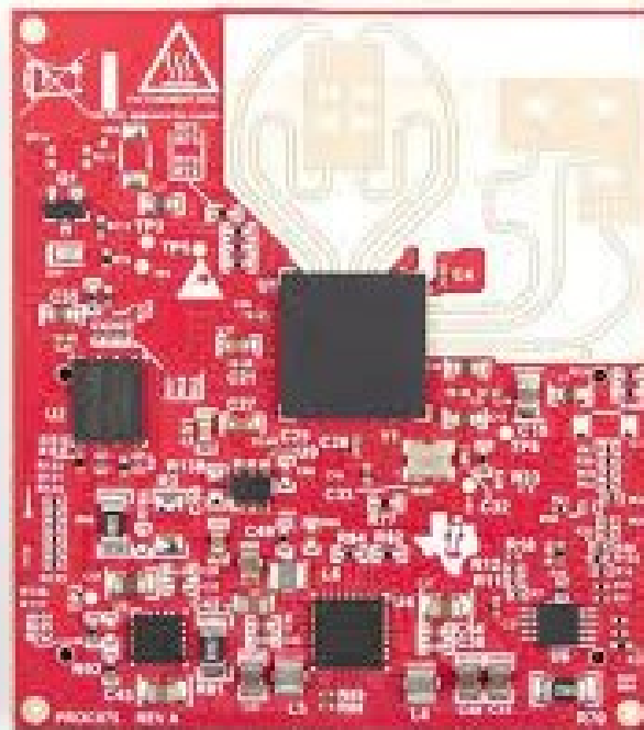
Figure 2.4 Low-cost radar chip and antenna on a printed circuit board.
