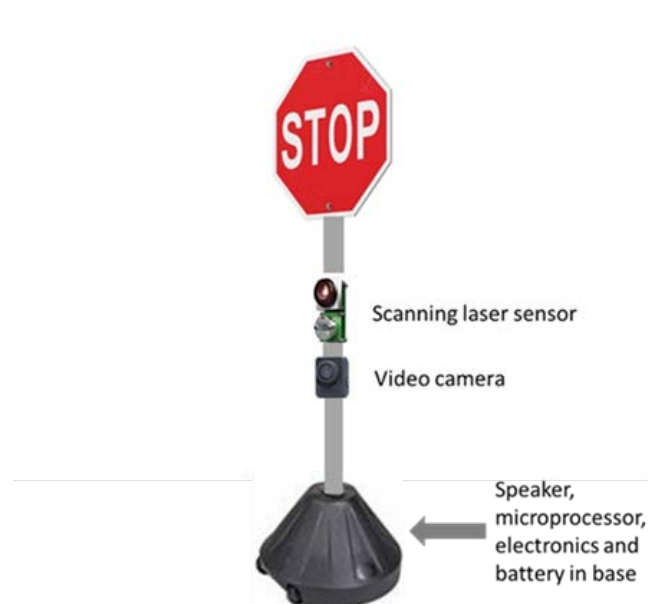
Figure 7.1 Initial STOP/SLOW prototype design proposed by engineering team
