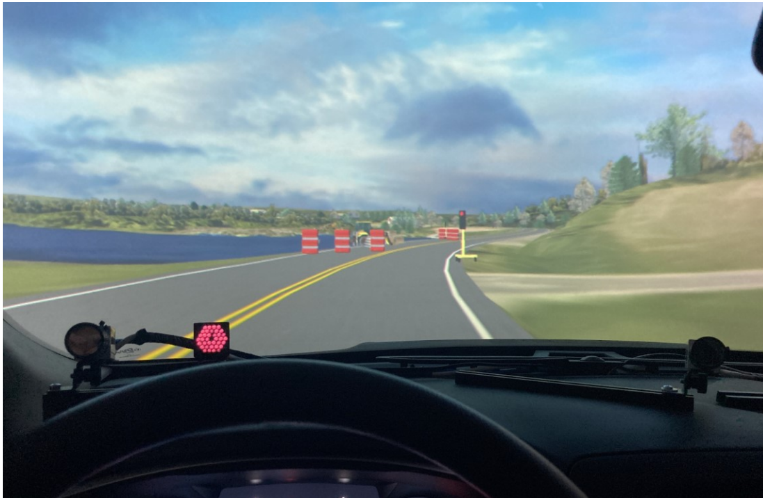
Figure 4.10 Image of driver's perspective of signal displaying red light at work zone
