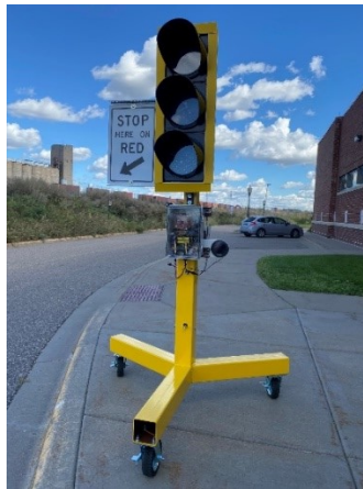
Figure 7.3 Final traffic signal prototype design
