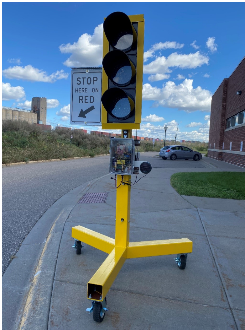
Figure 2.2 Photograph of the implemented smart work zone traffic signal.
