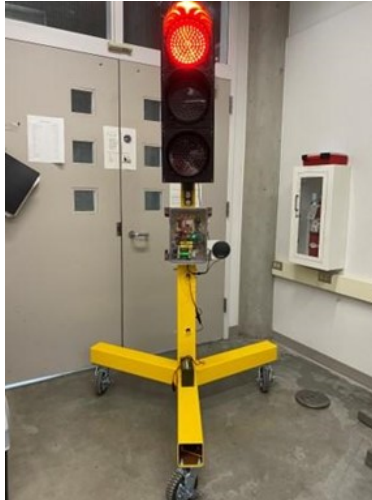
Figure 7.2 Revised traffic signal prototype design
