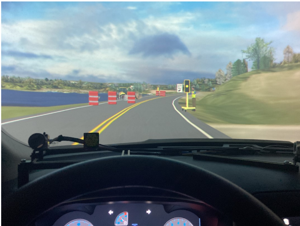
Figure 5.5 Image of experimental traffic signal signaling to proceed at work zone
