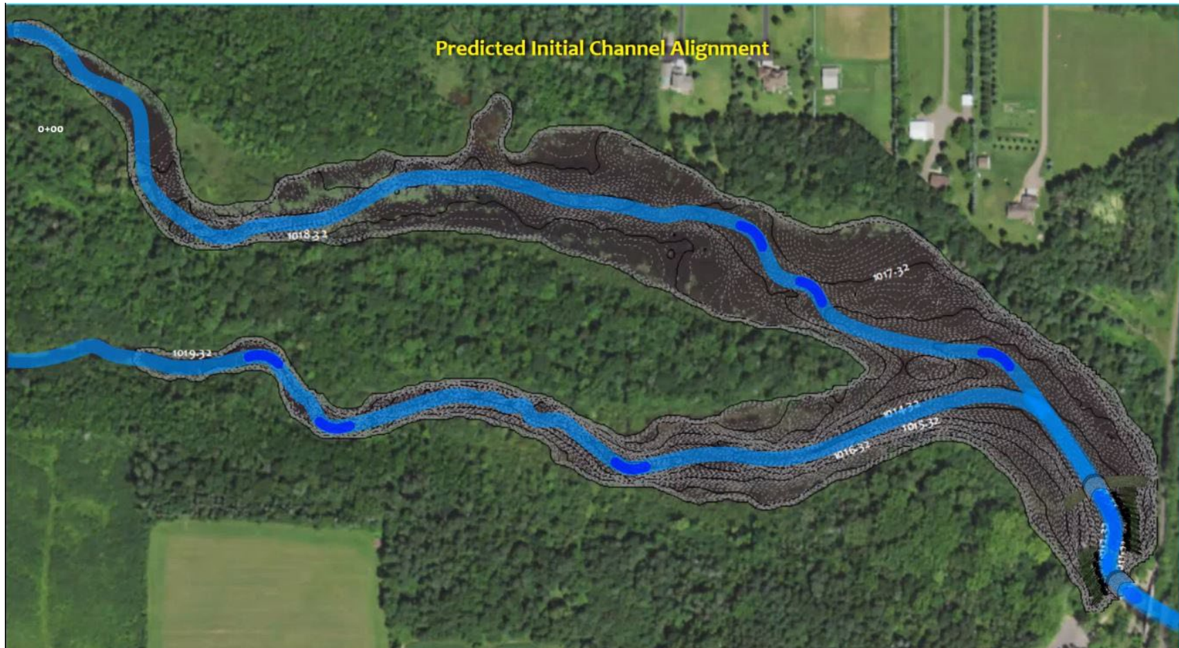
Figure 2-1. Predicted initial channel alignment following proposed project implementation. Dark blue areas indicate areas of pool formation. The two constructed riffles are depicted at the dam location and just upstream.
